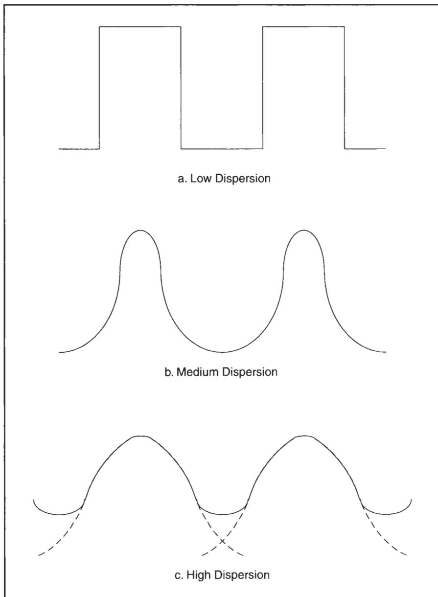
the received pulse the time between  $-3$ -dB points is  $T_d$ . The dispersion is expressed as the difference, or:
