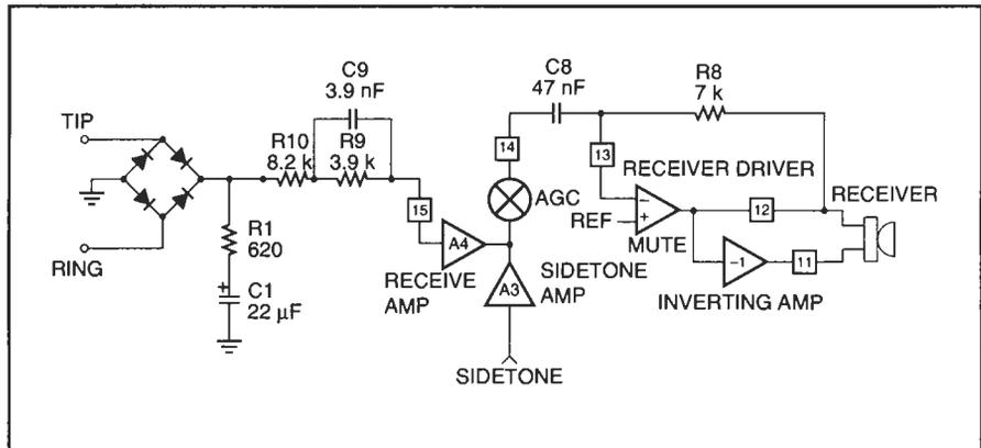
sidetone signal from the sidetone amplifier is mixed with the receive signal to supply sidetone in the telephone handset.
