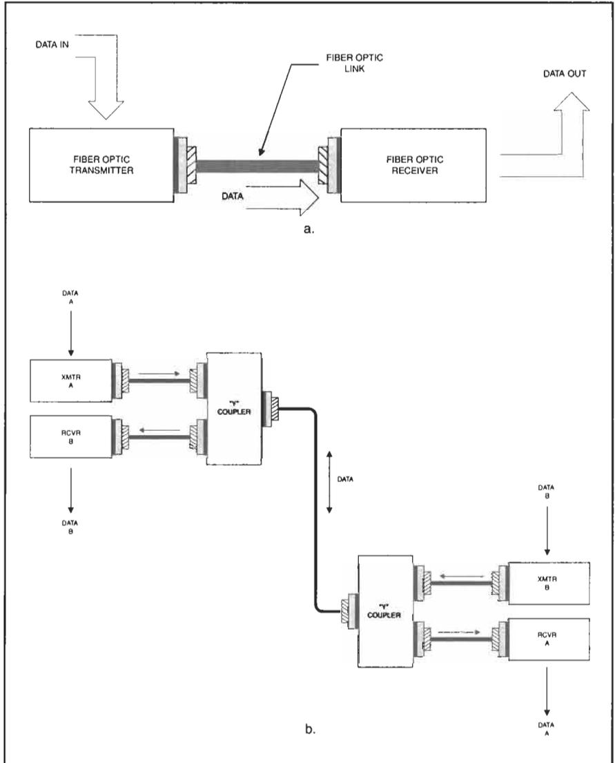
information over the path in only one direction to a receiver set at the other end. The receiver cannot reply or otherwise send data back the other way. The simplex system requires only a single transmitter and a single receiver per channel.
