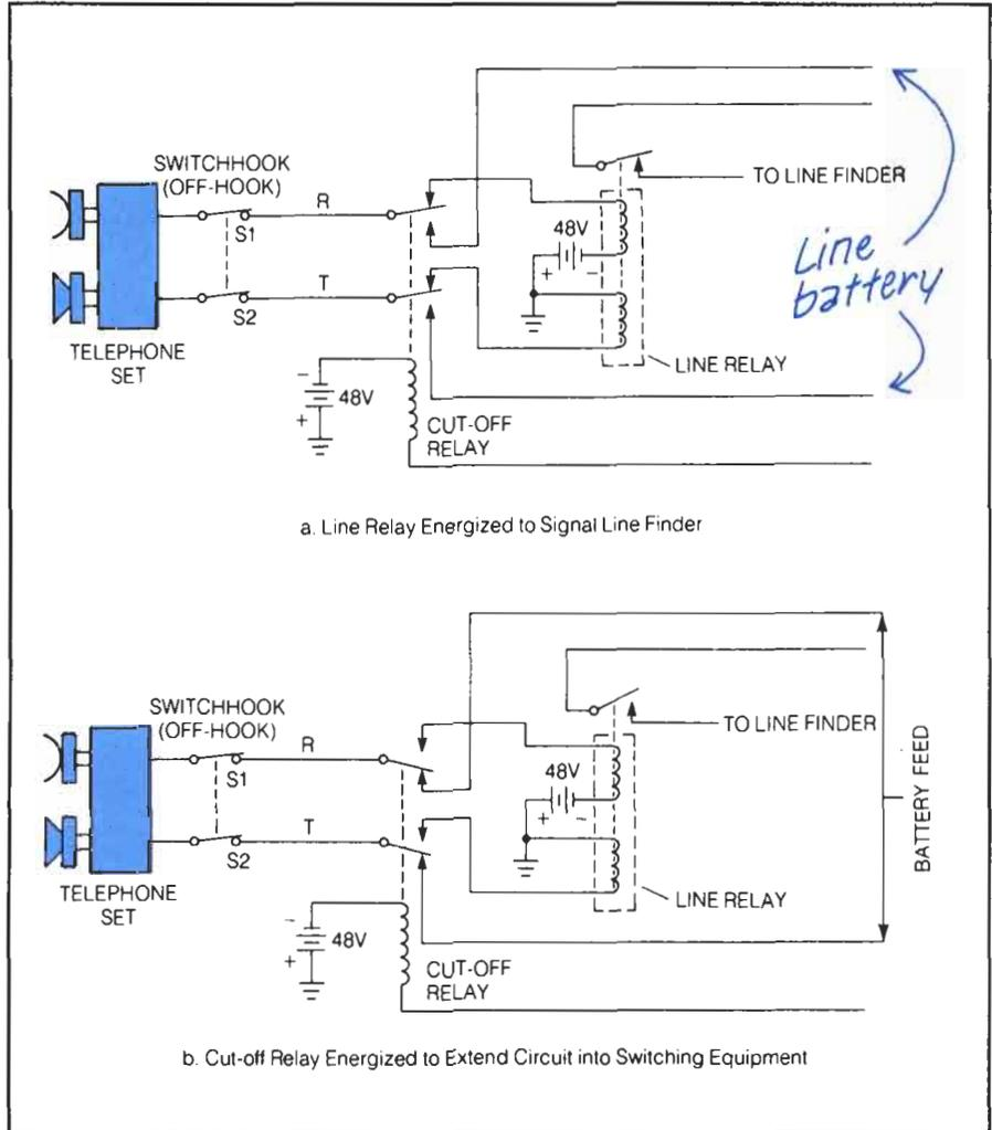
Three relays are used to supervise dialing. By using different relay characteristics, the circuit detects the difference between no current due to dial pulses and no current due to the handset being on-hook.
