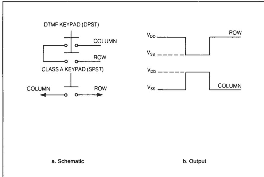
arranged to provide only a pulse, as is the case for a keypad that is used with a scanning sequence. The output waveforms are shown in Figure 4-10b.
