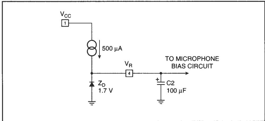
with the load. A zener diode provides a stable 1.7-volt reference voltage. External capacitor C2 is added to remove noise from the zener diode and to stabilize the output voltage.
