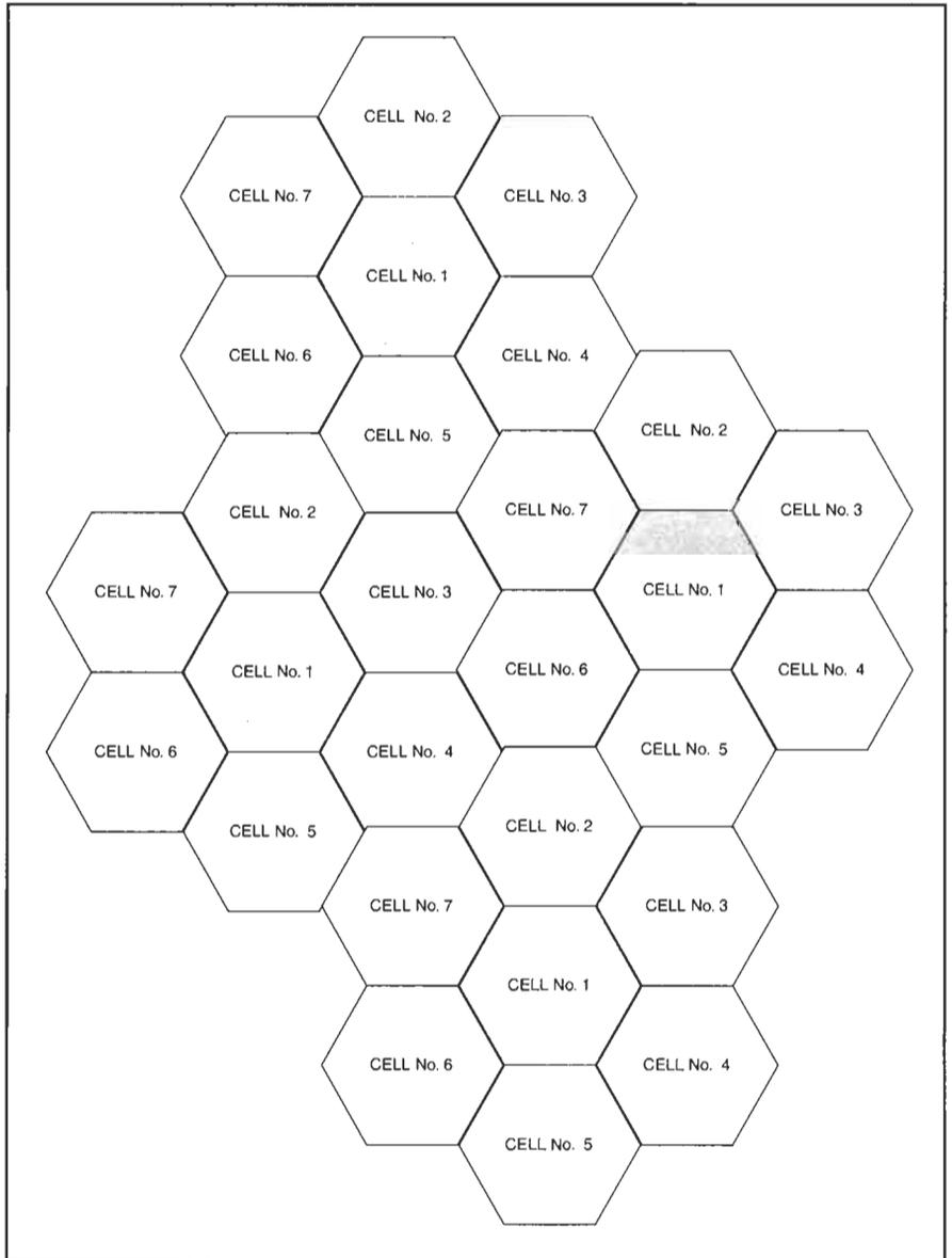
Whenever a mobile unit is turned on but not in use, the mobile control unit monitors the data being transmitted on a setup channel selected from among the several standard setup frequencies on the basis of signal strength. If signal strength becomes marginal as the mobile unit approaches a cell boundary, the mobile control finds a setup channel with a stronger signal.
