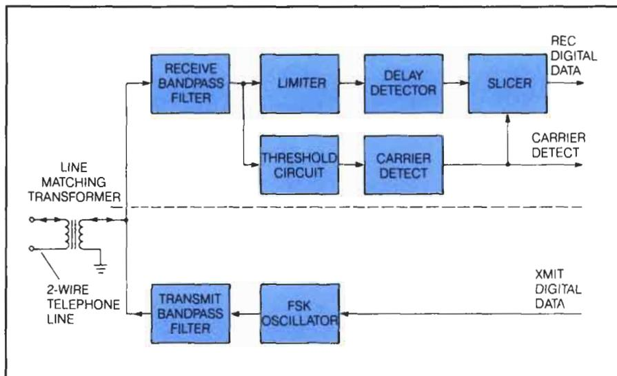
prevents the transmit signal from entering the receive section because the transmit and receive frequencies are in different bands. The receive bandpass filter also rejects noise and spurious frequencies riding on the receive signal from the telephone line. The limiter eliminates amplitude variations.
