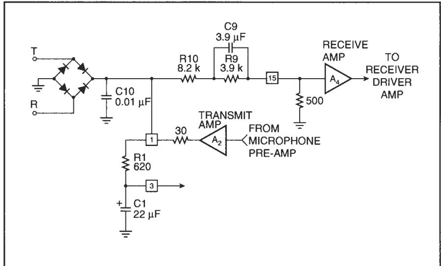
caused by other circuits. The equalization circuit comprising resistors R9 and R10 and capacitor C9 presents high impedance to line. The transmit amplifier (A2) has an open-collector output that presents high impedance to signals on its output (i.e., the line).
