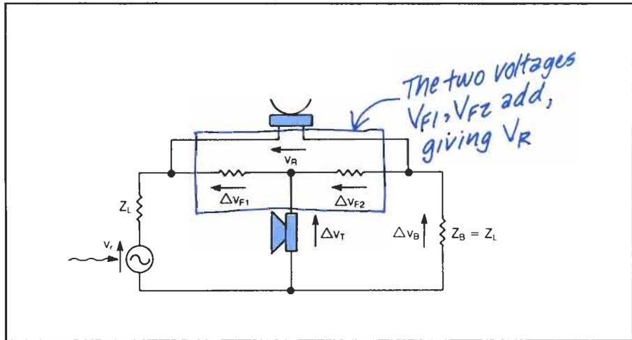
The receiver equivalent circuit of the telephone is represented by the source of emf in series with the load, feeding a series-parallel resistance network. Note that the actual voltage drop across the receiving device is now large enough to drive the device.
