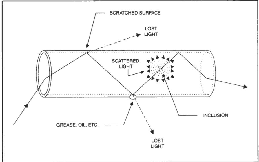
then it may act as if it were glass and cause loss of light to the outside world. Finally, there is always the possibility of *inclusions*: objects, specks, or voids in the material making up the optical fiber. Inclusions can affect both clad and unclad fibers. When light hits an inclusion, it tends to scatter in all directions, causing a loss. Some of the light rays scattered from the inclusion may recombine either destructively or constructively with the main ray, but most do not.
