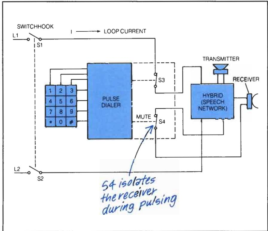
When a key is detected and verified, the binary code of the number is stored in internal memory. Certain dialer ICs may store anywhere from 16 to 20 digits per phone number. Additional control circuitry in the memory directs the location at which each digit is stored or recalled. Numbers stored in memory will be held until a new number is entered, or until power is removed from the dialer.
