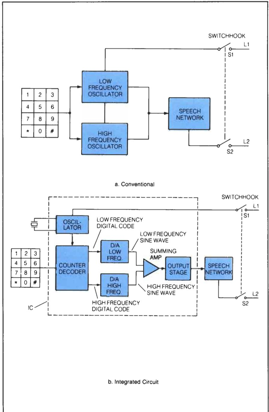
of the two outputs from the counter feeds into its own digital-to-analog (D/A) converter. The D/A converter, as the name implies, converts the digital code out of the counter to a sine-wave tone.
