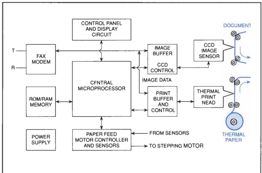
memory) holds results of calculations, variables, system status flags, or any information that will change regularly during normal operation. Figure 9-18 is a block diagram of a conventional microprocessor/memory configuration. The exact amount of memory will depend on the particular fax machine.
