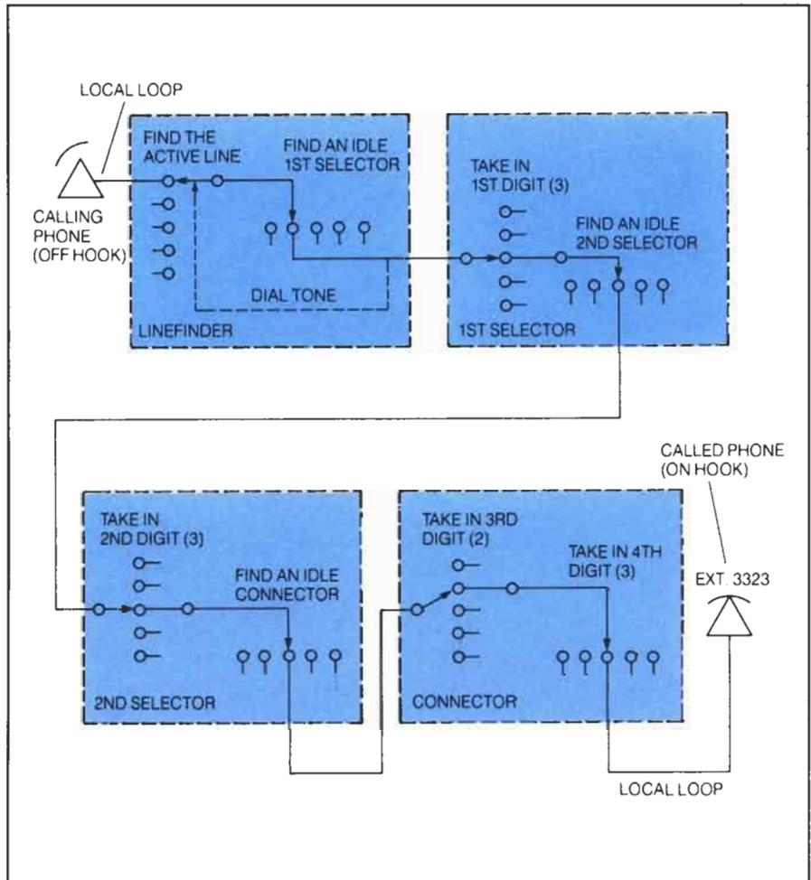
finder, first selector, second selector, and connector). A line drawing of a Strowger bank is shown in Figure 1-17.
