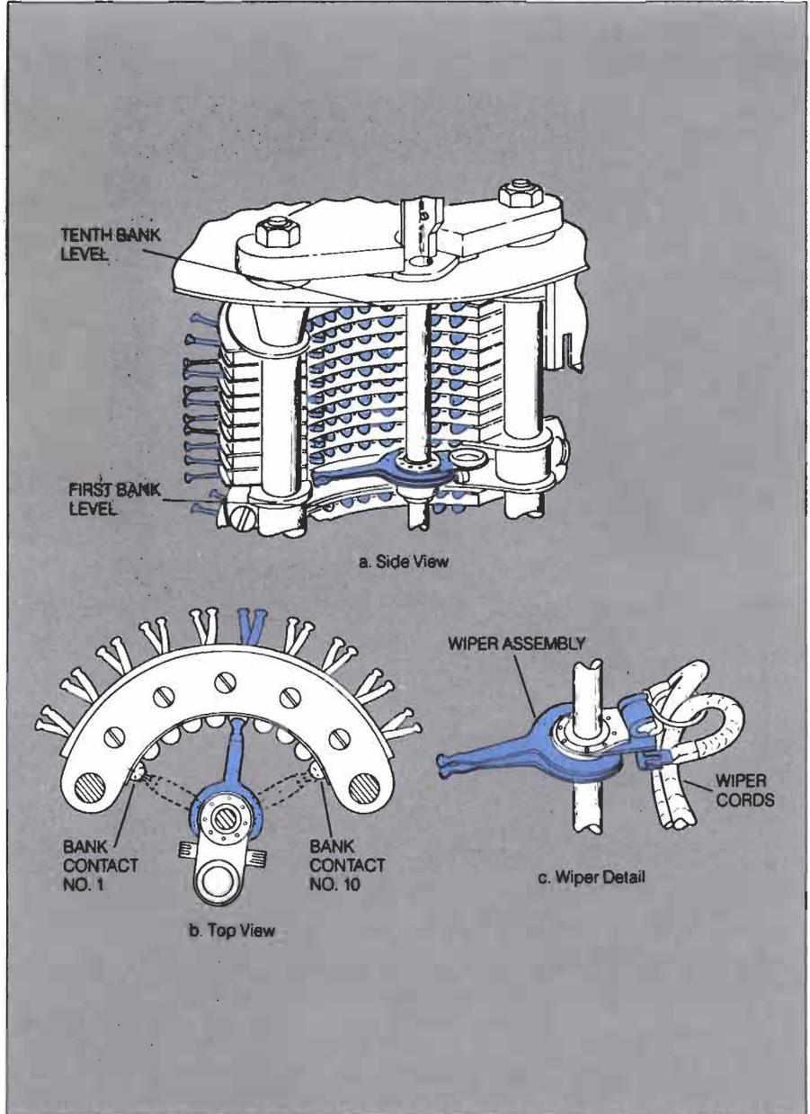
3. The switch requires the successful sequential (step-by-step, time related) operation of several relays, and a sizable voltage and current is switched each time a switch is stepped. Consequently, the mechanical reliability of the switches is low, they require large amounts of maintenance by skilled people, and they generate large amounts of electrical and mechanical noise.
