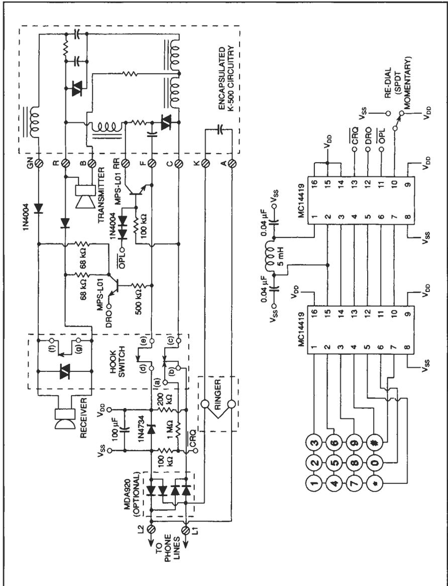
the Dial Rotating Output (DRO) becomes logic high. This shuts off the transistor, providing a current path to the receiver and effectively mutes it. DRO will stay high while digit pulses are being sent. Dial pulses (Figure 4-8) are sent through the Outpulsing (OPL) pin, which switches a diode-transistor
