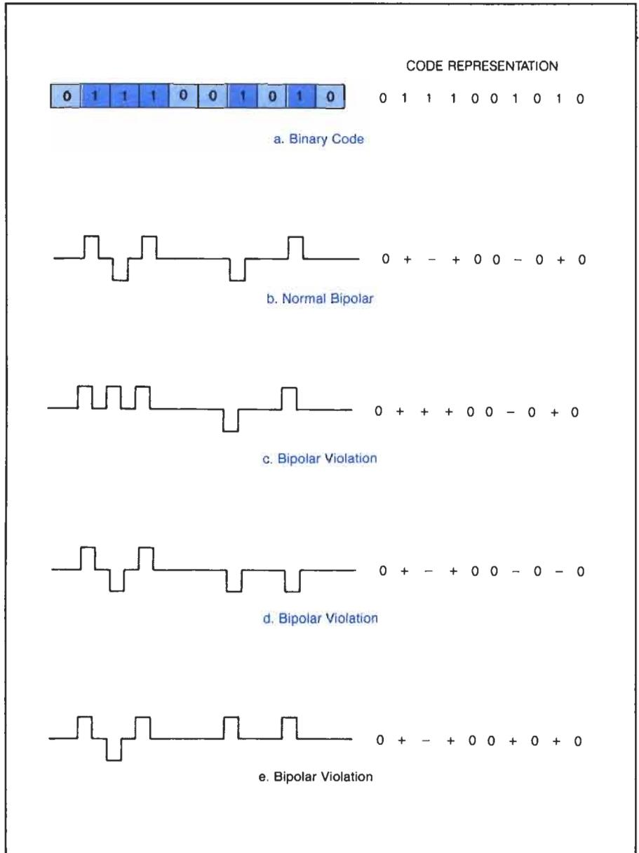
polarity of the 1 pulse immediately preceding the string of six 0s. Note also that in the substituted code, a built-in bipolar violation is caused by the substitution of the second and fifth pulses. When the second pulse is substituted it causes a
