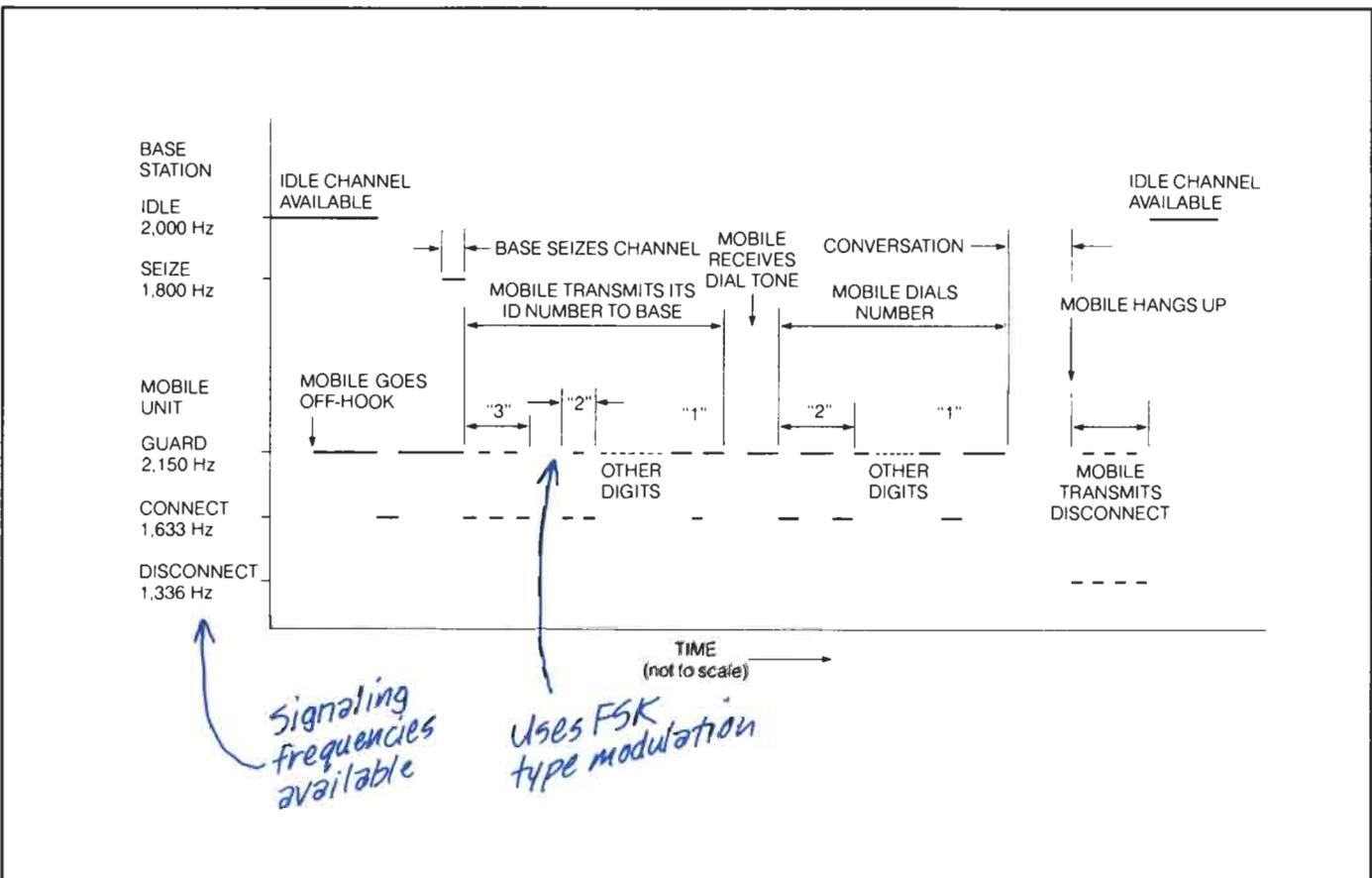
When a call is originated from the field, the mobile unit finds a marked idle channel and broadcasts an acknowledgment to the base by sending its identification. The mobile unit then completes a call in the usual manner by receiving a dial tone, dialing the number, and waiting for the called party to answer.
