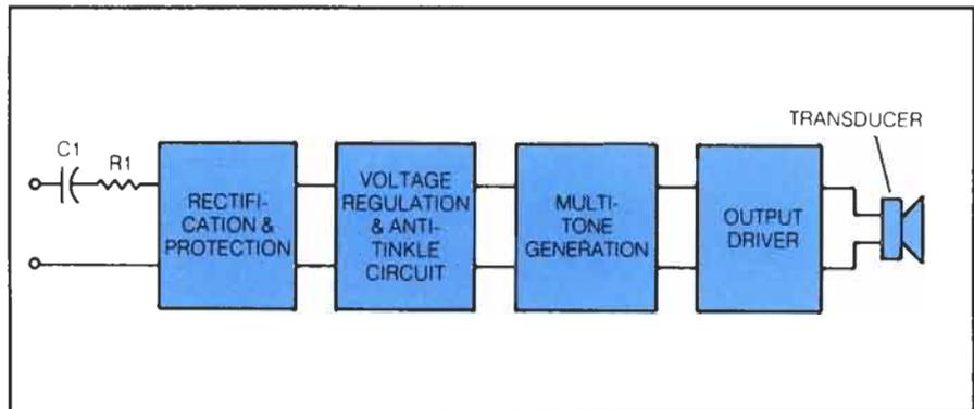
Voltage regulation in the multitone ringer permits normal ringer operation over a wide range of voltages.
