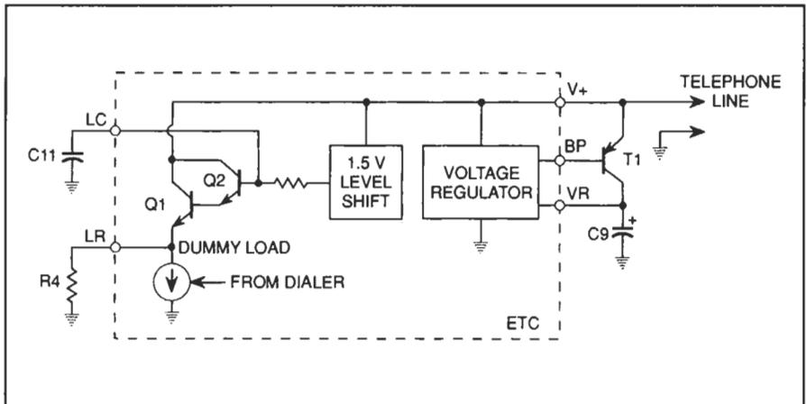
The line interface regulator controls the voltage and current delivered to the entire telephone circuit.
