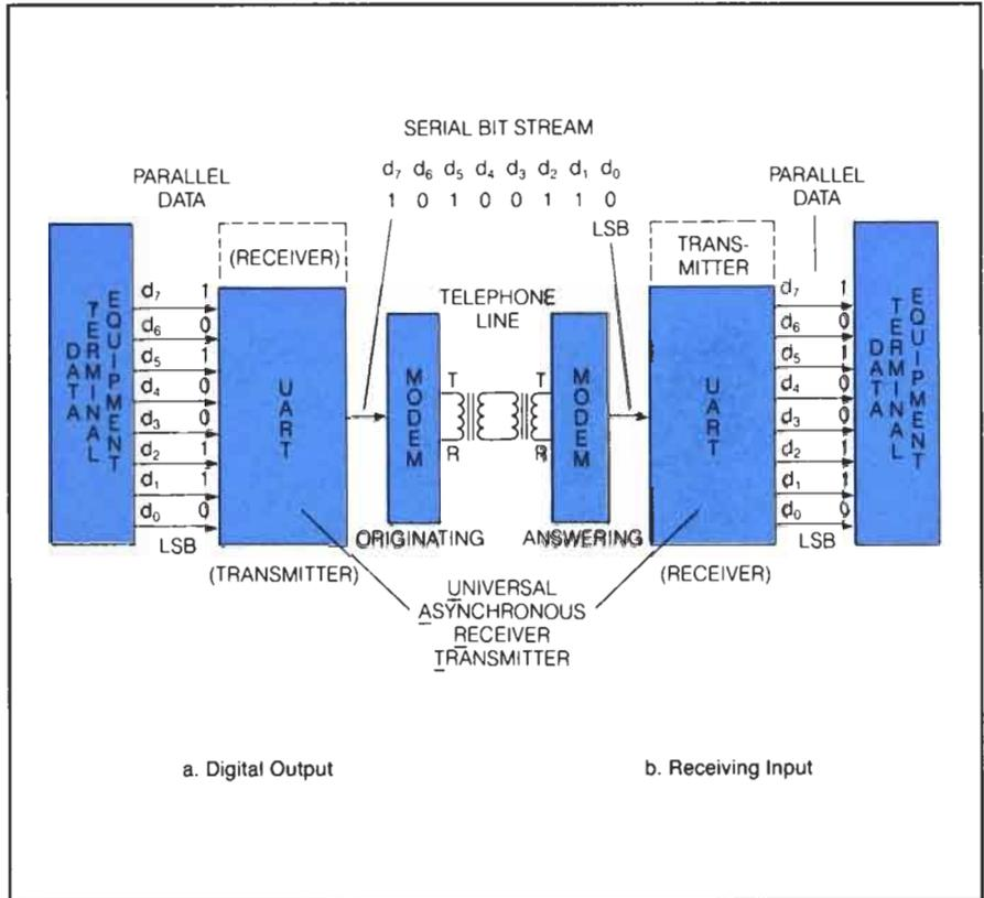
The serial bit stream cannot be transmitted directly, but must be changed to tones that can be sent over the telephone line. A modem provides the conversion and coupling to the telephone line. The word modem is a combination of the words MODulator and DEModulator, the two principal functions accomplished by a modem.
