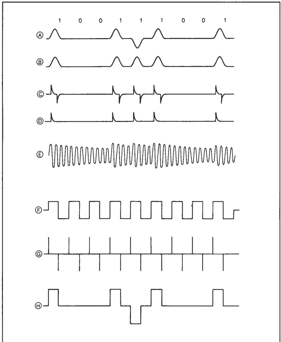
for the amplifiers for the previously used analog carrier system that T1 replaces. Thus, the same manholes can be used when a system is replaced. The energy in the DS-1 signal is concentrated at 772 kHz, which gives a loss figure of 26.6 dB at 6,000 feet over 22-gauge paired wire cables.
