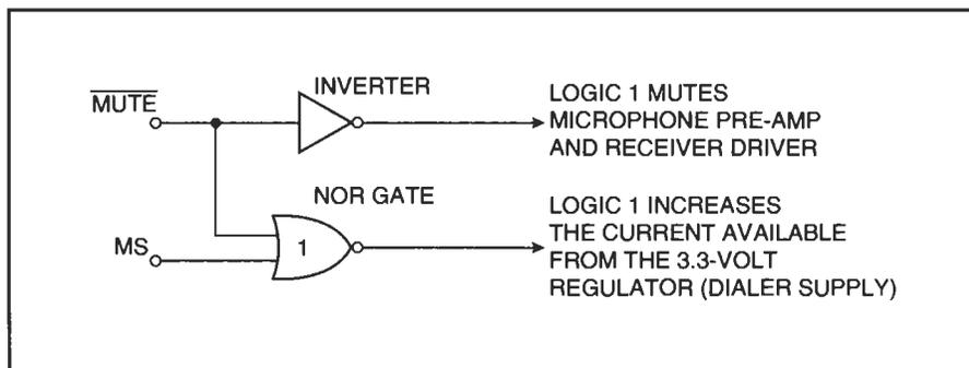
When dialing, the mute signal will become logic 0. The inverter produces logic 1 and disables the receiver driver. If the mode select signal is also at logic 0, signifying tone dialer mode, the NOR gate will output a logic 1. The NOR gate controls the current available from the 3.3-volt regulator (dialer supply), and increases it to 2.5 mA when the NOR gate output is logic 1. The 1.5-mA increase in current is drawn from the loop compensation circuit, as described earlier.
