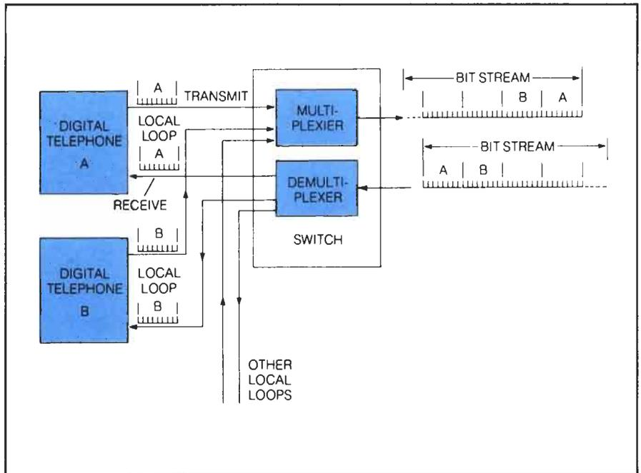
multiplexes these and other signals into one continuous bit stream. (This process is explained later.) The bit stream is transmitted in serial form to a demultiplexer switch at the destination. This is shown as the receive function in Figure 6-6. The switch separates the individual signals from the bit stream and routes them to the proper telephone set.
