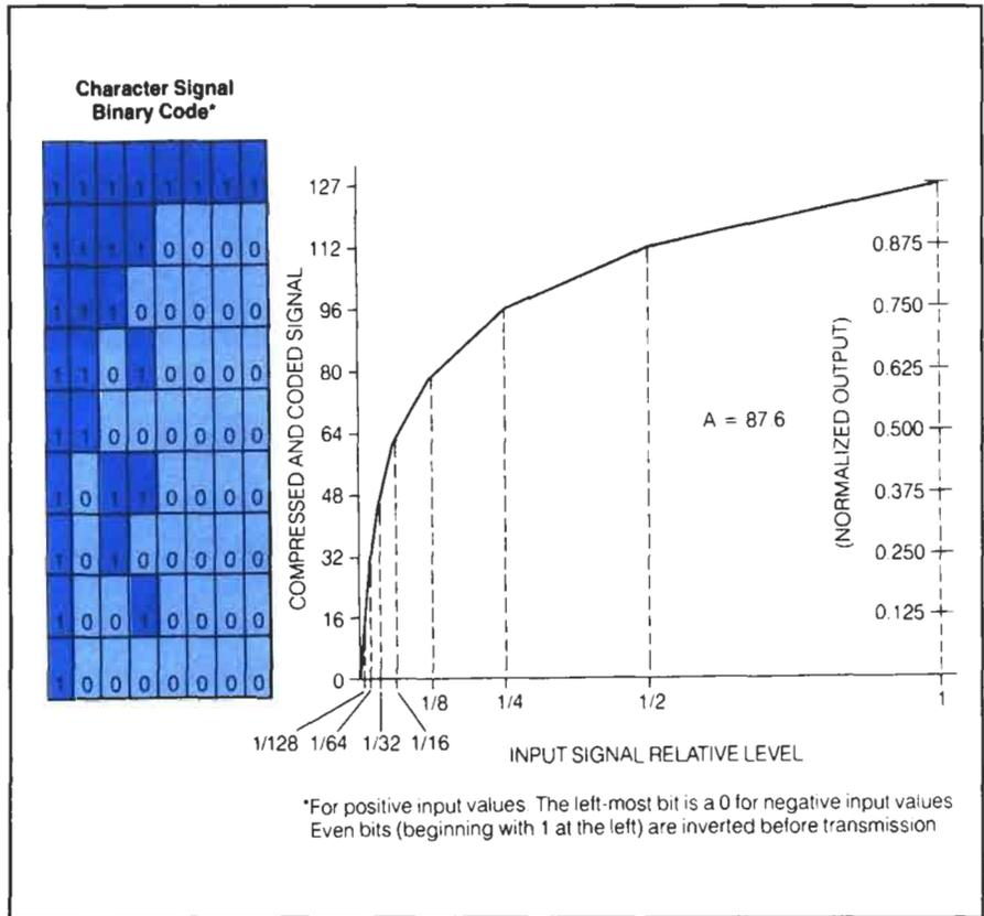
transmitting any waveform, as long as its bandwidth is limited to what the chosen sampling rate can encode without error. The capability to accurately transmit any waveform is obtained at the cost of sending enough bits to encode the entire sample at every sample interval.
