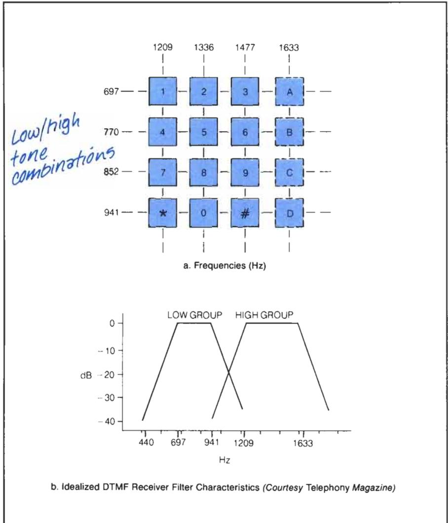
The filtering section provides for gain and for noise and speech rejection.
