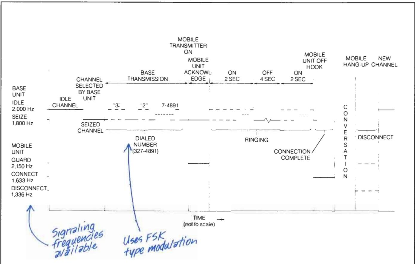
When the land-originating call reaches the control terminal, the idle tone is replaced by a 1.8-kHz seize tone which seizes the reserved channel. The control terminal then sends out via the transmitter the mobile unit's number.
