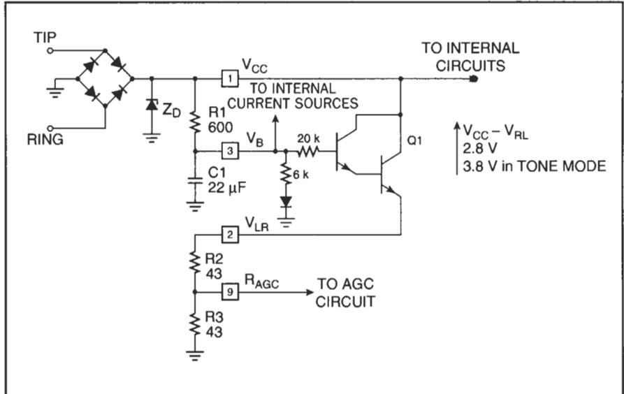
between  $V_{LR}$  and ground is calculated for a given line voltage and current, allowing a 1.4-volt drop across the bridge rectifier and 2.8 volts across transistor Q1. This resistance is the sum of the values of R2 and R3. The value of R3 is then selected so that AGC circuit reduces the gain of amplifier stages on short lines.
