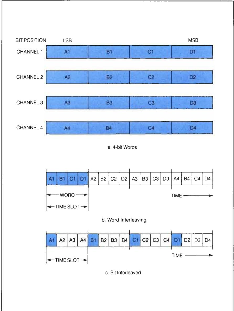
code words as outputs from each digitized channel. The higher level multiplexers in the public network are bit interleaved because the data sources are continuous bit streams from the lower level multiplexers.
