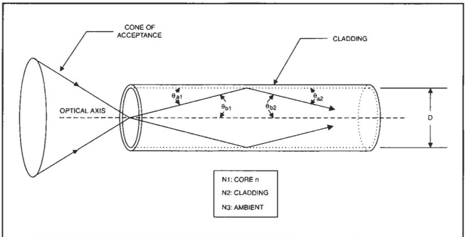
The refraction angle of the rays internally, across the air- $n_1$  interface, is given by Snell's law:
