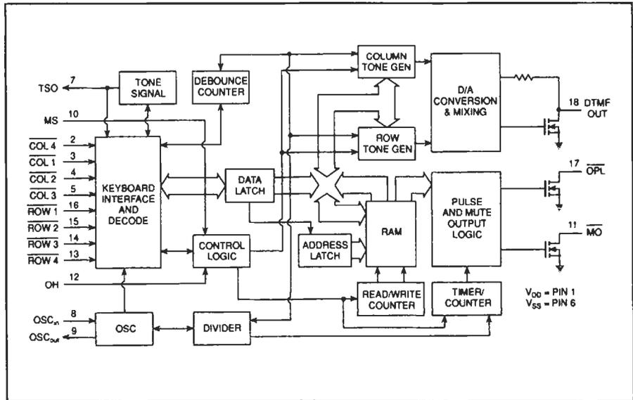
or  $4 \times 4$  keypads. A single input pin will select between DTMF, 10-pps, or 20-pps dialing. An internal memory can hold up to 10 complete telephone numbers, each up to 18 digits long—this includes last number redial. Finally, the dialers operate on line power as low as 1.7 volts. This makes them very closely compatible with the MC34014 integrated speech network covered in Chapter 3.
