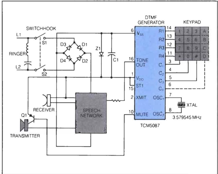
power to the IC and Z1 protects against transients. The capacitor C1 maintains and filters the voltage across the IC to eliminate noise and supply variations. A mute signal controls Q1 and mutes the transmitter of the speech network. The XMIT output on pin 2 and the ST1 input on pin 15 were described in the discussion of Figure 4-11.
