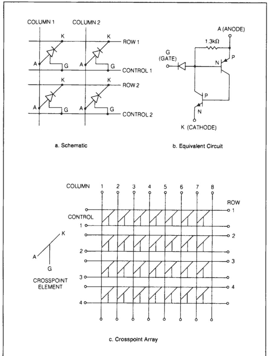
The connection is made as follows: First,  $I_H$  for the top section is enabled. Second, the logic gates, either  $G_A$ ,  $G_B$  or  $G_N$ , turn on so that current can be drawn from gate to anode on the respective crosspoint elements. Note that any combination of crosspoints may be used to establish a path through the arrays.
