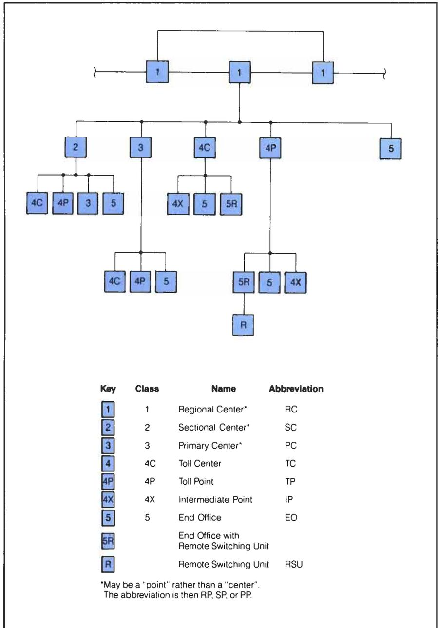
The ten regional centers (Class 1 offices) in the United States and two in Canada are connected directly to each other with large-capacity trunk groups. North America has 67 Class 2, 230 Class 3, 1,300 Class 4, and about 19,000 Class 5 exchanges.
