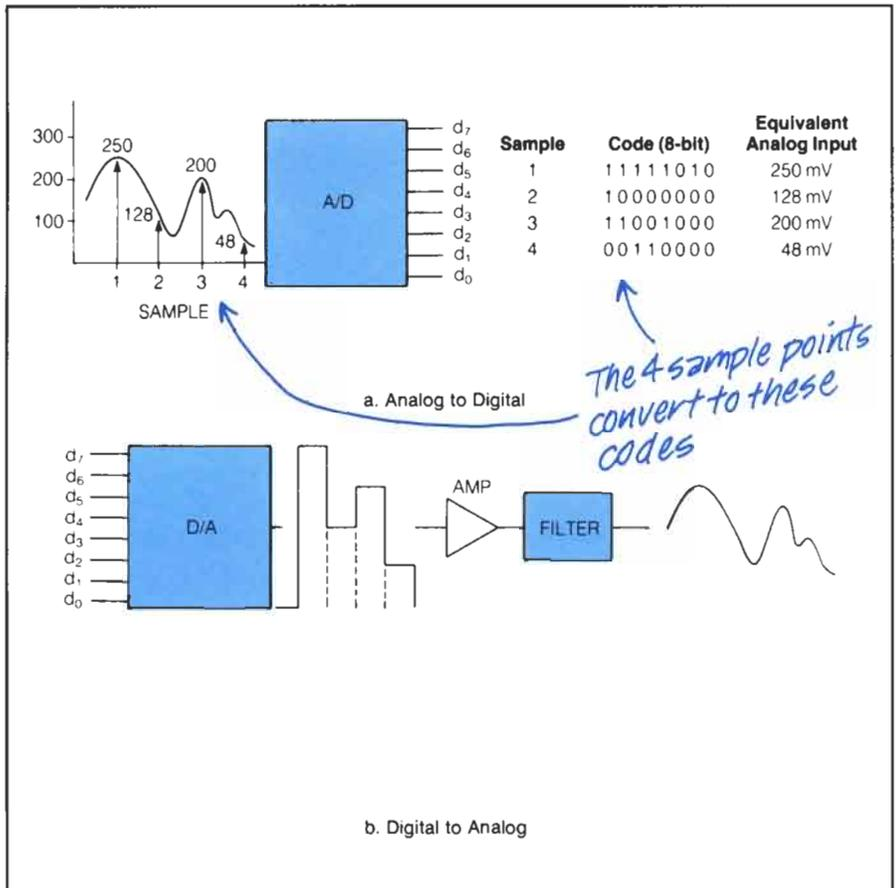
To convert a digital signal to analog, the D/A converter takes the digital signal and outputs an approximately similar, but stepped signal to an amplifier/filter network, which smooths the output and provides a nearly perfect replica of the signal.
