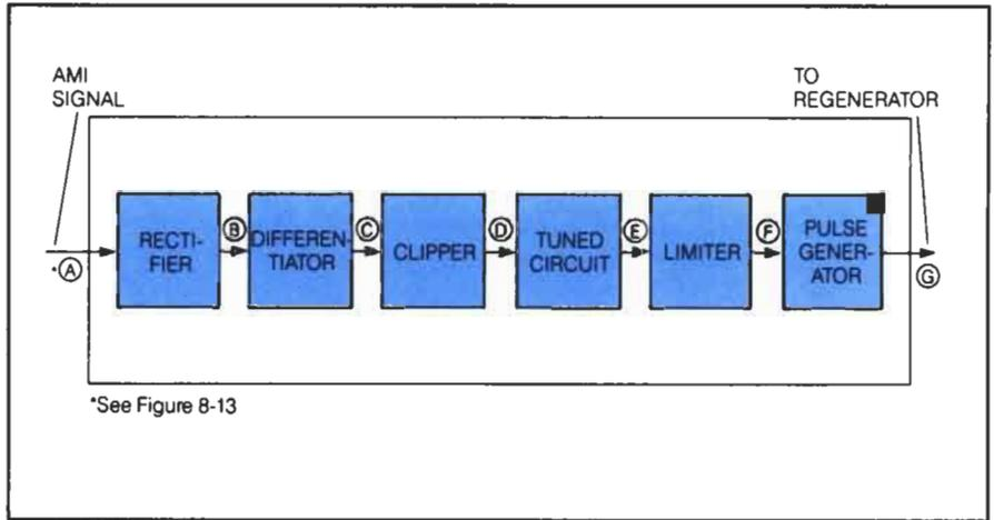
In the timing circuit, clock recovery is accomplished by processing the incoming data signal. The input signal is rectified, differentiated, and clipped.
