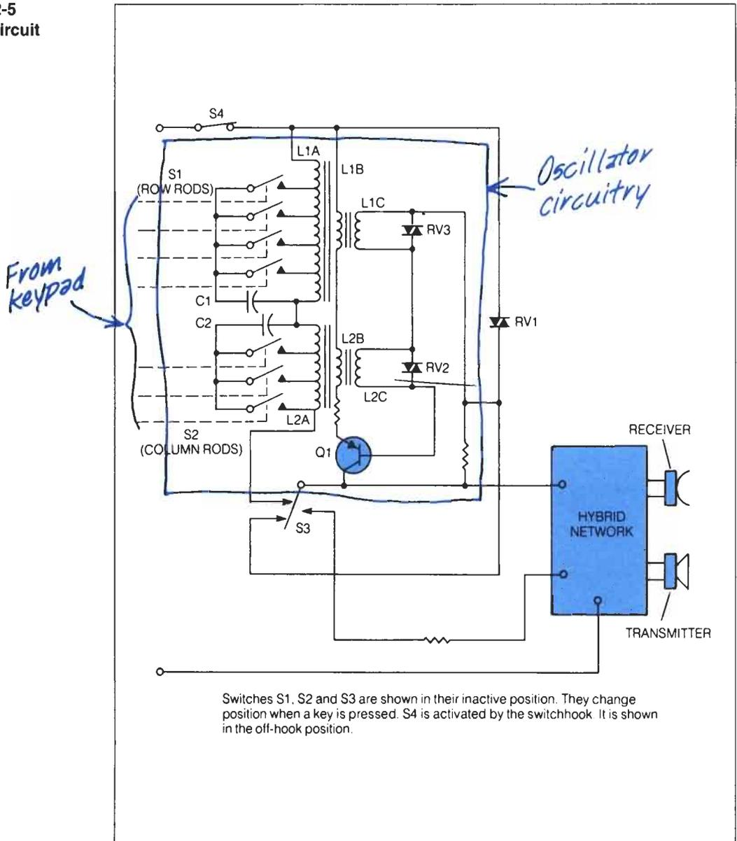
the loop current to transmit the two tones to the central office. The transmitter and receiver are shunted when S3 switches, but the outgoing tones can still be heard in the receiver at a low level. Modern DTMF tones are produced with integrated circuits instead of discrete oscillator components.
