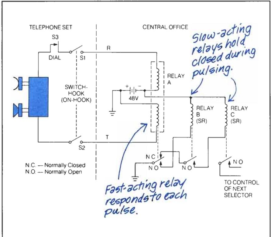
(ms); thus, the B relay is held energized as long as the subscriber is off-hook and indicates, by releasing, when a subscriber hangs up.
