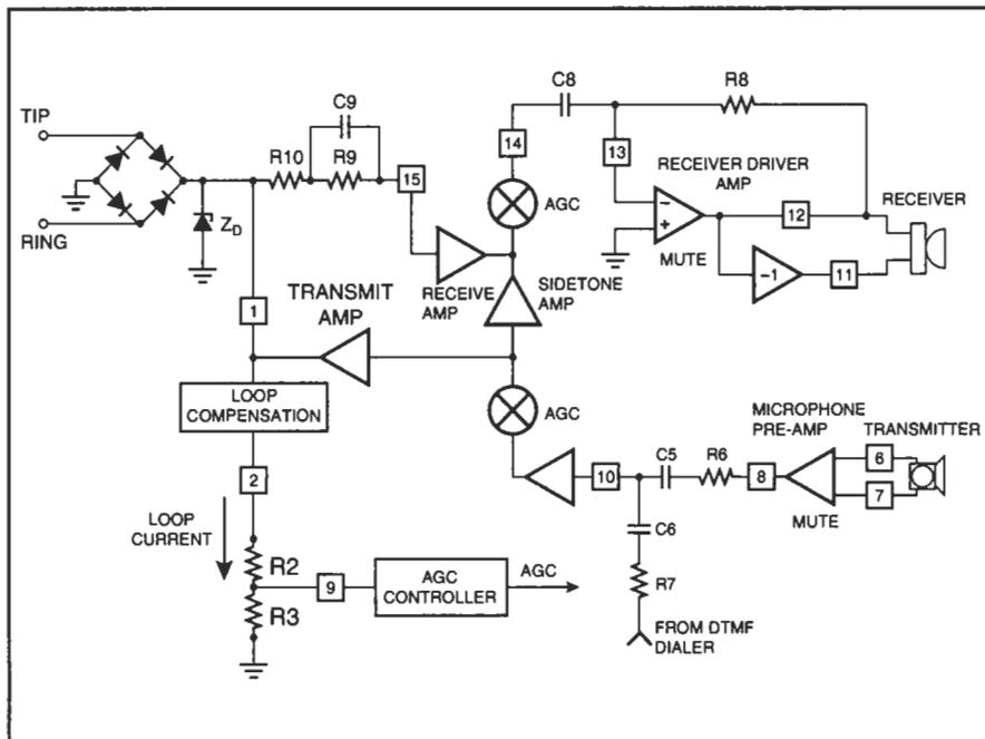
$C_9$ ). The MC34114 is designed to work with a high-impedance electret microphone, although a low-impedance dynamic microphone can be used.
