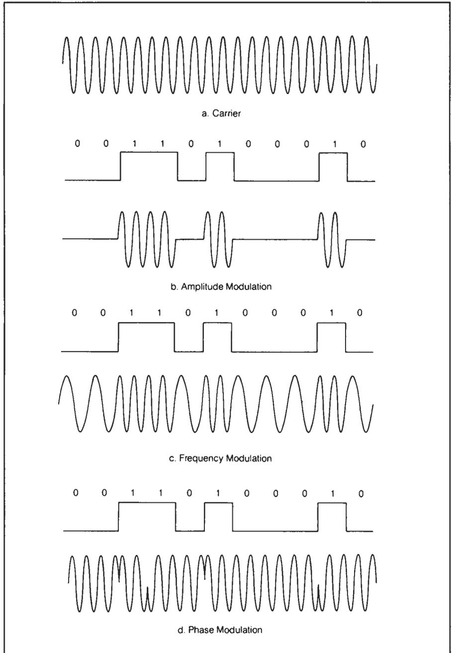
In demodulation, the telephone signal is processed to recover the original digital stream of 1s and 0s.
