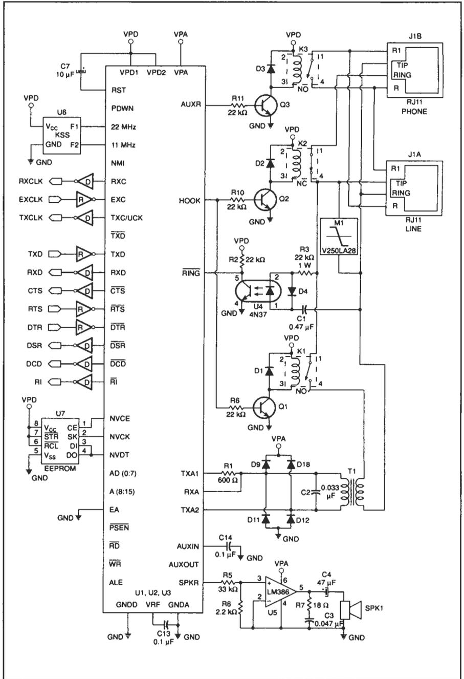
The SSI 73D2291/2292 frames its data using the high-level data link control (HDLC) protocol. It also supports error checking and correction by adding a frame check sum to the data stream. Fax operating sequences are similar to (but are more complicated than) those required for conventional modems since fax operation needs format conversion and file compression steps in addition to normal data transfer.
