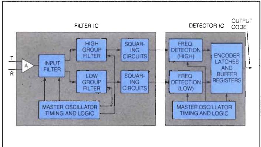
Each DTMF frequency is tested to ensure its validity and if valid is output as a code to represent the dialed number.
