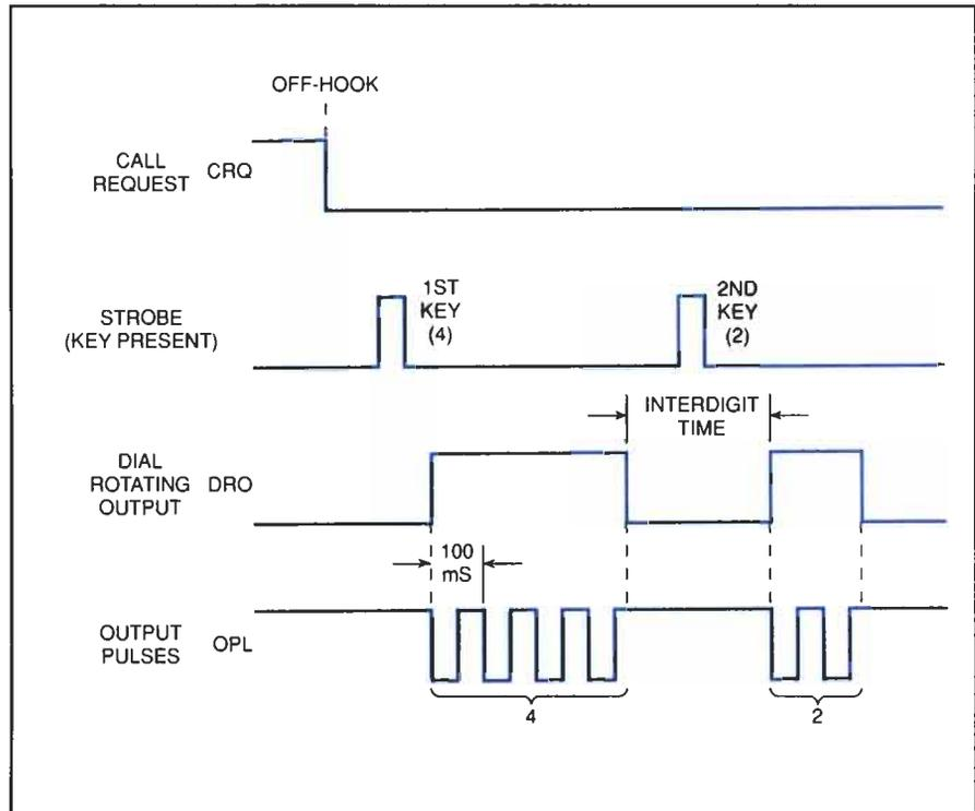
network on and off to interrupt loop current. The central office interprets these current pulses as digits.
