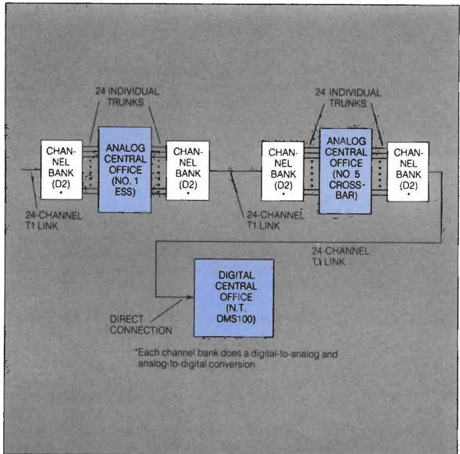
Interfacing digital hardware with existing analog equipment creates some problems. Digital hardware operates on low voltages and currents, and is quite susceptible to the signal spikes generated by the existing high-voltage equipment.
