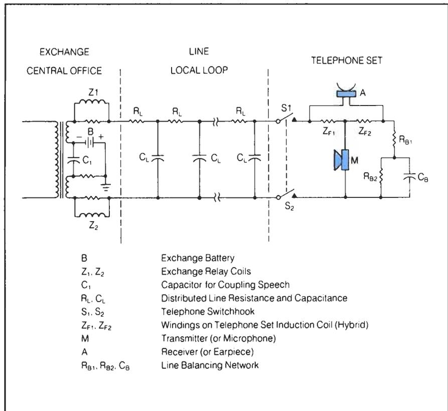
The transmission equivalent circuit of the telephone is represented by the transmitter being the source of emf, feeding a series-parallel resistance network. Note that net voltage drop across the receiver is about zero.
