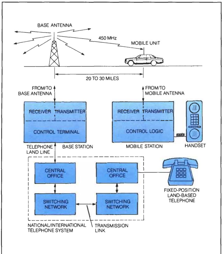
The base unit receiver contains the necessary electronics to present its control terminal with a good audio signal. The control terminal interfaces the voice and control signals to the standard telephone circuits.
