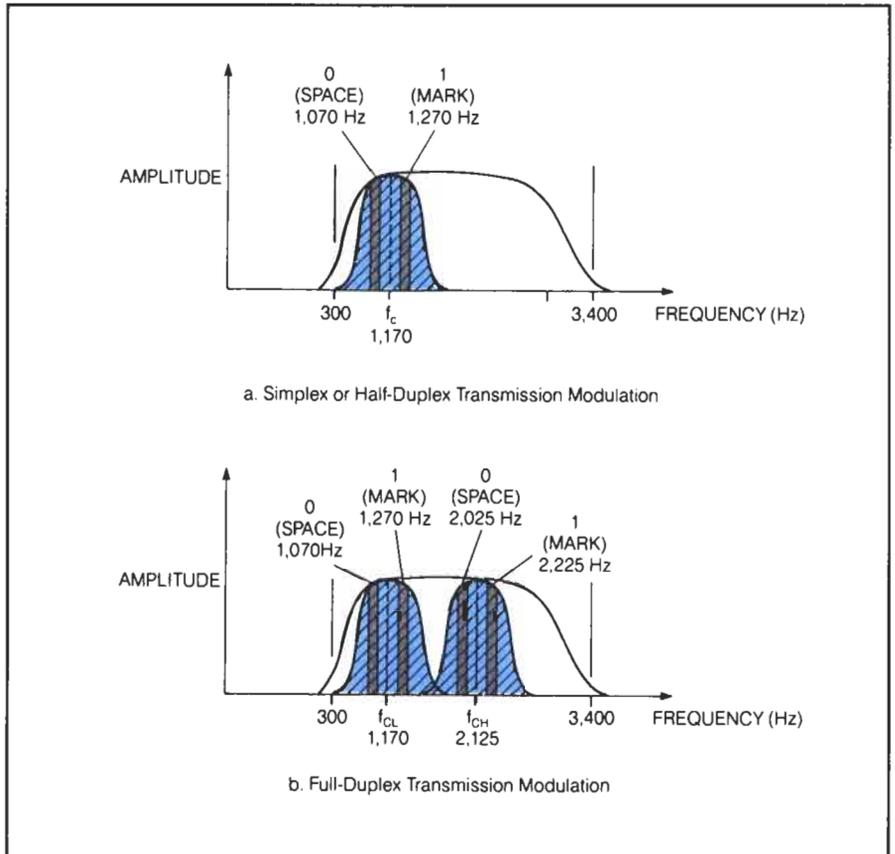
In the Bell 202 modem, the mark and space frequencies are widely spaced because of the increased bandwidth requirements of a higher data speed.
