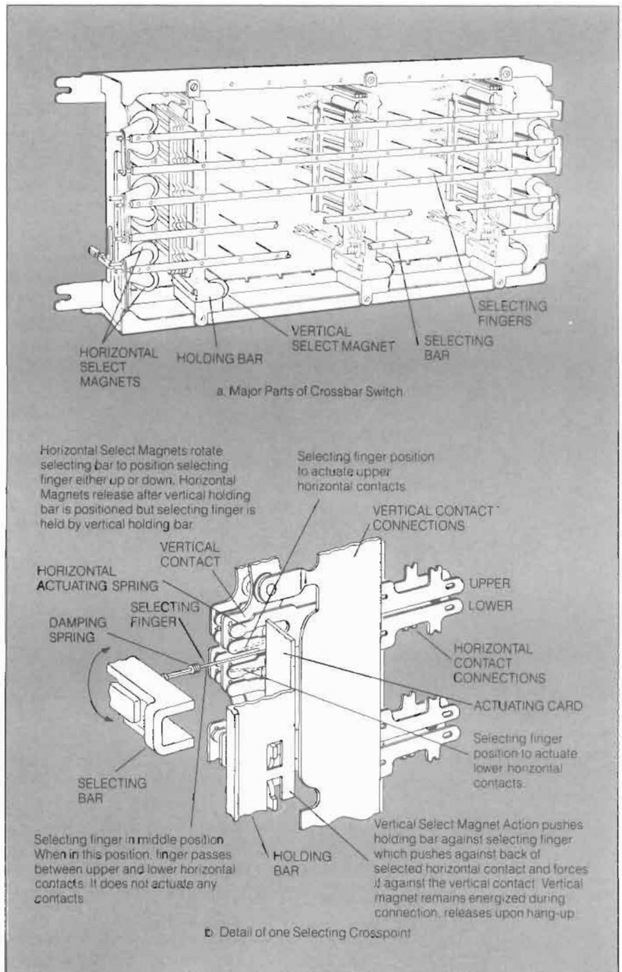
to its idle position, but the previously selected finger is held by the vertical holding bar. When the calling end goes on-hook (hangs up), the vertical select magnet current is interrupted and the crosspoints are released. Thus, the calling party controls the connection.
