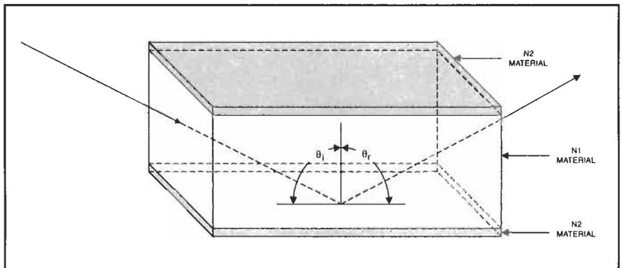
the illustration, the ray will be subjected to successive TIR reflections as it propagates through the  $N_1$  material. The proportion of light energy that is reflected through the TIR mechanism is on the order of 99.9%, which compares quite favorably with the 85 to 96% typically found with plane mirrors.
