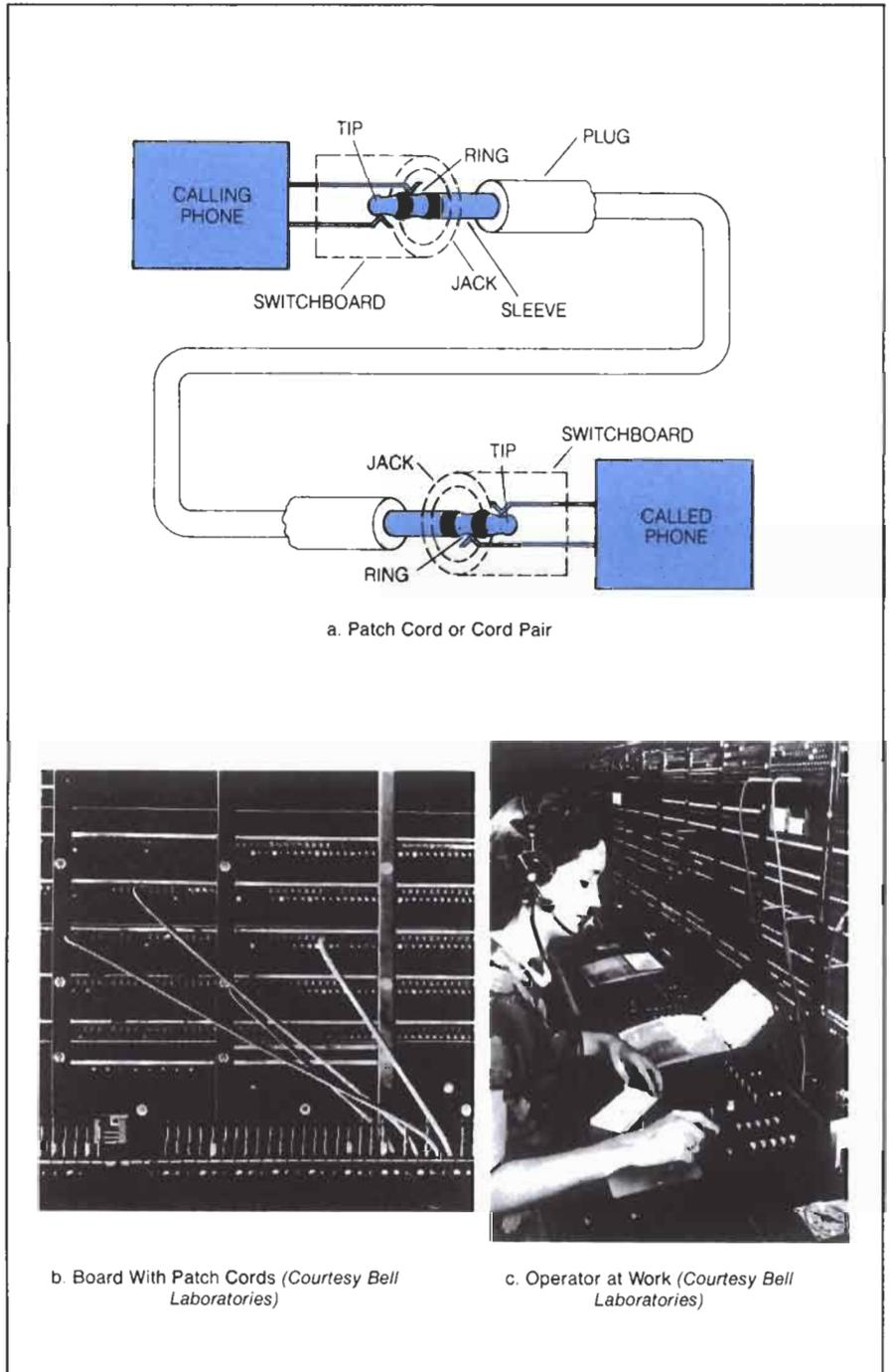
requesting service, obtained from the calling party the name or number of the desired party, then plugged the other end of the cord pair into the correct outgoing line jack. Many thousands of cord switchboards are still in operation, a tribute to the versatility and ease of programming of the control system, and the personal touch it provides. However, not every subscriber appreciated the personal touch.
