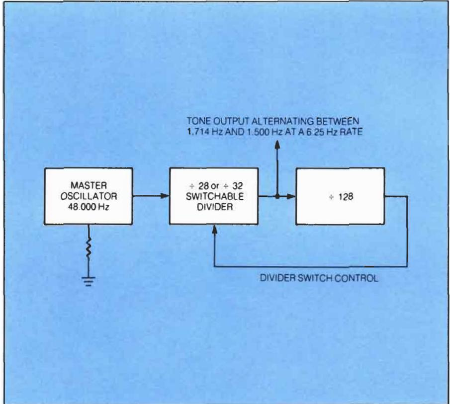
and input to the shift rate divider is 1,500 Hz. The shift rate divider then counts 128 cycles at 1,500 Hz and returns the programmable divider to divide by 28. This cycle repeats as long as the ringing voltage is present on the line.
