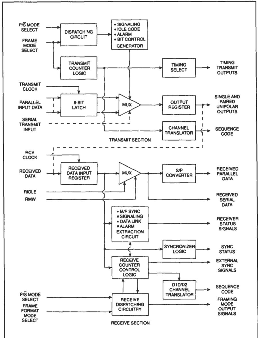
Eleven modes of operation are available to support most common former variations of T1 and CEPT formats. A microprocessor can interface easily with the R8070 to enhance control and the serial or parallel transfer of data. This device represents a tremendous savings in component costs and system
