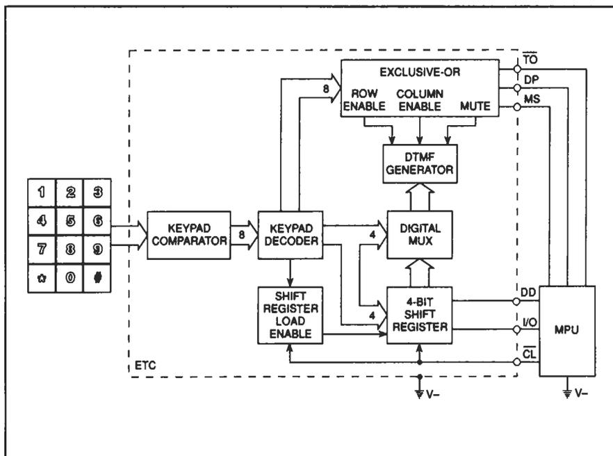
clock pulses sent over the CL line by the microprocessor. It also manages the direction of data flow using the Data Direction (DD) pin. In this way, dialing activities of the telephone circuit can be supervised. Whether the microprocessor reads or writes key data will depend on what particular function it is performing and how it is programmed.
