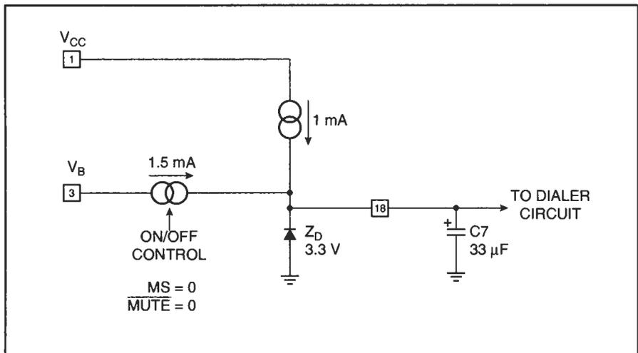
When in tone dialer mode (Mode Select input and the Mute input both set at logic 0), a second constant current circuit provides an additional 1.5 mA. This current is drawn from the bias point ( $V_B$ ) of the loop compensation circuit.
