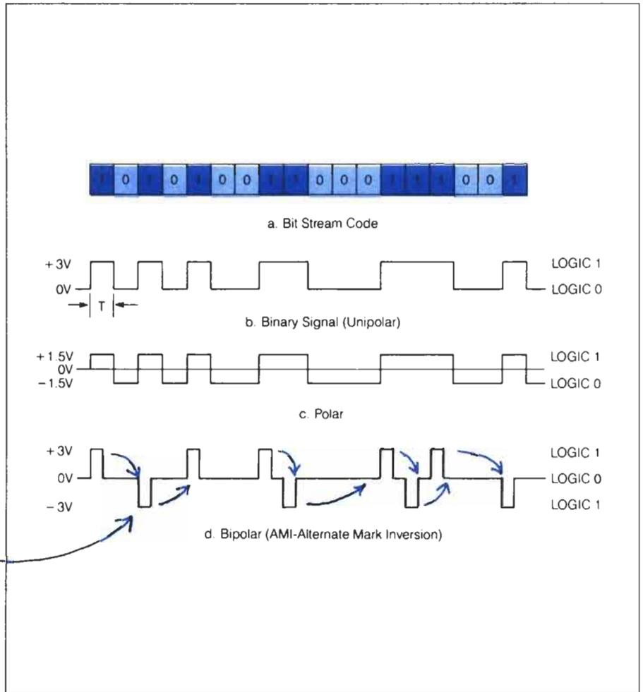
component is present is shown in Figure 8-10. Long sequences of 1s or 0s can cause a shift in the waveform amplitude with respect to 0 volts. When this occurs, signal recovery circuits that are detecting the 1s and 0s lose proper amplitude reference and errors occur. Special circuits called dc restoration circuits are designed to eliminate the dc wander and restore the proper reference levels.
