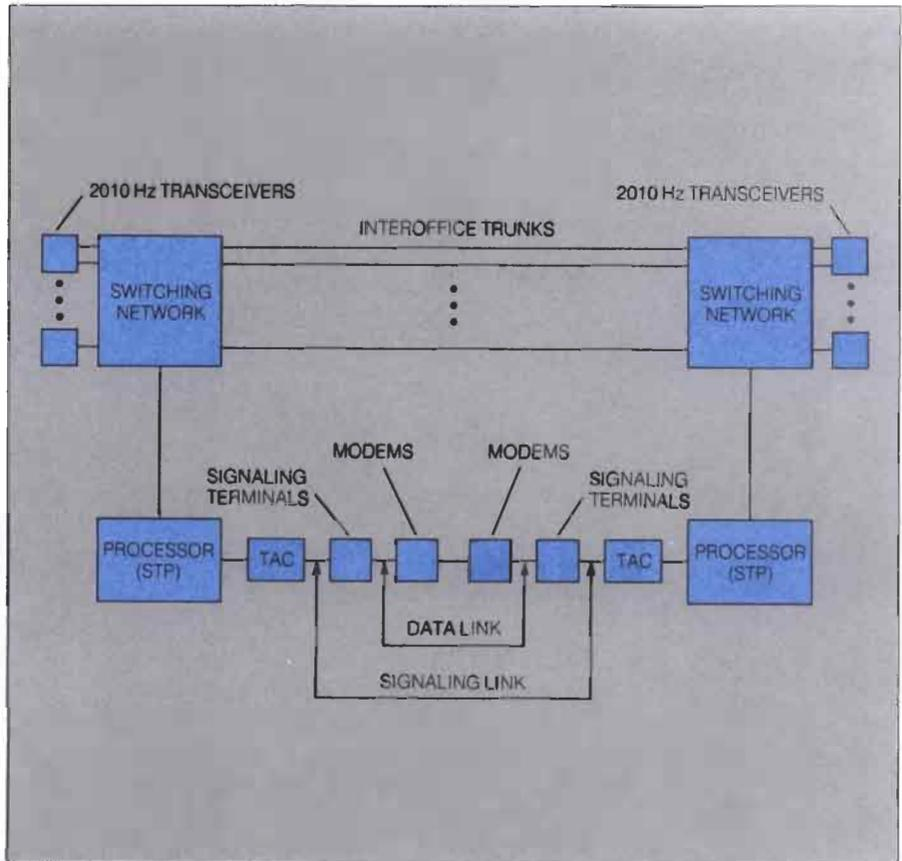
The CCIS link consists of a terminal access circuit (TAC), a signaling terminal, and a modem (discussed in Chapter 6) at each exchange; and a channel to a control computer called a signal transfer point (STP). Several exchanges may be interconnected with two or more STPs for backup protection against equipment failure.
