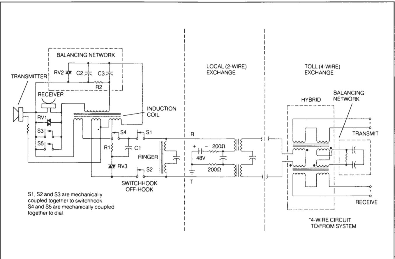
The hybrid circuit permits the interfacing of a 2-wire with a 4-wire system. Normal full-duplex operations can still be maintained.
