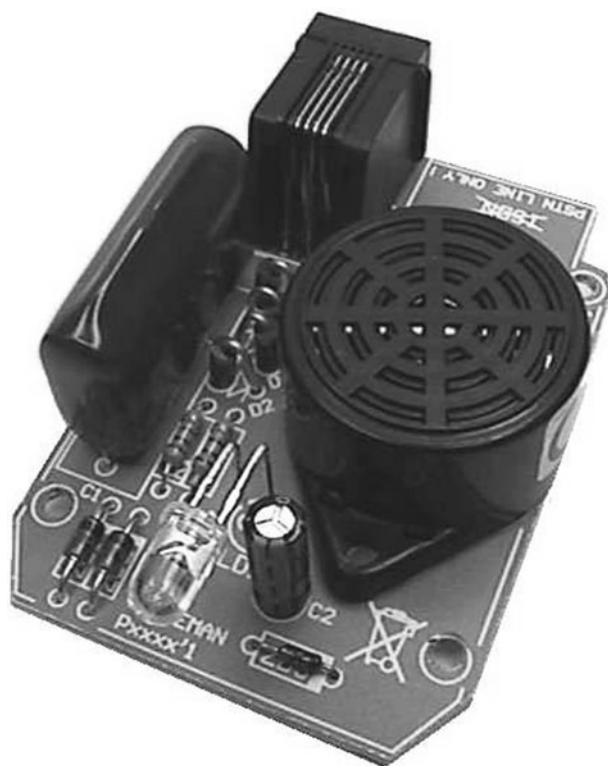
Figure 13-2 Remote telephone ring indicator. Courtesy of Velleman Kits
