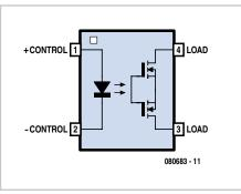
package. When choosing a relay for a particular application the description will include the specification 'X form Y'. X is a number indicating how many switches are in the package and Y indicates the type of contact: 'B' = normally closed while 'A' = normally open. Some of these relays have both normally open and normally closed in the same package, useful for making a changeover switch.
