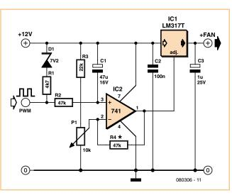
signal originates from an open collector output which can only be pulled up to a maximum of 5.5 V. For this reason R1 is connected in series with a zener diode to limit the pull up voltage to 4.8 V. The PWM signal is integrated by the network formed by R2 and C1. The resulting signal is amplified by an opamp (almost any type that can work at 12 V will do here). The opamp output signal controls an adjustable voltage regulator which supplies sufficient current even for the most powerful fan.
