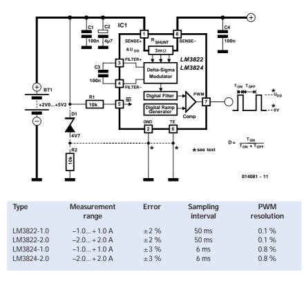
5.5 V, the Zener diode shown in dashed outline in the schematic diagram can be use with a 10-k $\Omega$  series resistor. The Zener diode limits the operating voltage across the LM3822/24 to a safe 4.7 V. Note however that in this case, the output signal is not longer referenced to ground, but swings between the supply voltage level and 4.7 V below this level. A level converter is thus needed for signal processing. The GND and Test (TE) pins should be connected to the zener diode.
