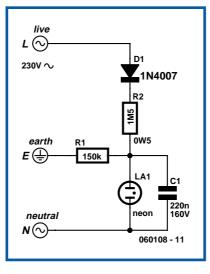
devices are frequently in wet conditions, the screw and/or lug used to connect the earth wire to the device frame corrodes gradually and ends up breaking or causing a faulty contact. The remedy is then worse than the problem because the user, thinking that he/she is protected by earth, does not take special precautions and risks his/her life.
