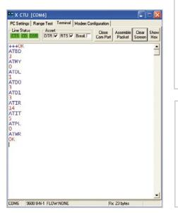
(from 1083 to 10A2). If you immediately perform a Write with the new version, you will lose communication with the module because the configured parameters will be overwritten.
