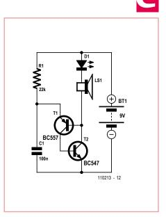
the LED cathode and the PNP transistors base to ground, reinforcing the ON condition of the PNP transistor and causing a relatively high current to pass through the LED to emit a flash.
