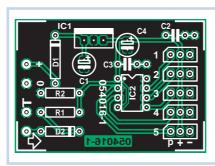
D1 in order to juice the craft battery. The servos are connected via the usual 3-pin connectors. As servo manufacturers use different pinouts for pulse (p), ground and +5 V on their connectors, you should check the data available.
