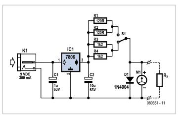
ist equipment is expensive. The simple circuit described here allows milliohm measurements to be made safely on a standard multimeter. The circuit consists of little more than a 6 V voltage regulator and a mains adapter capable of supplying around 300 mA at 9 to 12 V.
