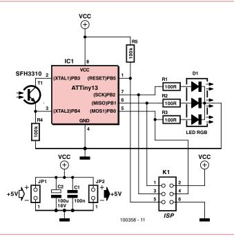
voltage level is read by the ATtiny13 microcontroller through an ADC channel at pin 3. The circuit is designed for a 5 V power supply and has no integrated power regulator. The supply voltage is taken from a 'rail' created by plug-
