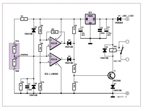
had the same key, which is clearly not a good idea! So you need to decide for yourself not only R4 and R8, which form the key, but also R1 and R9 which let you customize the 'lock'. Here are the relationships between the values of resistors R1, R4, R8, and R9 for the key to be able to open the lock:
