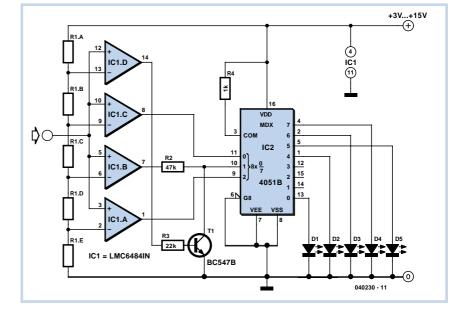
shorting it to 0 V, thus overriding IC1.B's output pin 7. This creates one additional binary input number (binary 101) for IC2, and adds a fifth stage to the bargraph. A 'logic' MOSFET such as a BUZ11 or IRF510 would also work in this position, and in this case R1 may be omitted.
