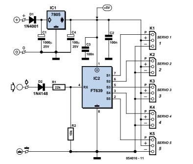
to the device using software and the PC's printer port (LPT:). The 'get-to-know-u' program can be downloaded from the Elab Inc. website (see below) and should not be too difficult to convert into PIC or AVR code. On the same website we also found a Visual BASIC programming example complete with source & executable code to illustrate how the edeFT639 servo controller can be driven via Windows and RS232 (see screendump).
