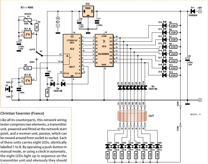
transmitter unit and obviously they should do the same on the receiver unit. In this way, just by watching the LED lighting cycle on the receiver unit, you can immediately spot any crossed wires, as well as any open circuits (the relevant LED never lights up) or shorts (two or more LEDs light at the same time).
