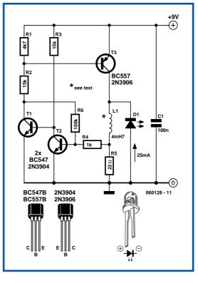
ghost. As soon as the current through R.5 increases about to 25 mA, T2 will conduct, T1 will block and T3 will also block. The current cannot flow through T3 any more and will look for another path, in this case through LED D1, which will now light up. By placing D1 in this position it acts in fact as a free-wheeling diode, which is good for the efficiency.
