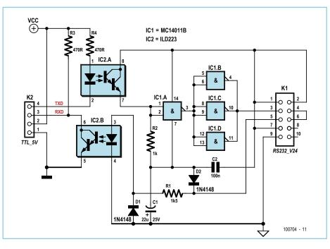
sheet the maximum permitted is 6 V. When a transmission originates on the TTLlevel side, the receiver transistor in the optocoupler drives a buffer implemented here using four NAND gates. Each gate is wired as an inverter, and it is easy to see from the circuit how overall inversion of the signal is avoided. Three of the gates are wired in parallel to increase the available output drive.
