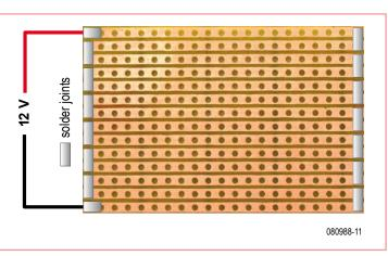
alternate soldered ends so that all the strips are connected in series. The two connections to the plate are made at the end of the strips as shown in the picture.
