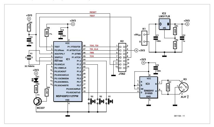
author built a small stand-alone DMX transmitter that can easily be configured using three buttons.
