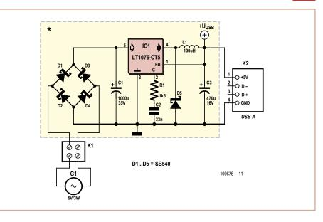
ering or charging mobile devices using their USB connector. Smoothing capacitor C1 is charged up to the peak value of the alternating voltage delivered by the dynamo; for most hub dynamos the typical peak output voltage is in excess of 10 V. Under load the typical voltage is of course lower, but still enough for the LT1076-CT5 as long as Schottky diodes are used and C1 has a value of at least  $1000 \,\mu$ F.
