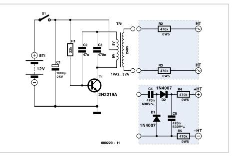
As the circuit diagram shows, the project is extremely simple, as it contains only a
