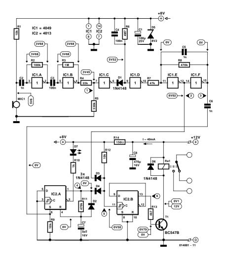
LED D1 is connected to the  $\overline{Q}$  output of IC2a and will indicate the time slot available for the two successive claps.
