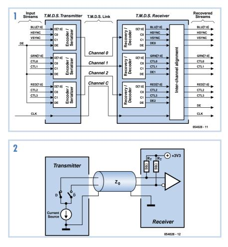
acquire a monitor or playback equipment you have to check both types of equipment to see whether they use a doublelink interface (six data channels) or a single-link interface (three data channels). The DVI 1.0 standard supports several different resolutions. They are listed in **Table 2**. Each resolution can also be
