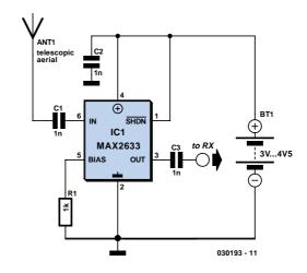
ure and low supply current makes it ideal for RF receive, buffer and transmit applications. The MAX2633 is biased internally and has a user-selectable supply current, which can be adjusted by adding a single external resistor (here, R1). This circuit draws only 3 mA current.
