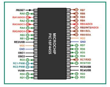
Figure 2. This diagram of the PIC18F4455 is purposely simplified, showing only the actually used functions of the pins of the PIC. D stands for 'Digital I/O' and A for 'Analogue input'.
