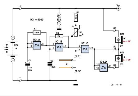
CMOS logic chip, which contains four 2-input Schmitt trigger NAND gates.
