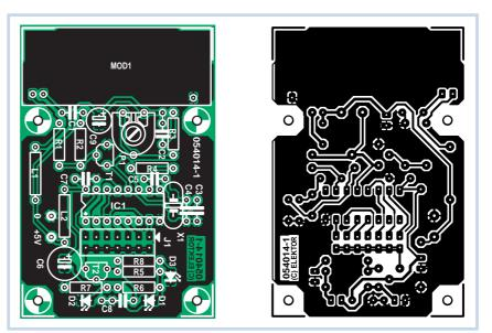
which means that battery operation is not suitable (unless a hefty electrolytic capacitor is connected across the supply terminals). L1 and L2 ensure that the supply voltage for the receiver module is as clean as possible. The quiescent current consumption is approximately 1.3 mA, and it increases to around 8 mA on average with a good received signal level.
