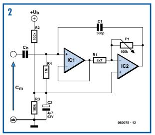
may not be too large. Otherwise, the AC voltage across  $C_m$  will cause clipping at the output of the second opamp. At maximum  $C_m$ , the gain of A2 is about 20 times. The peak-to-peak value of the input voltage may therefore not be more than about 1/20 of the power supply voltage. The circuit will always work well for smaller signals, provided the frequency is not too high.
