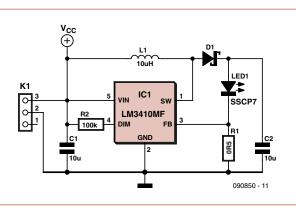
Power dissipation in the shunt resistor is therefore low. Using the desired value of LED current the value and power dissipation of the shunt resistor is given by:
