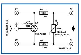
suddenly becomes a full conductor to the point of being able to absorb colossal currents without being destroyed. The one we are using here, whose size is of the same magnitude as an ordinary one watt resistor, can absorb a standardized 5,000 amps pulse lasting 8/20 ms!
