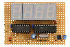
smaller QSO package with only 16 pins, can operate at 3.3 V, and has a shutdown mode with a current consumption of only 20  $\mu$ A. Inspired by this progress, the author resolved to design a digital thermometer circuit using this IC. Aside from the MAX6958, four common-cathode LED display modules (Toshiba TLR 324) and an Atmel AT89C2051 micro-
