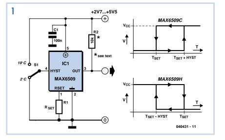
the temperature drops below the set point. The IC is housed in a SOT232 SMD package (**Figure 3**). The MAX6509 operates over a supply voltage range of +2.7-5.5 V with a supply current of only approximately 40 µA. The resulting self-heating is thus small enough to avoid corrupted temperature measurements (as long as the output transistor is not required to switch high currents to ground). The table lists suitable values of resistor R<sub>SET</sub> for various threshold temperatures.
