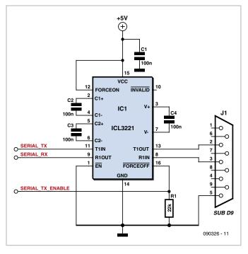
ber of RS232 modules in a project, as each requires a serial interface at the master. A hardware solution in the form of an RS232 multiplexer would be a solution but wouldn't it be nice to get this functionality for free!
