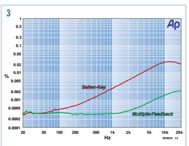
an input signal of 5 V<sub>rms</sub>. Standard polyester (MKT) capacitors were used in the circuits. To make the ultimate result more distinct, we intentionally used a simple opamp (TLO81) and avoided using expensive polypropylene, polystyrene or silver-mica capacitors.
