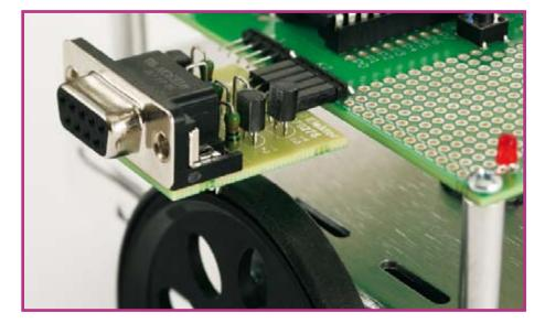
We have designed a small PCB for this circuit, but of course it's no problem to build it on piece of perforated prototyping board instead. With a bit of effort, you can probably even make it so compact that the entire circuit fits in a plug housing for a 9-way RS232 connector.
