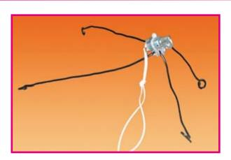
aligned to the longitudinal axis of the long front legs. In other words, the direction of vibration of the eccentric weight is toward the short legs. When the motor is switched on, the eccentric weight causes the robot to start vibrating, with the result that it moves forward. This robot can be built quickly with all sorts of bits and pieces from your junk box, and kids just love it.
