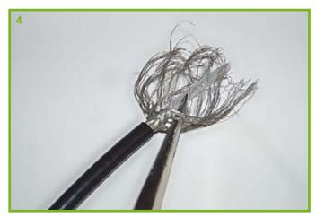
Using the pointed tool, carefully unweave the braid strands.
