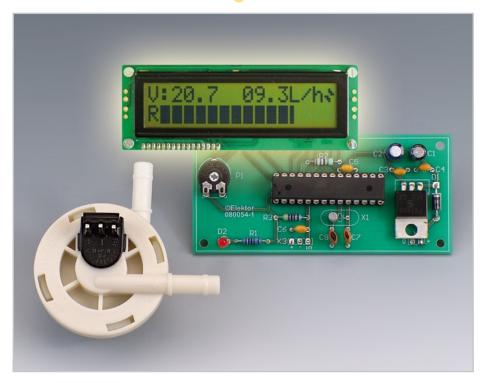
Now let's move on to the more interesting bit, which is the electronics of the virtual fuel gauge proper. flow sensor. This is an FHKSC 932-8501 from Digmesa [1] & [2]. This detector can measure fluid flows from 0.03 to 2.0 l/min, equivalent to a range of 1.8 to 120 l/hr — more than sufficient for the application envis-
