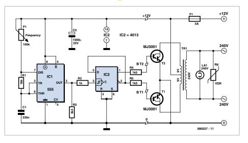
Note that, even though the circuit is intended and designed for powering by a car battery, i.e. from 12 V, the transformer is specified with a 9 V primary. But at full power you need to allow for a voltage drop of around 3 V between the collector and emitter of the power transistors. This relatively high saturation voltage is in fact a 'shortcoming' common to all devices in Darlington configuration, which actually consists of two transistors in one case.
