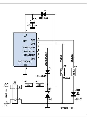
Cross() routine. As soon as this arrives the time information is updated in Realtime(), which also sends part of the IrDA data every 100 ms. Only a small part of the data is sent to the IR-diode each time to prevent C1 from being discharged too much (relatively large current through the LED).
