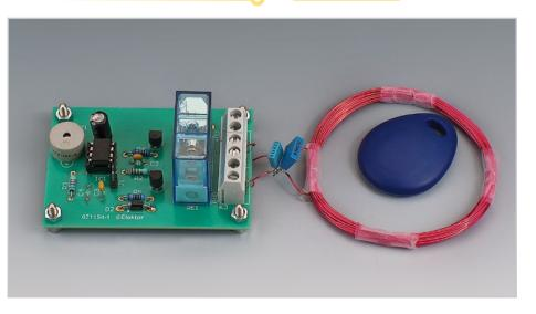
Each line is terminated by a 'CR' and an 'LF'. The first line gives the count of stored tag ID codes. There follow the individual ID codes, starting with the master tag. Each ID code consists of ten hexadecimal digits, making a total of 40 bits. The data transfer format is 9600 baud, 8 data bits, no parity and one stop bit. If a piezo buzzer has been connected to pin 2 it will emit a strange sound during any serial activity.
