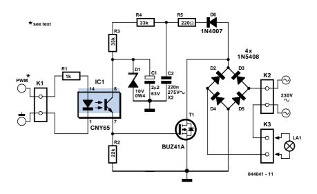
from the PWM signal only. When the voltage across T1 reduces, the voltage across D1 remains equal to 10 V up to a duty cycle of 88 %. A higher duty cycle results in a lower voltage. At 94 % the voltage of 4.8 V proved to be just enough to cause T1 to conduct sufficiently. This value may be considered the maximum duty cycle. At this value the transistor is just about 100 % in conduction. At 230 V mains voltage, the voltage across the lamp is only 2.5 V lower, measured with a 100-W lamp.
