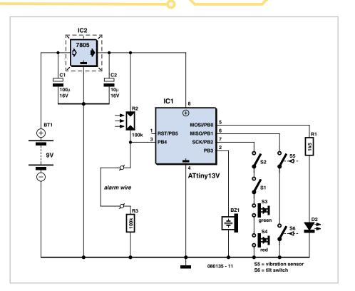
The arrangement and labelling of these buttons and switches is described below. On the left of the device lies switch S1 with the (deliberately misleading) legend 'Power on/off'. Of course, this does not turn the alarm on and off. On the right of the device is switch S2 with the legend 'Speaker on/off', which, naturally, does nothing of the sort. As you have probably already guessed, the red and green buttons also have nothing to do with arming or disarming the alarm.
