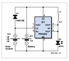
At night the energy stored in the battery is released into the LED. In contrast to similar designs, here we can make do with a single 1.2 V cell.
