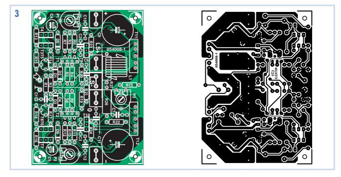
always stay below the maximum value (also take into account any possible mains voltage variations). If you do need to reduce the voltage, that should be done by **lowering** the value of R15 (R18). This causes the voltage across R14 (R17) to increase and hence the voltage across the JFET will drop.
