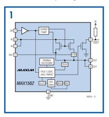
typically 40  $\mu$ A or 3  $\mu$ A in standby mode. The circuit introduces a very low resistance in the power line (typically 26 m $\Omega$  but guaranteed less than 50 m $\Omega$ ) from an internal MOSFET. The FET gate bias voltage is generated on-chip from a charge pump circuit.
