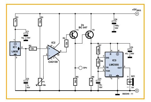
piezoelectric buzzer Bz1 to raise a loud alert. Components R7, R8 and C4 determine the on/off rhythm of the sounder. A transistor based relay driver may be driven off the emitter of T1 (TP1). Similarly, replacing the piezo sounder with a suitable relay allows switching of high-power flashers, sirens or horns working on the AC mains supply.
