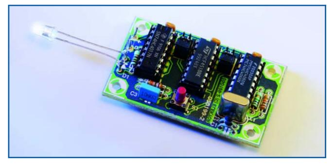
This little aid was originally designed to test the Shutter Time Meter from the January 2006 issue. This meter was specifically designed for 'analogue' SLR cameras.
