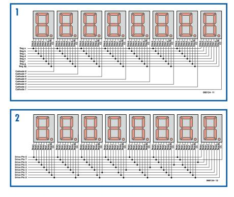
to flow. This current has to flow via a segment (the leftmost one in this case) but that segment is connected in the reverse direction! Display 1 remains dark therefore and the same applies to the other six displays.
