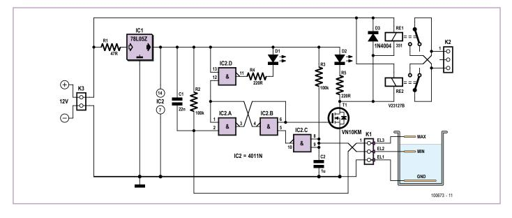
shown in the circuit diagram, corresponding to two positions for relays on the printed circuit board with different pin configurations. Only one of the two possibilities is fitted. The three electrodes are made from solid connerwire with a croce cortion of 1.5 mm to
