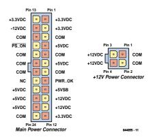
ity as with ATX motherboards (only -5 V has been omitted!). The extra 4 pins are for more 3.3-V, 5-V and 12-V connections (refer figure). In addition, there has to be a separate 4-way connecter ('+12 V power connector') that's intended to power the CPU only.
