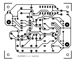
necessary is stored in two relatively large capacitors (C2 and C3) and these are charged through resistors R1 and R6 respectively. The disadvantage is that the circuit needs approximately 0.5 minute between switchovers to ensure these capacitors have sufficient charge. The current consumption of the entire circuit however is reduced to just a few milliamps.
