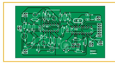
Figure 4. Component layout of the binaural sensor PCB. The PCB files can be downloaded from (3).
