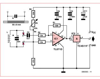
nals. The value of the capacitor (22 nF) has 5.3 kHz, but this can of course be adapted for been selected for use at a frequency of about use at different frequencies. The received
