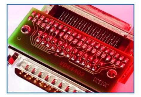
the PC have a female connector. The new cable that you bought cannot be used and you will have to look for another solution. One of these is to make an adaptor, which allows the USB/SCSI converter to be connected directly to the scanner. For the scanner we assumed a 25-way sub-D and for the converter a high-density connector. The schematic shows the necessary connections and their names. We don't discuss this any further, there is plenty of information available on the Internet.
