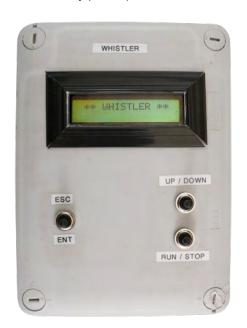
This device makes it possible to generate beeps at chosen regular time intervals for timing track race training. Each time interval is indicated by a beep, and the end of a performance test is indicated by a double beep. Two types of test are allowed:
