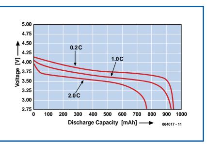
output voltage must be measured under load conditions to obtain a satisfactory result. Moreover, the value of the load must be known. Also, the battery must be under load for at least a minute.
