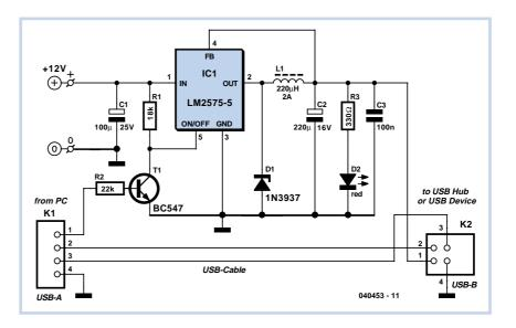
fast-recovery diode. Its principle is that internal power transistor switch on and off according to a feedback signal. This chopped or switched voltage is converted to DC with a small amount of ripple by D1, L1 and C2.
