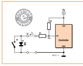
Klaus Jürgen Thiesler's '2-Wire Interface' was published in Elektor magazine in the form of both basic [1] and low-current [2] versions. Each variant used two transistors and a handful of other components to hook up an LED and a pushbutton to a microcontroller. The author still felt driven to simplify this arrangement further and can now provide a solution that, with only two resistors and a single I/O pin, could hardly be minimalized any more. Unless you know better!
