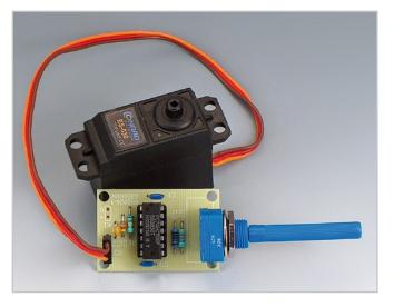
of IC1B, which repeats every 20 ms and the duration of which can be adjusted with P1. From experimenting with this circuit and an S3003 servo from Futaba it was observed
