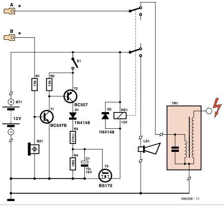
ably a miniature type or its electrical equivalent. To deactivate the alarm, the hidden switch should be flipped to the 'off' position to disable the movement sensor and the siren
