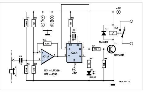
gear. The monostable will time out 2 s after m being triggered, the delay being deter-
