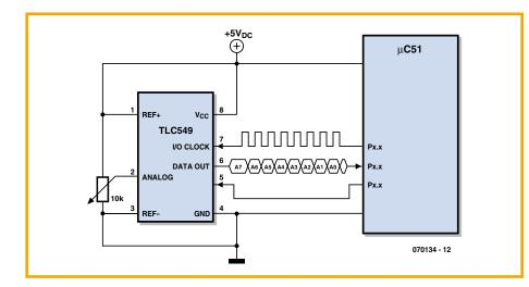
data from the TLC549 and returns the value addat is given below. Tests with an AT89S8252 Controller-Board (the Elektor Electronics December 2005 Flash Micro Board) indicated that the \_wait() can be omitted because the controller runs slowly
