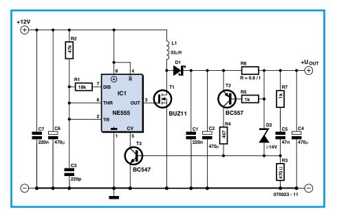
C5 and R7 provide a soft-start effect. The value of R1 can range from 22 k $\Omega$  for an output voltage of 15 V to 10 k $\Omega$  for an output voltage of 40 V.
