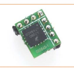
Figure 2. The sensor chip on the adapter PCB.
