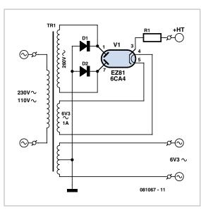
tre-tapped HT winding on the power transformer but this has a number of drawbacks for an adequately rated core size including increased voltage stress, small wire size and a poor utilization of the available winding window.
