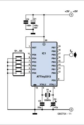
ter0 is used as an additional prescaler (division factor: 10) between the prescaled system clock and Timer/Counter1. The latter is set in the counter mode and now counts pulses at the Timer/Counter0 output pin OC0A (PB2); hence, the OC0A pin (PB2) and the external input pin T1 (PD5) are interconnected. The output frequency can be calculated as:
