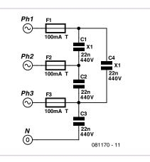
cuit involves just four capacitors which form a high-frequency bridge between the phases.
