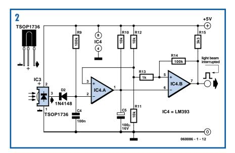
are included to prevent chatter of the output around the trigger point, although there is not really a risk of that happening in this circuit. Together with R14, the output of IC4b delivers a clean logic signal that we can use for further processing.
