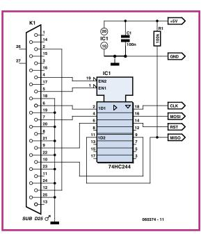
nothing more than one buffer IC type 74HC244, one 25-pin male sub-D connector for hooking up to the parallel printer port ('Centronics') on the PC, a 100 k $\Omega$  pull-up resistor on the MISO line and a .1 µF decoupling capacitor on the +5 V supply rail.
