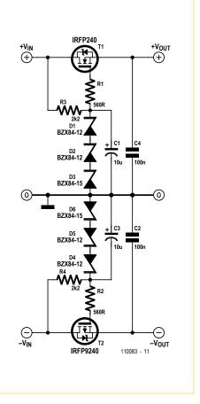
the heatsink already present in the amplifier; otherwise, a separate heatsink will be required. A thermal rating of 2.5 K/W will be suitable.
