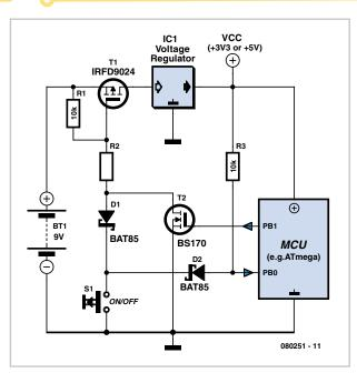
Now the microcontroller must poll the state of the pushbutton on its input port (PB0) at regular intervals. Immediately after switch-on it will detect that the button is pressed (a low level on the input port pin), and it must wait for the button
