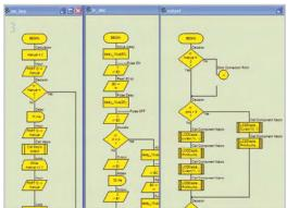
eight bits of PORTD individually, switching on or off any AC or DC devices by way of an 8way relay board or similar. The Standby key is used to switch all eight outputs on and off. There are also eight push-to-make switches to manually toggle the state of any output. By pressing switch 1 and 2 at the same time you switch all outputs on or off. The state of the outputs is shown on the LC display. Bits 6 and 7 of PORTB are used to select the address mode of the output control; 00 =TV, 01 = VCR,
