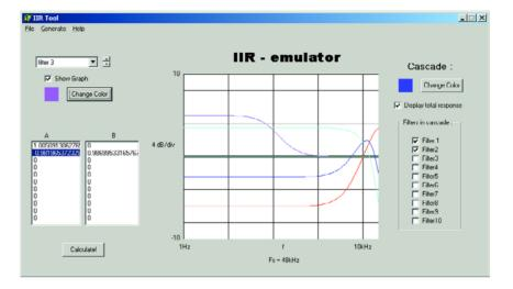
selected. The coefficients that are shown on the screen belong to this filter. To enter your own coefficients for this filter you only need to click the desired coefficient after which you can type in the new value. For example, try changing  $a_1$  (the second value at the top of the column near a) from 0 to 0.5. Immediately after this change you will note that the graph of the frequency characteristic has changed.
