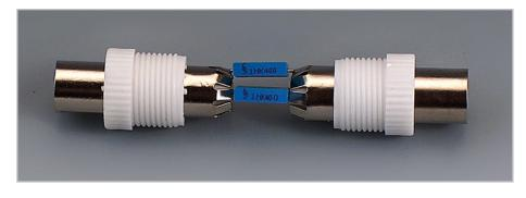
This often creates a problem when earth loops are created in the shielding of the video cables, which may cause hum and other interference. The surround-sound receiver contains a tuner that takes its signal from a central aerial distribution system. The TV is also connected to this and
