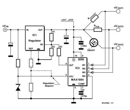
current as necessary to ground to force the regulator to raise its output voltage to bring the lowest of the MAX1804 inputs to four times the voltage on the ADJ pin. The voltage on ADJ can be provided by a reference voltage generated by the regulator, or, if this is not available, by an external voltage reference or Zener diode. The available control range can be set via R3: in the limit, R3 is effectively in par-
