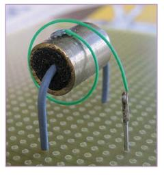
copper cylinder. This is the second contact. The foam resistance is pressure dependent. Consequently, when the device moves due to an external force, the inertia of the cylinder causes varying pressure in the foam, resulting in a small change of resistance between the inner conductor and the cylinder. Because of that, it's important to ensure the cylinder vibration is not
