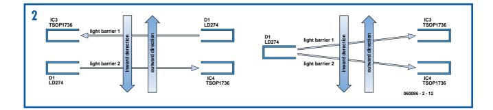
IR-transmitters is a better solution. This circuit has a range of several meters, even if the sun shines directly on the receiver!
