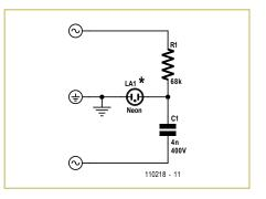
into a power socket; the author used a small transparent cover to protect the neon.
