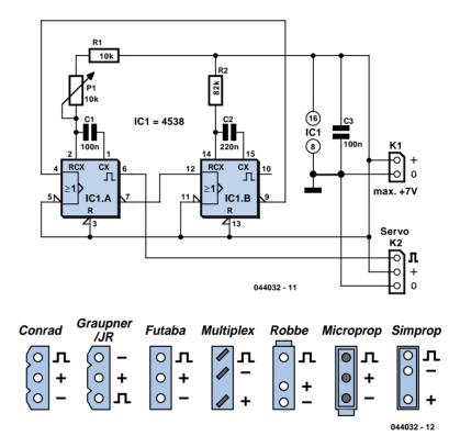
At the end of this pulse inverting output  $\overline{Q}$  generates a rising edge. This edge triggers IC1.B, which then generates a pulse. The pulse-width here is 82 k × 220 n  $\approx$  18 ms. At the end of this pulse the  $\overline{Q}$  output will also generate a rising edge. This in turn makes IC1.A generate a pulse again. This completes the circle.
