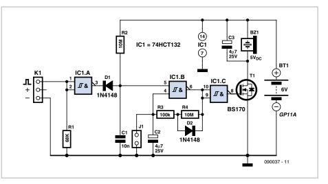
MOSFET transistor T1. All the time that the RC receiver output is delivering positive pulses, the oscillator is blocked by IC1.A and diode D1. Setting jumper J1 parallel to C2 also disables the oscillator and serves to 'disarm' the distress beacon.
