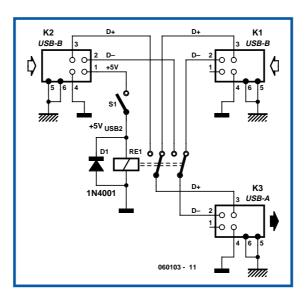
nected to K2, so the USB signal to the printer comes from the PC via K1, the normally closed contacts of relay Re1, through to K3 and from there to the printer. Whenever the laptop is connected up, the presence of the 5volt power signal on its USB port causes Re1 to switch over to the printer's connection to K2 and the laptop. Unplugging the laptop returns control of the printer back to there PC.
