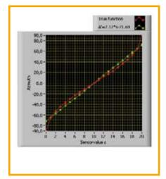
Figure 5. Resolution of the sound source bearing is a function of its azimuth. The average value is approximately 9°.
