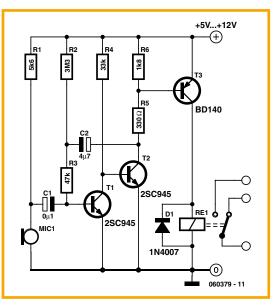
capacitor C2. Allow a few seconds for the relay to be switched off. You can increase or decrease the 'on' period by changing the value of C2. A higher value results in a longer 'on' period, and vice versa. Do not use a value greater than 47  $\mu$ F.
