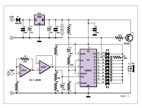
out! D1 protects the circuit against reverse polarity.
