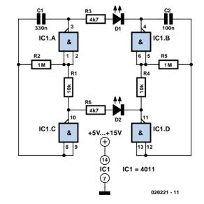
4011 can be operated over a supply voltage range of 5–15 V. Higher currents can be provided by the HC family (supply voltage 3–6 V) or the HCT family (5 V). Incidentally, the part number of the quad gate IC in the HC family is HC7400.
