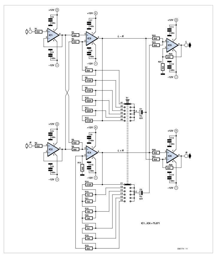
channel is slightly shifted in phase. To make the stereo image 'wider', you can amplify the difference signals of both channels.
