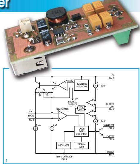
in the circuit board for this purpose. As we haven't been able to invent a device that produces more energy than it consumes, you should bear in mind that the input current of the circuit is higher than the output current. As a general rule, you can assume that the input current is equal to the product of the output current and the output voltage divided by the input
