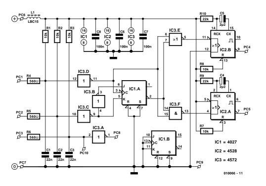
winding the volume up to the maximum or down to the minimum. This is clearly not desirable: to rectify the situation we use a monostable to deliver a brief negative-going pulse. The pulse width is determined by R9-C4 and R10-C5.
