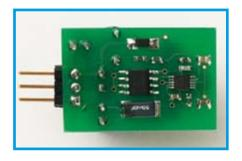
pin form factor makes it a simple replacement for conventional three-terminal voltage regulator ICs. The buck-boost switching circuit uses an SMD power FET for T2, and to achieve high efficiency (approximately 90 %) a Schottky switching diode for D1. The most specialised component is the miniature transformer designed for use in this type of supply. For the prototype we used a Coiltronics CTX50-4.
