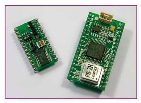
Photo 3. The PicBasic (right) marked Comfile Technology's entry into the world of these special microcontrollers. It wasn't yet pin-compatible with the Basic Stamp 2 (left).
