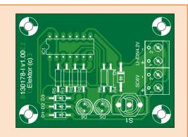
Connectors marked SC6V and LI-ION4.2V = PCB terminal block, lead pitch 5mm
