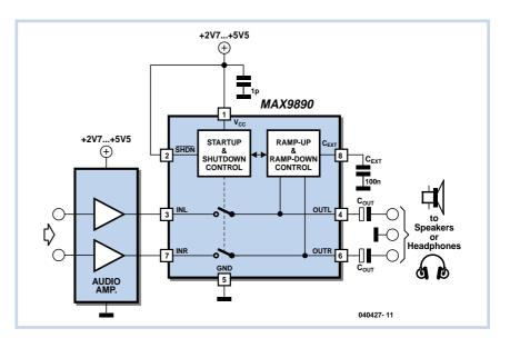
sion being preferred for capacitors up to 220 μF. With coupling capacitor values larger than this, switch-on noises may still be audible under certain conditions.
