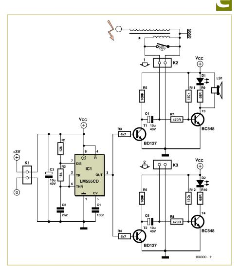
breaker is open the amplified pulses will turn on T3 and T4 respectively, so that the relevant LEDs turn on and the buzzer will sound.
