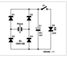
is relatively small and the crystal is effectively a capacitor with a capacitance of only around 20 nF to 50 nF. This means that we need larger-scale storage in the form of an electrolytic capacitor.
