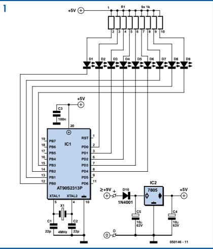
the array of 1 k $\Omega$  resistors: this is enough for the low-current LEDs, which are used in order to ensure a long battery life. A 5 V fixed voltage regulator (IC2) and decoupling and smoothing capacitors C3 to C5 round off the circuit. Diode D10 prevents damage should the 9 V PP3 (6F22) type battery be accidentally connected the wrong way around.
