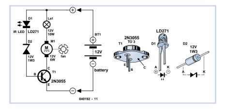
Don't try to replace the LED by two 1N4001 diodes or the like, replace the ZPY12 by a ZPY13, or fit a series resistor for the LED. That would make the 'on' region too large.
