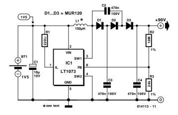
voltage of 90 V will be obtained. The output of the circuit can deliver a few milliamps of current.
