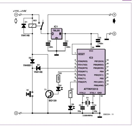
the author's case) will shortly be turned off. Pressing button T1 (start/stop) now restarts the counter and extends the on time for a further period. As before the timer can be terminated at any other time by a press of T1.
