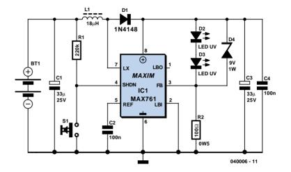
and 50  $\mu$ H. It stores current in its magnetic field while the MOSFET inside the MAX761 is switched. A toroid inductor is preferred in this position as it will guarantee low stray radiation. D1 has to be a relatively fast diode so don't be tempted to use an 1N400x because it has a too slow recovery time.
