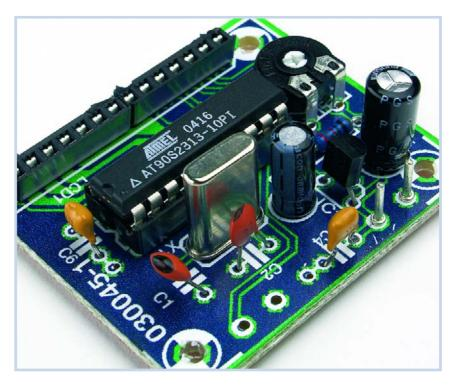
quency from above the timer 0 overflow occurs at a frequency of 32 Hz. The measurement timing window is closed when 32 interrupts have been counted and the frequency of the input signal is calculated and displayed. The interrupt rate restricts the maximum input to 1.5 MHz and at this frequency the display will exhibit a jitter of 4 Hz i.e. the displayed frequency will 'wander' by 4 Hz. All input frequencies below 200 kHz should not display any jitter.
