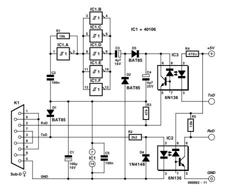
supply voltage. A voltage of around + 9 V is thus available from C4, which is connected to the collector of optocoupler IC3. In principle, the voltage level at an RS232 interface should be + 12 V to + 15 V, but PCs can generally work with significantly lower voltages. Notebook computers in particular sometimes have a voltage of only + 8 V.
