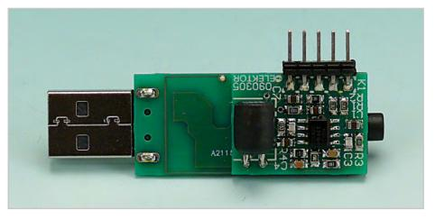
of the FM transmitter board also played a part here. To make it easier to connect this circuit to the transmitter board, a connector was included on this board. The supply voltage and audio signals are carried via this connector. The board has been designed in such a as aerial and connected to the transmitter board (it just so happens there is a via next to C4).
