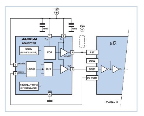
tor is more accurate, with an error of only 1% at 5 V and 25 °C, although this is still a bit too much for time measurements. The error can be as much as  $\pm 3\%$  over the
