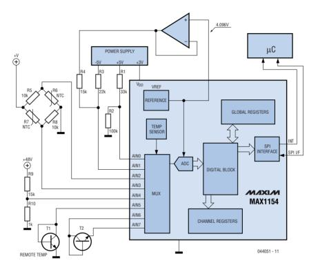
2 internal voltages. These 8 external voltages can also be programmed for temperature sensors, where an external diode can be used as a simple and cheap sensor.
