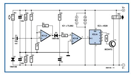
ply voltage for the circuit is also taken from the motherboard via this connector. Components C3, C4, R8 and R9 create an artificial ground potential at half the supply voltage (6 V), which serves as a reference voltage for the opamp. Diode D1 should have the lowest possible voltage drop to minimise the voltage loss to the fan.
