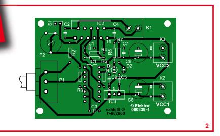
the chip temperature is 145 degrees. The IC is automatically shut down when 170 degrees C is reached. Pin 8 of the LMD18200 is the current sense input. R6 connects this pin to ground. The Brake input (pin 4) is hard wired to ground. C2 and C4 at the motor output are 'bootstrap' capacitors. Pins 2 and 10 are the H-Bridge outputs powering the DC motor.
