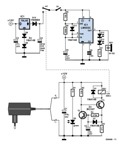
as long as possible. Resistors R5 and R6 define a short 'on' time of just 10 ms. That is, however, sufficient to get a loud warning from the active buzzer. In case the pulses are too short, increase the value of R5 (at the expense of a higher average current drawn from the Goldcap).
