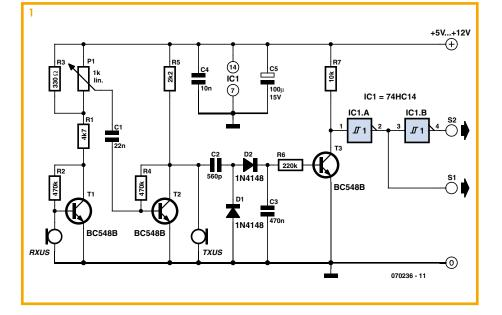
amplifier using transistors T1 and T2. As the gain of this stage is very high, it can be reduced if necessary by pot P1 to avoid its going into oscillation all on its own, even in the absence of an obstacle. The output of this amplifier is connected to the ultrasonic emitter TXUS, therby forming the loop that is liable to oscillate due to the effect of feedback.
