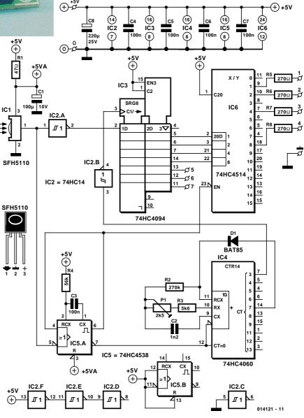
never be more than one active output. In case of the 'Switchbox for Loudspeakers', when several amplifiers are connected to a loudspeaker, there can never be a short circuit, or conversely, an overload of the amplifier. For this reason the 'inhibit' is also connected to the output of IC5a, stopping any transient pulses from appearing at the outputs during the clocking in of the data and giving time for the relay contacts to release before another relay is activated (break-beforemake).
