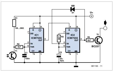
light output (they are often driven by a multiplex signal) producing a more stable DC voltage to inputs 2 and 6 of IC1. The circuit is battery powered so the CMOS version of the familiar 555 timer is used for IC1 and IC2. The output of IC1 (pin 3) keeps IC2 reset (pin 4) held Low while there is no light falling on T1. When the wash cycle is finished the LED lights, causing T1 to conduct and the voltage
