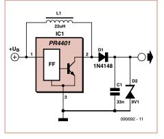
However, this is only half the story. Even when there is no load at the output the IC still draws current, and so the battery will eventually run flat even if the equipment is switched off. This means that some kind of automatic shutdown circuit is needed. How can we make a
