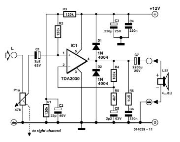
the amplifier in the high frequency range. The load is connected via the output electrolytic capacitor C7. In the data sheet, you can see which parameters change if you 'play around' with the values of the resistors and capacitors. Any individual speaker with an impedance of 4 to 8  $\Omega$  or a multi-way loudspeaker can be connected to the output. The maximum achievable power is 6 to 12 W, so a heat sink with a thermal resistance of 8.3 K/W to 4.2 K/W is mandatory.
