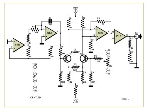
The third opamp (IC1.C) is configured as a difference amplifier, which presents the sine wave at its output. This signal is then buffered
