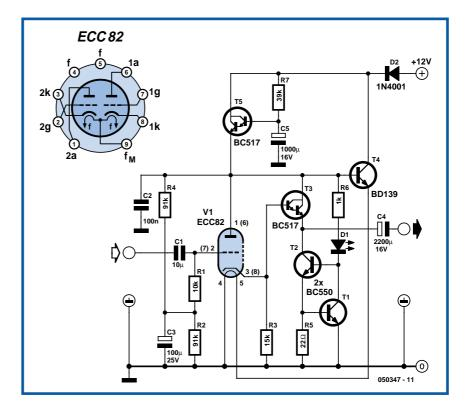
equivalent: 12AU7). This device, as opposed to a transistor configuration, enables the output stage to be driven with a constant value, low impedance. In other words, the signal from the low impedance point is used to drive the high impedance of the output stage, a situation which promotes low overall THD.
