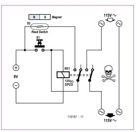
main entrance door, and a matching magnet is attached to the door itself such that when the door is closed the reed contact is also closed. To enable power to the house, press S1 briefly. Relay RE1 will pull in and complete the circuit for all the AC powered appliances in the house. The relay will be held in even after the button is released via the second relay contact and the reed contact ('latching' function).
