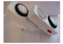
tial to keep the 'on' time of the second timer shorter than that of the first timer. If a maximum cycle time of 48 days is too short, you can also connect a third timer. With three timers, the maximum cycle time is 2304 days (one 'on' time in approximately 6.5 years).
