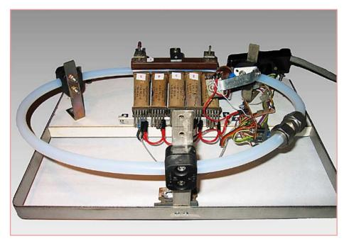
All of the coils used in the author's device (heavy-duty relay coils) have a resistance of 12  $\Omega$  and operate from a 12 V DC supply voltage. The indicator LEDs have 270- $\Omega$  series resistors and operate from 5 V. They light up when the associated coils are energized.
