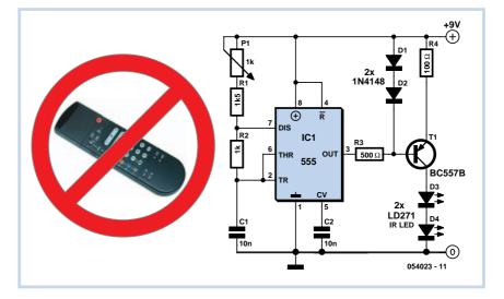
longer 'sees' the remote control! The oscillator is built around a standard NE555. This drives a buffer stage, which provides the current to the two LEDs. Setting up this circuit is very easy. Point the IR LEDs towards the device that needs its remote control blocked. Then pick up
