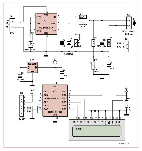
One last little detail: to allow more accurate setting of the output voltage, you can include a second 1 k $\Omega$  potentiometer in series with P1.
