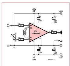
from mutual dependency of the measured and offset voltages and was therefore not suitable. The AD620 from Analog Devices, however, has been especially designed for this type of application and works well. In this opamp each of the input signals has its own opamp, so that they do not interfere with each other.
