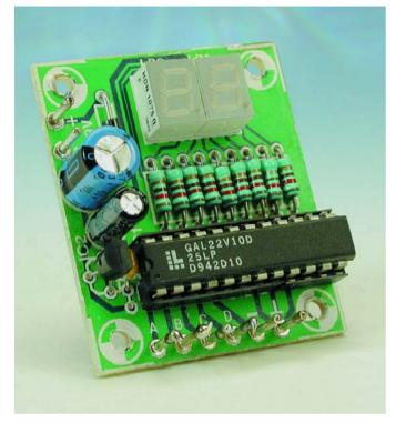
The circuit is provided with its own 5-V regulator (78L05, take note of the dissipation!) so finding a suitable power supply should not be problem. The current consumption is a minimum of about 60 mA (indication '-') to about 85 mA maximum (indication '10'). The jedec file you'll need to program the GAL may be obtained as a Free Download from the *Elek*-
