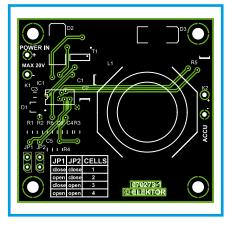
coil it may be necessary to let the soldering iron heat up a bit more first. The connecting leads are quite chunky and they require a fair amount of heat to raise them to the correct temperature.
