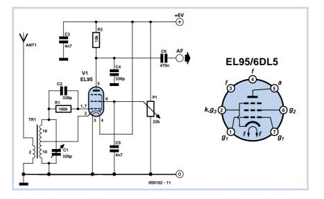
necessary, since the voltage level is sufficient for a direct connection to the Line input of a PC sound card. A screened cable should be used for this connection. A two-turn antenna coil is located at the bottom end of the tuned circuit. It provides very loose coupling to the antenna, which is important for good stability.
