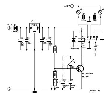
used. In one prototype model, the relay pulled in OK and energised R3 and P2, but it refused to do anything further. If your construction exhibits similar behaviour (and you are dependent on a particular type of relay), it may help to include capacitor C2 in the circuit (as shown in dashed outline) in order to slightly delay the effect of switching in P2 and R3.
