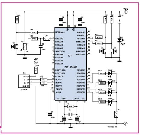
Figure 1. Schematic of the USB demo board.
