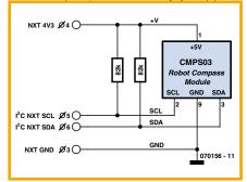
a ready-to-go compass module type CMPS03. Two mutually perpendicular Philips KMZ51 hall-sensors are used to detect the Earth's geomagnetic field. With a small PIC-controller a value between 0 and 360 degrees is calculated and made available in digital form at the output of the module. The communication with the outside world takes place via the I<sup>2</sup>C protocol or via a PWM output.
