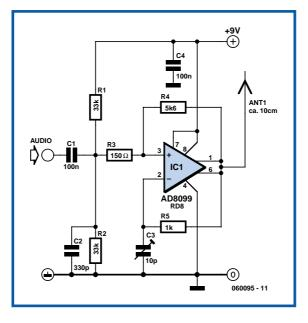
is continually being charged and discharged when the voltage reaches the hysteresis threshold. The output continually toggles as a consequence. This results in a square wave output voltage. With a 10-pF trimmer capacitor the frequency can be adjusted into the VHF FM broadcast band 88-108 MHz). The frequency of the oscillator is stable enough
