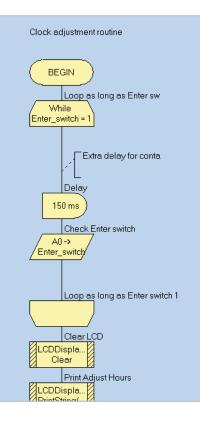
to set the minutes (in the same way as for the hours). After pressing Enter again, you are asked for a value for the light threshold. This value is compared with the amount of light falling on the LDR. When the value of the LDR becomes less than the threshold the lights come on.
