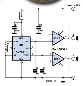
available at the accelerometer IC output information reflecting the acceleration registered — in analogue or digital
