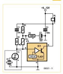
The circuit has a couple of handy features, firstly it works very well on the end of a twisted-pair — the output can be tapped off at the wiper if  $R_{\rm L}$  is a pot at the power supply end, secondly by salvaging the JFET from an old electret mic (some common types of JFET will work but not quite as well), just about
