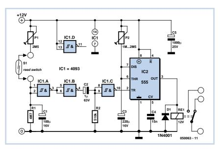
The time constant of P1 and C1 is set so that the fan does not run as a result of lavatorial transactions of a more minor nature, where the lid is opened and then closed shortly afterwards, before C1 has a chance to charge sufficiently to trigger the circuit.
