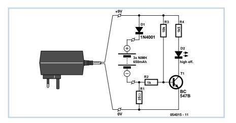
somewhat, but with a maintenance charge such as in this application it is not necessary to charge with an accurate constant current, provided that the current is not too high.
