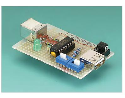
data lines and switching the MOSFET on. The PC now recognizes the USB device. Pressing S1 disconnects the device.
