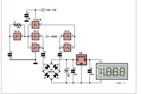
IC1 is a 40106 CMOS hex Schmitt inverter. Its first gate IC1.A is wired as an oscillator by way of R1 and C1, at a frequency of around 10 kHz. IC1.B inverts the signal, so that gates IC1.C / IC1.D and IC1.E / IC1.F can be driven in antiphase. The signal is output via C2 and C3, rectified by a diode bridge, filtered by C4 and C5, and stabilized by IC2 and C5 to a value of 8 V. The input supply voltage, decoupled by C7, is not very critical, somewhere between 10 and 15 V.
