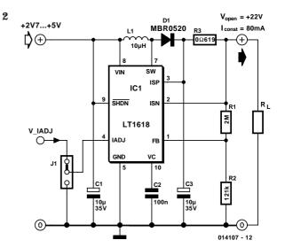
tor with a current limit mechanism. This makes it easy to protect an otherwise not short-circuit-proof switching reg-
