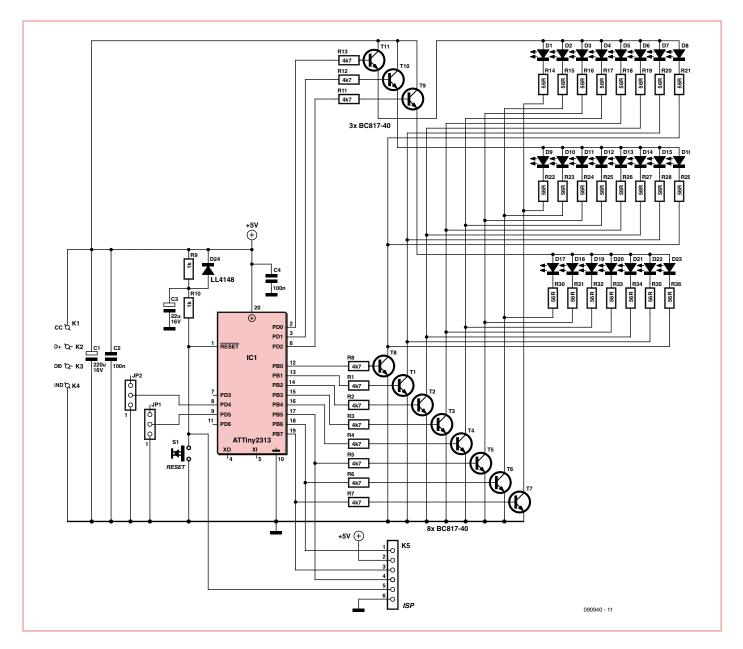
LO L296 orange LEDs from Osram, which have a viewing angle of 160°. A six-way connector is provided to allow in-system programming (ISP) of the microcontroller. The configuration fuses are set to enable use of the internal 4 MHz clock source, which is divided down to 0.5 MHz by an internal divider. If the fuses are not correctly programmed the light sequences will run too quickly, too slowly, or even not at all!
