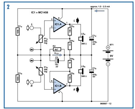
tendency to oscillate. It is possible to calculate suitable values for these components, but it is better to determine them by experiment. C2 must be sufficiently large
