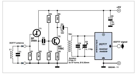
circuit. A bipolar transistor (T2) provides a gain of around 5 dB. The output signal is coupled to the antenna input of the DCF77 module via a transformer. The secondary of the transformer, in conjunction with capa-
