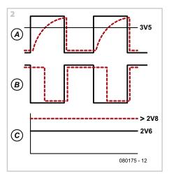
shown the signals at various points in **Fig-ure 2**. The dotted line represents the signal when the plate is touched, the solid line when it isn't touched.
