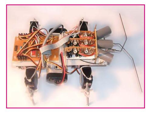
of 15 devices. For this reason, the three PIR sensors are connected to the robot in parallel with the ISP port via jumpers. In normal operation, the PIR sensors are connected to the robot. If a new program must be downloaded to the robot, the jumpers must be switched over to make the ISP port available.
