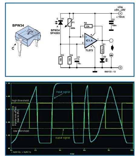
can 'see' the laser beam directly. The small hole should be filled with a black drinking straw so that only light from the direction of the laser beam can enter. With the appropriate setup of the box and the mirrors, the laser beam is so intense that even direct sunlight cannot affect the operation of the photodiode.
