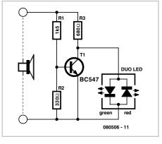
During the negative half cycle the red LED is driven via R3 and will turn on when the voltage is high enough. In the transition region (where T1 conducts more and more and 'throttles' the green LED as a result) the combination of red/green gives the orange
