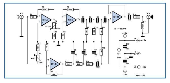
higher than that of IC1.C to ensure the overall response curve remains as flat as possible at equal settings of the tone controls. Because each network introduces a loss of about 1.72 (times), IC1.D and IC1.C first amplify the signal. The gain is set at about 8 (times) allowing input signal levels up to 1 V to pass the circuit at maximum gain and distortion-free. The gain also compensates the attenuation if you prefer to keep the tone controls at the
