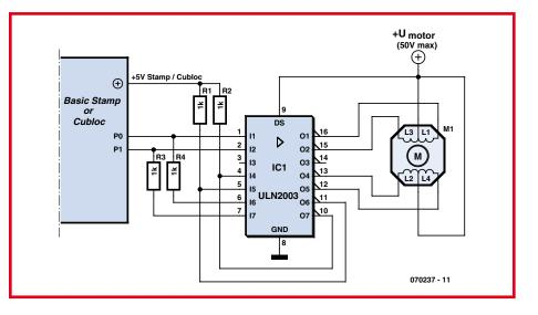
per motor: single-pole and double-pole. The former are simpler to drive, as all you have to do is apply voltage or not to their windings, while in 2-pole motors, the voltage applied to these windings has to be regularly inverted, slightly complicating the circuitry that's required.
