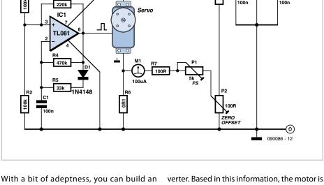
electronic scales based on a servo motor. Depending on the type of servo you use, it can measure weights of up to around 10 pounds (just under 5 kilograms) with reasonable accuracy.
