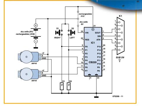
5 V regulator. However, if you are going to use NiMH rechargeables instead of primary cells, you'll have to use the VDD input to power the Cubloc, as in this case the voltage available is only 4.8 V.
