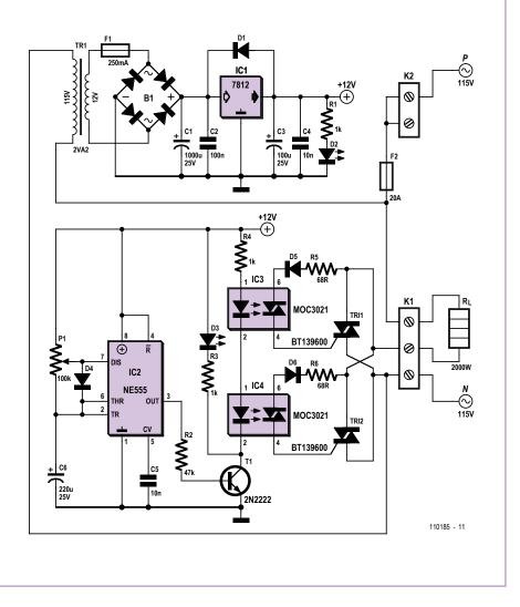
By way of transistor T1, IC2 drives two MOC3021 phototriacs (IC3 & IC4) which provide the isolation between the circuit's 'driver' section and the 'power' section, which is directly connected to the AC powerlines. Each phototriac drives a power triac (TRI1 & TRI2). These two triacs are fitted in parallel and share the task of supplying the convector ( $R_L$ ): one triac supplies the positive half-cycle while the other triac supplies the negative
