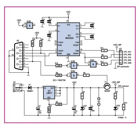
Figure 2. Circuit of the LPC900 programmer.
