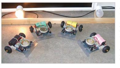
robot construction kit onto the market, the Asuro. This robot is available from Conrad Electronics [3], among others. The Asuro contains an Atmel ATmega processor with a builtin hex loader. You can write programs for the Asuro in C or (simpler) in Bascom [4]. Using an IR interface (with the supplied RS232 IR transceiver) the hex program can be sent to the Asuro. A USB IR transceiver is also available.
