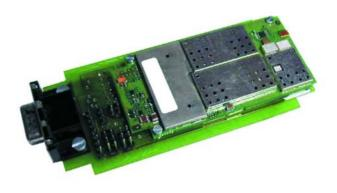
These modems can be used with a standard RS232 cable; just connect a power supply and antenna and you're ready to start experimenting! You do of course have to insert a valid SIM card into the GSM.
