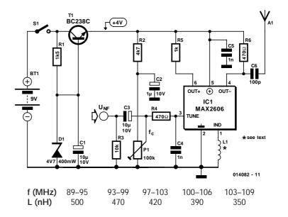
nected to each of the outputs for this purpose. You can use a capacitor to tap off the radio signal from either one of these resistors. Several milliwatts of power are available. At the audio input, a signal amplitude of 10 to 20 mV is enough to generate the standard VHF frequency deviation of  $\pm 40$  kHz.
