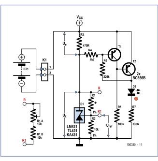
1.2 V cells). For example, if there are six cells in the battery, its nominal terminal voltage will be 7.2 V. A discharge threshold voltage of around 1 V per cell is appropriate, which means that for six cells the threshold is 6 V. We now need to set the voltage  $U_Z$  across the adjustable Zener diode D1 (an LM431) to about 0.5 V less than the threshold voltage at which we want LED D2 to light.
