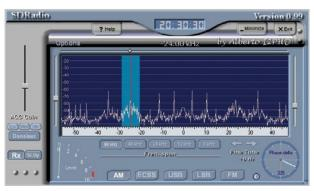
The SDRadio program by Alberto (http://digilander.libero.it/i2phd/ sdradio) is used as the decoder. The illustration shows an AM station being received. The sound card used (a USB Sound Blaster) has a sample rate of 96 kHz, giving a tuneable range of 48 kHz. In the illustration we can see three further transmissions.
