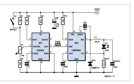
The U2352 can generate a PWM signal adjustable from 0 % to 100 % using a minimum of external components. The basic frequency of the internal triangle wave oscillator is set by C1 to around 10 kHz:
