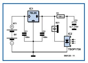
devices from other manufacturers can be used, and of course carrier frequencies other than 38 kHz can be used. The circuit still works if there is a mismatch between the nominal carrier frequencies of the transmitter and receiver IC, but range is reduced. It is still, however, adequate for determining whether a remote control is producing an IR signal or not.
