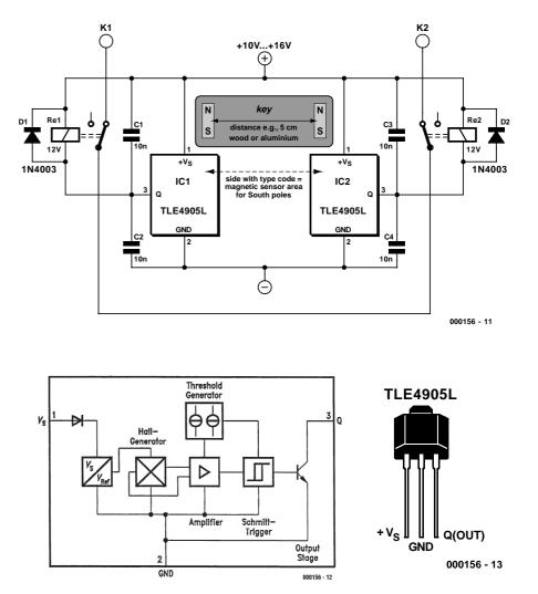
The two magnets should be glued in the same way round, which can easily be tested by checking that the poles repel. Alternatively, of course, the magnets can be fixed in a flat plastic box using hot-melt glue. Remember that only one side of the key will open the lock.
