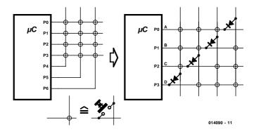
remaining port pins, which are configured as inputs. Thanks to the diodes, a voltage will be detected on only one of the inputs, depending on which key is pressed, and the software can assign the appropriate action to this event.
