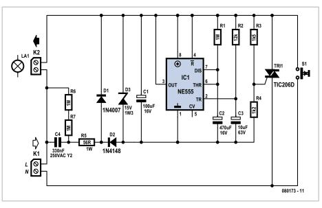
input. When the power supply is turned on, C3 holds the TR input of the 555 Low for a
