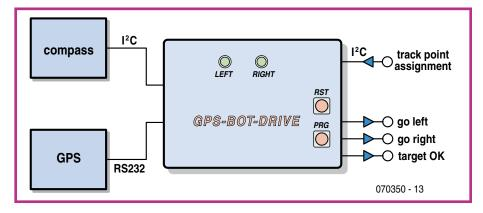
Figure 3. Simplified block diagram of the navigation system. The buttons are used when programming. Commands for the motors are output on two port pins.
