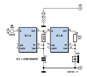
IC1.A is a slow oscillator which is enabled when reset pin 4 is taken High, and inhibited when it is taken Low. Output pin 5 of IC1.A pulses audio oscillator IC1.B, which is similarly enabled when reset pin 10 is taken High, and inhibited when it is taken Low.
