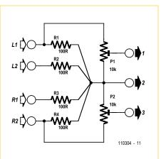
ter level is suitable for the input to a power amplifier. An appropriate trimmer setting can be found by ear, adjusting the volume of the rear speakers for the desired balance.
