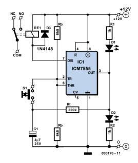
age. When the pushbutton is open-circuit, the input is clamped within this zone (at half the supply voltage) by two equalvalue resistors, Rb. To prevent the circuit powering-up into an unknown condition, a power-up reset may be applied with a resistor from supply to pin 4 and capacitor to ground.
