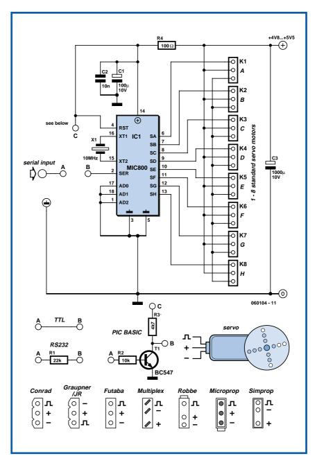
input signals in negative logic (a logic 1 corresponding to a Low level and vice versa). In the case of a direct TTL connection, and depending on the possibilities of the UART contained in the related microcontroller, it is sometimes impossible to generate such signals. Therefore, we must should an inverter transistor.
