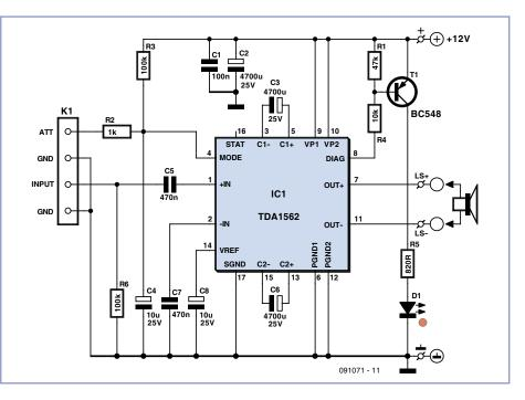
need it. This is a mute control that puts the circuit into stand-by when grounded. No output signal is produced and the consumption is reduced to a minimum.
