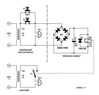
relay contacts. These contacts are the 'electronic' button for the second bell,
