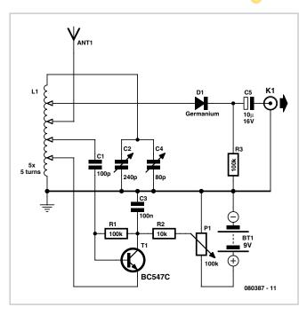
tune in to very weak stations. The tuning capacitor used has two gangs of vanes with capacitances of 240 pF and 80 pF. These two gangs are connected in parallel to make a 320 pF variable capacitance. The air-cored inductor has 25 turns on a diameter of 10 mm, with taps at 5-turn intervals. The resonant circuit so formed is capable of covering the full shortwave band from 5 MHz to 25 MHz.
