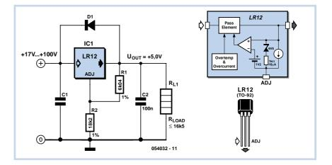
keep the LR12 stable. In cases where the voltage at the input may be smaller than at the output an extra protection diode is required, for example a 1N4004.
