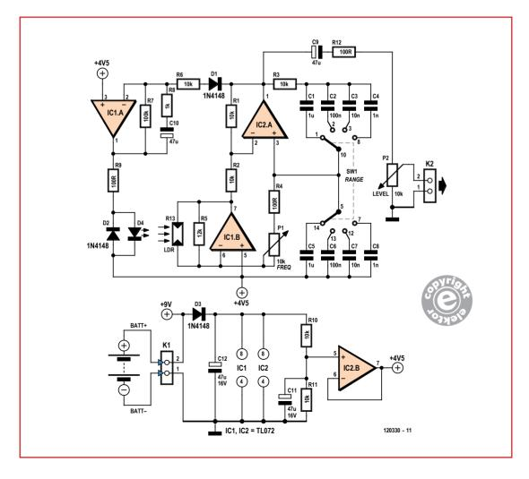
IC1A is an integrator that monitors the amplitude of the output signal and drives an LED (D2).
