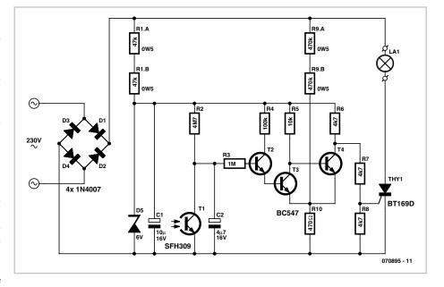
this will become high enough so that T2 and T3 will conduct. T4 will not receive any base current any more and blocks, so that the thyristor will receive continuous gate current via voltage divider R6/R7/R8 and the lamp will light up. R9 and R10 provide for some hysteresis in the switching behaviour of T2 and T3, so that the circuit does not repeatedly turn on and off when dusk falls.
