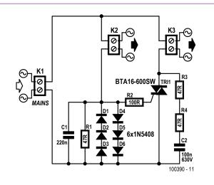
but this is strongly dependent on the characteristics of the triac and the waveform of the load current. If the current is not sinusoidal or R1 is too small, the triac will trigger later and may not be able to supply sufficient power to K3, in which case the circuit will act as a sort of dimmer.
