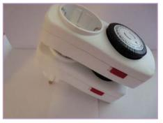
As you can see from the photos, the second timer may interfere with the tabs of the first timer if they are plugged together with one on top of the other. This can be avoided by turning the second timer by 180 degrees relative to the first one.
