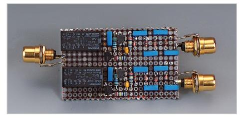
two devices with S/PDIF outputs to the receiver. When several devices are turned on that output a continuous S/PDIF signal, the required device needs to be momentarily turned off and then on again to select it. It is relatively easy to expand the circuit with more inputs.
