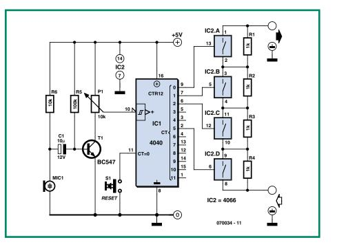
Switch S1 allows the counter to be reset, switching all 4066 switches to off, i.e., the
