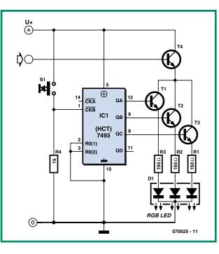
The type of transistor that is used for T1 to T3 is not very critical. Standard LEDs require relatively little current, about 20 mA. A BC337 will therefore work fine, as will a BC547.
