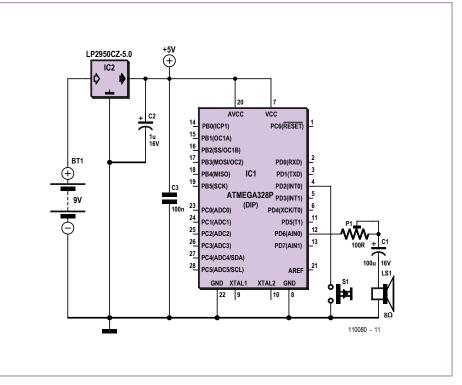
When power is applied the unit immediately plays the stored doorbell sound, and the AVR microcontroller then enters a low-power standby mode. Pressing the bell push button causes the microcontroller to leave standby mode and play the WAV file again.
