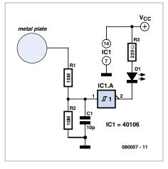
by input pin 1 of gate IC1.A. R1 has been added to prevent electrostatic discharge (ESD) energy from damaging the inverter gate input. ESD may occur when you have been charged with an amount of electro static energy by walking on a carpet with rubber soles. You can increase the sensitivity of the detector by experimenting with lower values fore R1 e.g. 1 k $\Omega$  and a smaller metal plate.
