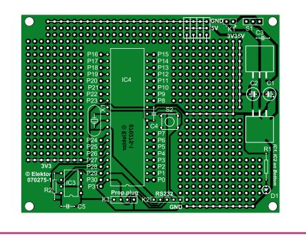
Figure 2: The board layout is single-sided. If you expect to use the prototyping area a lot then a double-sided through-hole plated version would be preferable.
