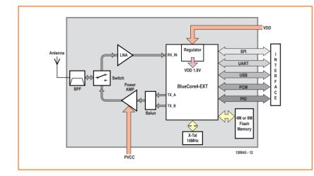
Figure 2. Block diagram of the BTM-222 Bluetooth module.
