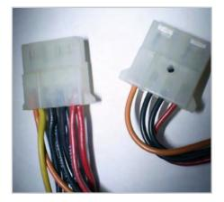
tact springs gently outwards and press each pin back into its right position. You will find the longer sizes of sleeve are easier to handle, also that the individual parts of the connectors move around more easily if you spray them first with contact lubricant.
