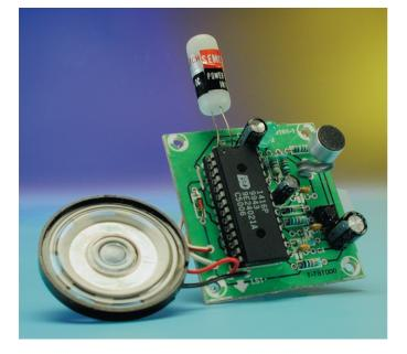
There are lots of exciting applications for a voice memory. The circuit presented here has been installed in the author's toilet in order to advise potential users of the facilities to do so sitting down rather than standing! A mercury tilt switch detects when the seat is lifted and activates the (remotely connected) voice memory: the admonitory text can be chosen at the whim of the householder.
