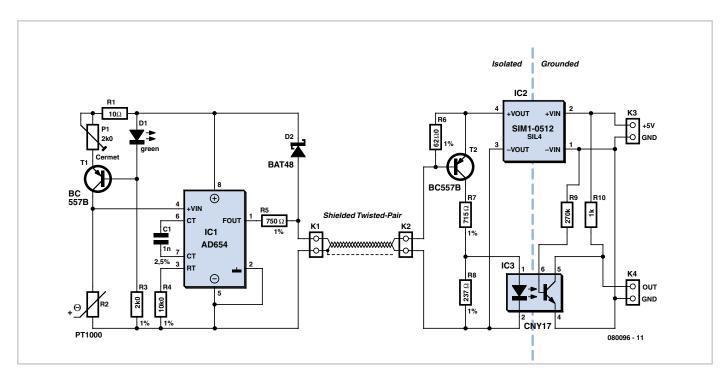
Finally, at connector K4 the signal is available with a low impedance, suitable for further processing.
