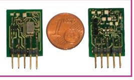
TEAclipper is then inserted into the target PCB and generates all the signals necessary to program the microcontroller. Connection is via a 5-pin header which also provides power to the TEAclipper. Since only a temporary connection is required, a socket is not necessarily needed. The pins can be pressed against plated-through holes in the PCB for the few seconds required for programming.
