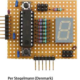
Thumbwheel switches are remarkably expensive and always playing hard to get. Here's a cheaper, digital equivalent with the ability to remember the value it was set to. It is programmable to different modes such as inverted or non-inverted BCD code output, programma-
