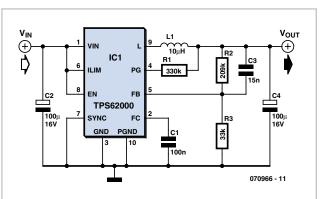
be higher than the desired output voltage. The output voltage is 3.3 V with the indicated component values and an input voltage of 5 V. If you want to reduce the component count even further, you can use a member of the family with a fixed output voltage. The available voltages are 0.9, 1.0, 1.2, 1.5, 1.8, 1.9, 2.5, and 3.3 V. With this approach you can omit R2, R3 and C3, so the output can be connected directly to pin 5.
