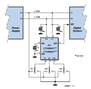
is that the larger the tolerance, the lower the internal threshold is set.
