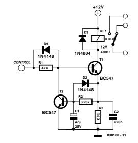
needed to completely discharge C1. T2 shunts the bias current of T1 when the delay has elapsed. Diode D1 helps to discharge C1 as quickly as possible. The relay shown in the circuit was specified at 12 V / 400 ohms. All component values for guidance only.
