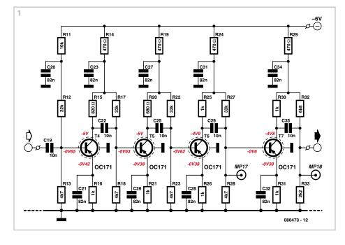
using an ohmmeter will not reveal faults in the junction proper. The device will also achieve its normal electrical specifications. However, an unexpected short-circuit may be measured between the shield wire (S) and the emitter or collector. In the 455 kHz IF amplifier shown in **Figure 1**, a dominoeffect with all transistor biasing occurs if, say, the collector of the first OC171 is shorted to the shield, hence to ground. This was a practical case and a trigger to start a research.
