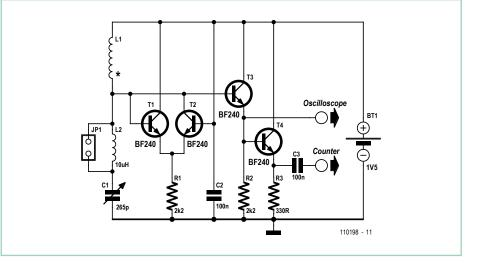
30 MHz. With jumper JP1 open an additional fixed inductance of 10 µH comes into circuit. The frequency measurement range is then from 2.5 MHz to 10 MHz. The switch may be replaced by a jumper.
