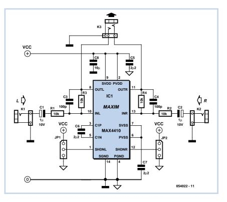
Each channel can be individually turned off (SHDNL and SHDNR) by jumpers JP1 and JP2. During normal operation these two inputs should be connected to the
