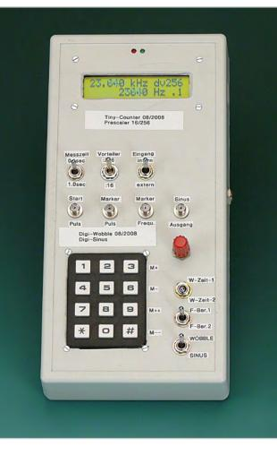
directly on the keypad in Hertz. For example, to enter 12 kHz, type '\*12000#'. The usable frequency range runs from around 10 Hz to
