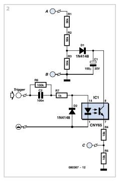
is nevertheless only a short pulse sent to the gate. R6 is necessary for the periodic discharge of C2. A standard 5 V digital signal is sufficient for driving this trigger input.
