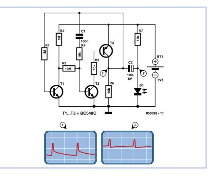
and a PNP transistor, which avoids wasting control current. The two transistors only conduct during the brief interval when the LED blinks. To ensure stable operating conditions and reliable oscillation, an additional stage with negative DC feedback is included. Here again, especially high resistance values are used to minimise current consumption.
