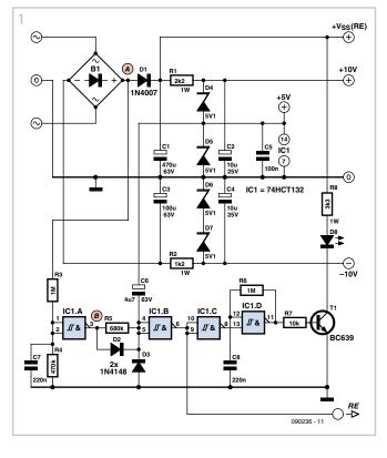
V rail. This circuit works by determining voltage thresholds: this means that we need to choose an SN74HCT132 quad Schmitt NAND gate for IC1.
