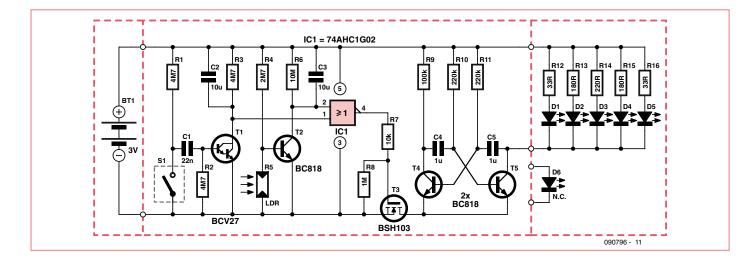
the NOR gate will go high, causing FET T3 to conduct. As a result power is supplied to the astable multivibrator comprising R9, R10, R11, C4, C5, T4 and T5, and the LEDs will flash at 5 Hz. They will continue to flash for as long as pulses continue to be supplied by the vibration sensor S1 and as long as it remains sufficiently dark.
