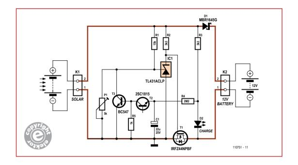
As the battery becomes fully charged, the oscillator's 'on' time shortens while the 'off' time remains long as determined by the timing components, R4 and C1. In effect, a pulse of current gets sent to the battery that will shorten over time. This charging algorithm may be dubbed Pulse Time Modulation.
