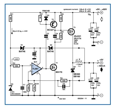
ers the IC from the output. Diode D1 becomes reverse biased reducing current through R1. When the circuit is first powered up the voltage on pin 2 of IC1 is below the reference voltage on pin 3, this produces a high level on output pin 6. The low power MOSFET T1 is switched on which in turn switches the
