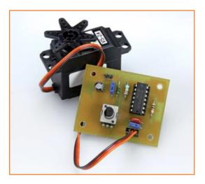
Figure 1. The circuit uses a dual timer IC.
