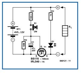
FET is negligible for the two types of FET specified (for a maximum load current of either 100 mA or 1 A).
