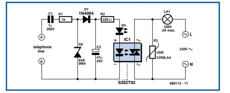
age on a fixed telephone line is pretty high. Since Europe and the EU Commission have not yet interfered, the exact value of this voltage and its frequency varies according to the country, but that's not important here. The line carries direct current whether unoccupied or occupied. Moreover, no more than a few hundred mAs needs to be stolen from an unoccupied telephone line to make the PSTN exchange believe the line is occupied.
