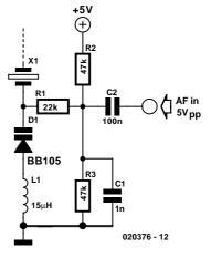
is also increased by a factor of 9. Crystals with frequencies near 10 MHz are relatively easy to find and inexpensive, so you should always be able to find a suitable frequency within the FM band. A crystal of 10.245 MHz for instance would give you a frequency of 92.205 MHz and 10.700 MHz results in an output of 96.300 MHz. You may find that the circuit operates on the border of the HC specifications. If this causes any problems you should increase the supply voltage a little to 6 V.
