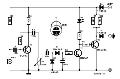
soon as the voltage across C4 rises above 0.5 V, T2 turns on and the LED connected to the collector of the transistor lights. T3 inverts this signal.
