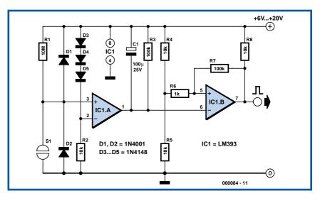
The power supply voltage for the circuit is not very critical. Any regulated DC
