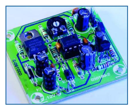
R6 + 1. The voltage offset is generated by IC2.A, which shifts the ground of the LM35, to which its output is referred, to a potential of 245 mV  $\times$  4.587 = 1124 mV relative to the circuit ground. Overall, this means that the voltage at the output of IC2.B is exactly 0 V at a temperature of -24 °C and 5 V at +84 °C.
