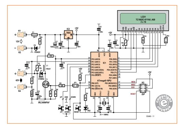
Figure 2. The microcontrollerregulated step-up converter.
