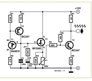
thus a linear sawtooth ramp, the capacitor is charged by a constant current source built
