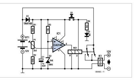
after the load has been disconnected, when the battery voltage rises above the reference voltage again, the reset coil will no longer be powered and the current consumption drops back to about 2.5 mA.
