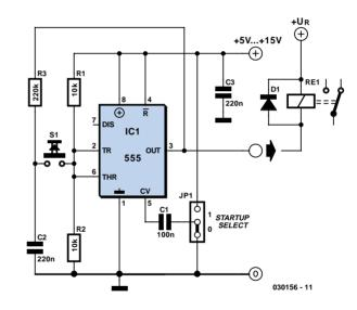
trigger input is less than 1/3 of the power supply voltage.
