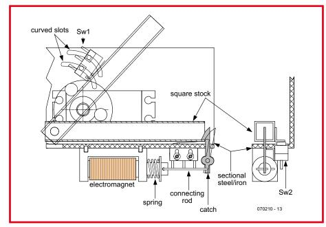
Figure 3. Mechanical construction details.
