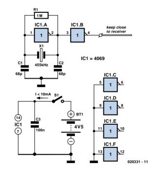
which is radiated from a length of insulated hookup wire wrapped several times around the receiver. The degree of inductive coupling needed to obtain a good beat note will depend on the IF amplifier shielding and may be adjusted by varying the number of turns. All unused inputs of the 4069 IC must be grounded to prevent spurious oscillation.
