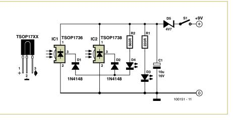
that even at 5 mA (the maximum output current of the receiver ICs) the indicator LED will light reasonably brightly. In his prototype the author used 5 mm LEDs with an output of typ-
