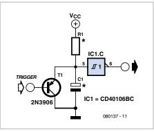
R1 to charge up capacitor C1, but not sufficiently to reach the positive voltage threshold set at input pin 5 of the gate. Consequently Schmitt trigger output pin 6 will remain High. For a retriggered pulse period of 3 seconds (or 0.3Hz) you'd use R1 = 330 k $\Omega$  and C1 = 10  $\mu$ F.
