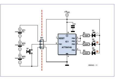
is only 20 mA per pin, the white LED is connected to two pins. Buffer capacitor C1 may be omitted if space is tight.
