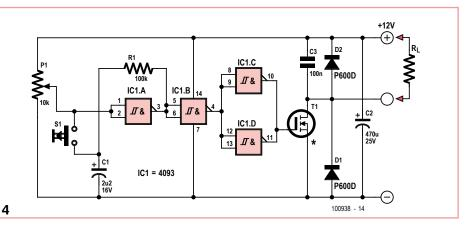
put when an N-MOSFET has to be driven (load returned to the positive rail). In both configurations, the relay remains off at power-on (safety feature).
