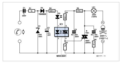
charges capacitor C2, which makes it possible to light LED D3 as well as the LED in the optocoupler IC1. This is no ordinary optocoupler, but is in fact an AC power zero-crossing detecting opto-triac, which allows us to control the chosen load while generating no, or less, interference, which would not be the case using a standard opto-triac.
