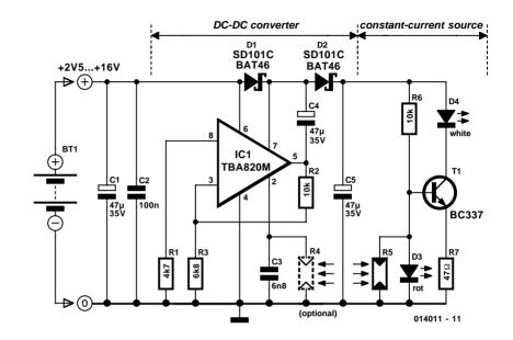
With the constant current source on its own the white LED would not be adequately bright when run from low voltages.
