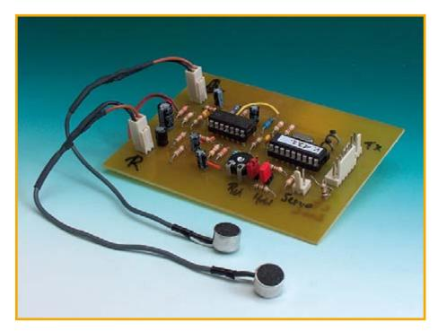
Figure 6. The binaural sensor prototype.
