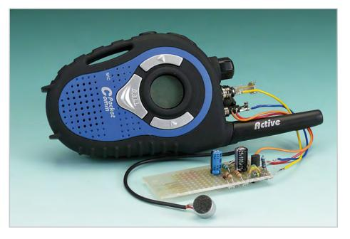
that can be obtained from Conrad Electronics (PMR Pocket Comm Active Pair, order number 930444). These walkie-talkies have separate jack sockets for the LS/Mic and PTT connections.
