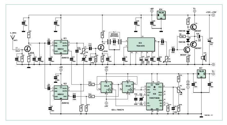
we've added a simple amplifier stage using a pair of transistors (BC547 and BC557) along with a potentiometer (P2) for the volume control.
