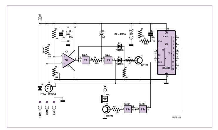
IC2.D, and T2, the sounder operates in time with the indicator.
