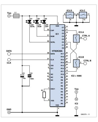
These switches are scanned many times per second in a matrix in order to detect the potential press of a key. The number of columns is usually eight (C0-C7 in the schematic); the number of rows varies for each type of keyboard and can range from 14 to 18 (R0-R17 with the HT82K28A keyboard encoder mentioned in the example). To each switch there is a single column- and a single row connection. The intention of the circuit is that sensor A will 'push'
