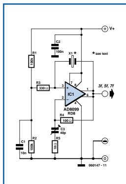
non-inverting input. The circuit amplification, which in principle must be unity to ensure oscillation, is determined by the network formed by R4, R5 and trimmer capacitor C3. This network is frequency-dependent such that the amplification increases as the frequency rises. The network gain is adjustable with C3. The setting of the capacitor must be such that the gain is too small for oscillation at the fundamental frequency, but sufficient for, say, the 5<sup>th</sup> or 7<sup>th</sup> harmonic.
