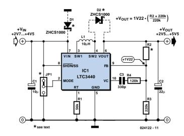
tion to the mark-space ratio of the switching signal. L1, together with the output capacitor, form a low-pass filter. If the input and output voltages are approximately the same, the IC switches into a pulse-width modulation mode using all four switches.
