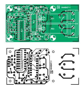
After the first pulse is transmitted, Re1 will be switched on via R7 and T1. The next pulse causes both Re1 and Re2 to be switched on. After the next pulse only Re2 will be on. The reset-input of the decade counter is connected via D3 to output Q4. This causes the switch to return to the rest position after the next pulse.
