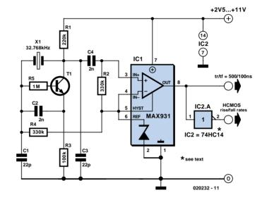
shift causes the oscillation. The bias voltage of 1.25 V for the comparator inside the MAX931 is defined by the reference via R2. The comparator's input swing is thus accurately centred around the reference voltage. Operating at 3 V and 32 kHz, IC1 draws just 7  $\mu$ A.
