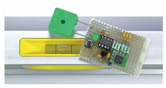
it was found that the circuit would still function with a supply voltage as low as 3.6 V. Maximum current was measured at 4.56 mA and averaged around 3.06 mA with the LED blinking and the tone sounding.
