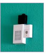
virtually self-explanatory: when the existing doorbell button is pressed to actuate the buzzer, the voltage is rectified by the bridge rectifier and regulated at 5 V by the 7805. This voltage drives the relay directly, causing the switch in the wireless doorbell button to be
