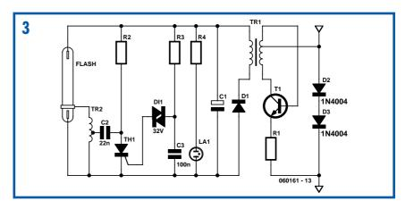
It's reasonable to reserve 24 V for 20 flasher units, with a protection resistor of about 10  $\Omega$  to limit the current surges, not forgetting a 1-amp fuse.
