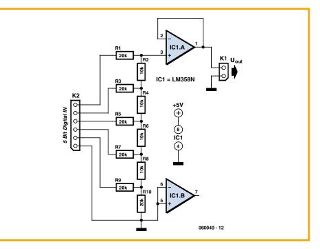
Figure 7. The resistor network functions as a simple D/A converter.
