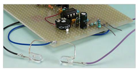
DIY electronics. By contrast, the variation in blood flow can easily be sensed using light transmission, since the absorption of the transmitted light depends on the blood flow. Ear lobes and fingertips are especially suitable for light transmission measurements.
