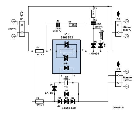
sensitive and will successfully switch the slave even when the master equipment draws very little mains current.
