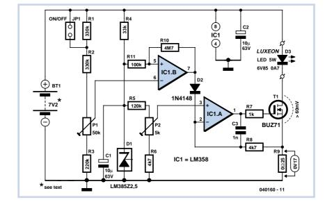
of using a semiconductor-based circuit. The inefficiency can be mitigated by using a modern device such as a power MOS-FET as the series component. Power loss is then limited to that in any current sense resistor that might be used and the dissipation in the relatively small 'on' resistance of the switching transistor.
