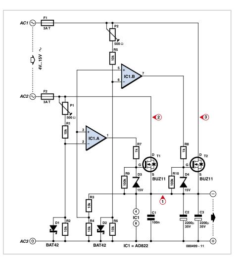
in the MOSFETs are only around 150 mW to 300 mW and so the devices do not need extra cooling. The potentiometers should not be set so that the MOSFETs conduct for longer than necessary, as this leads to brief short circuits of the input, audible as a humming of the transformer. It is best to start with the potentiometers adjusted to the centre of their travel.
