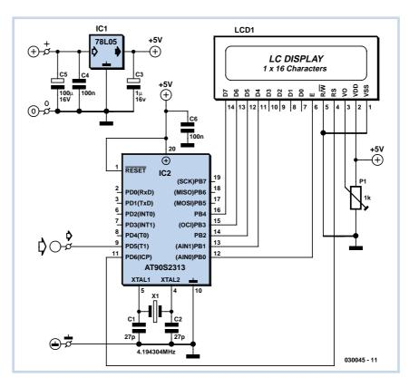
The program is written in AVR Basic and is small enough to be compiled and downloaded to the microcontroller by the free demo version of the BASCOM AVR compiler (Download from: www.mcselec.com). The single line LCD display interface is designed for a Hitachi 16x1 or compatible display. Preset R1 allows adjustment of the display contrast. IC1 provides a regulated 5 V for the microcontroller and display.
