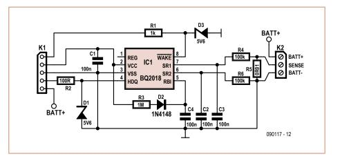
The same PCB contains shunt resistor R5 (Welwyn, 0.01  $\Omega$ , 1 W, SMD, 20 ppm/K). Since the maximum input to the BQ2018 is 200 mV this gives a full-scale of 20 A. A maximum of 200 A or 400 A might be appropriate for larger vessels, in which case you will use a lower value shunt. Metal-film resistors are recommended for R4 and R6 to keep noise and thermal drift to a minimum. R4, R5 and R6 should be connected in 'Kelvin' arrangement with heavy duty wires on the R5 terminals.
