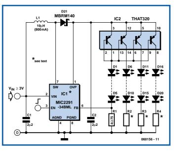
The circuit shows a type MIC2291 PWM step-up LED driver from Micrel driving a four-by-five LED array. This arrangement leaves the device a little headroom in terms of mark-space ratio and total power. The voltage at the output will be at most 18 V in normal operation. A particular advantage of the MIC2291 in this circuit is its low feedback voltage of 95 mV, which makes for a correspondingly high efficiency. The current in each chain is calculated as follows:
