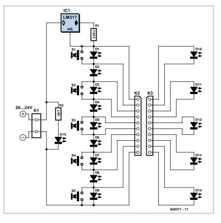
• Two LEDs opposite one another fail to light: two conductors are crossed or shorted.
