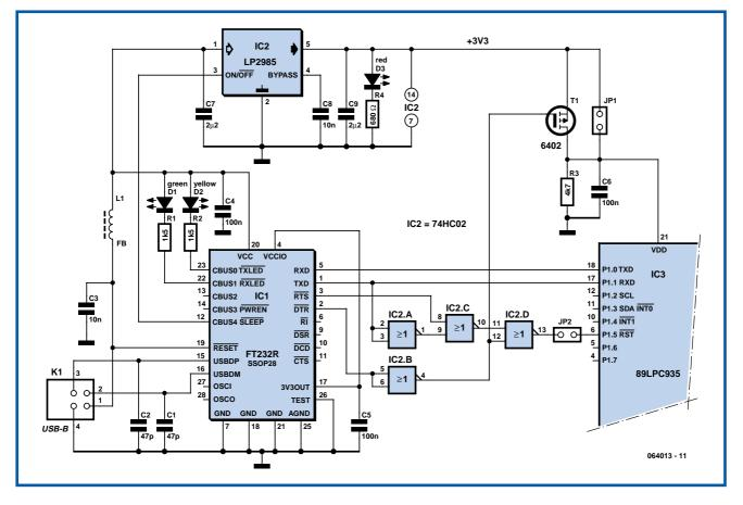
Back in November 2003 you could already read about a small development system for the (then) new series of controllers from the 8051-compatible 89LPC9xx-family. A nice feature of the current 89LPC9xx-series is that these chips can remain in the circuit while (re-)programming. All that's required for this programming is an RS232 port. But because many modern computers do not have an RS232 connection any more,
