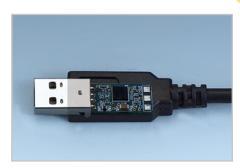
output are converted into RS-232 signals on the tiny board described here.
