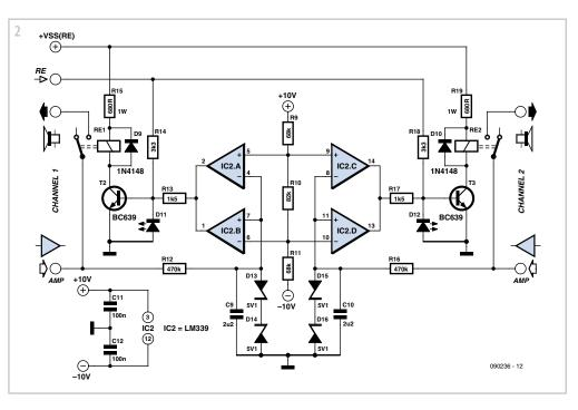
cause current to flow in the LEDs D11 or D12, indicating that the protection has been activated. Zener diodes D13 to D16 provide over-voltage protection for the comparator inputs. It's wise to make sure that R12 and R16 are indeed correctly connected to the amplifier outputs and not to the relay contacts feeding the loudspeakers. The choice of
