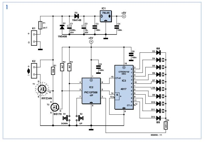
means of two pushbuttons. A PWM signal with a frequency of 100 Hz is generated, while the power is indicated with a classical 4017.
