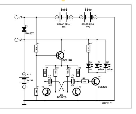
and one (D3) is a normal 3-mm red LED for control purposes. Of course it is possible to increase the number of LEDs to obtain higher brightness. However you will run into limitations regarding the maximum collector current of transistor T4. For really high power applications a MOSFET transistor is suggested instead of the common or garden BC547B.
