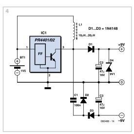
Applications of this attractive device as a voltage source are also worth a quick look. For example, you might be looking for an application for the printed circuit board, with PR4401 IC and coil ready fitted, that came free with the September 2007 issue of *Elektor*.
