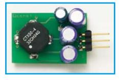
producing a steady DC voltage of 12 V at its output over input variations from 13 V to 25 V, at loads of up to 750 mA. Its three-
