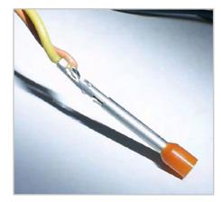
the pressure. Exactly as this click is heard you need to remove the wire in question, with its pin, from behind out of the plastic housing. If this doesn't work exactly as desired, it can help to twist the sleeve around while you are pulling. Normally you can release about four pins using one sleeve. For assured reliability, however, it is recommended to use several
