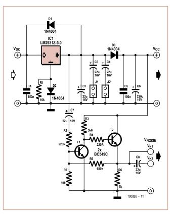
output resistance of the amplifier is relatively low and the output signal could be used to directly drive the input of an ADCs. The gain of the transistorized amplifier may be changed to requirement chiefly with resistor R3.
