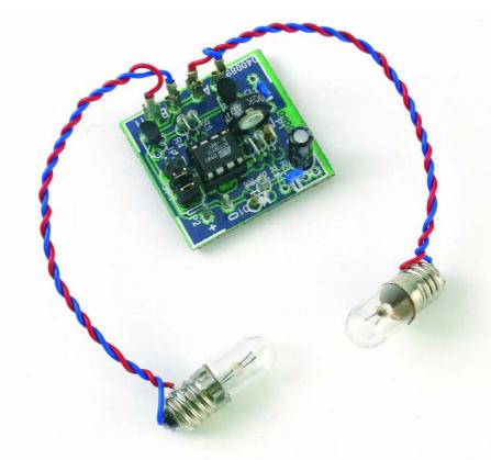
making the board and populating it should not present any difficulties, thanks to the absence of SMDs. The total component cost is very low, at around two or three pounds, not including the circuit board. Power can be obtained from any regulated 5 V supply. If only an unregulated supply is available, then this should be connected to V+. Current consumption is of course mostly dependent on the choice of lamp.
