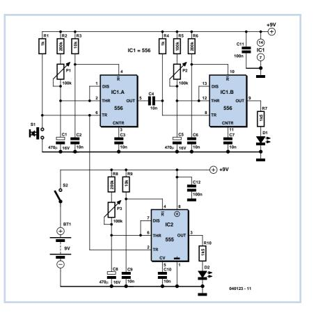
IC1b, is thus triggered. Its pulse duration is set at one minute, determined by C5, R5 and P2. D1 thus lights for one minute. Potentiometers P1, P2 and P3 allow the various time intervals to be adjusted to a certain extent. If considerably shorter or longer times are wanted, suitable changes should be made to the values of C1, C5 and C8. The period of the monostable is given by the formula
