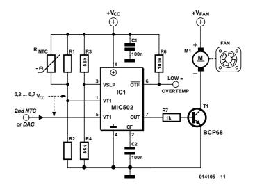
up to the desired logic level with an external resistor.  $\overline{\rm OTF}$  switches low when one of the two inputs VT1 or VT2 rises above 0.75  $V_{cc}.$
