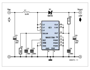
Schottky type: for a 1 A output current the SB140 is a suitable choice. For L1 a fixed power inductor, for example from the Fas-
