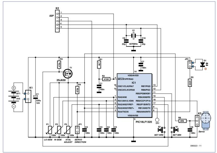
The circuit is powered by three 1.5 V cells. Depending on the size of the servo used, it may be better to replace the batteries by a small plugtop adaptor supplying 5 V. You can also use three NiMH rechargeable cells, well known to model enthusiasts. The microcontroller's 'brown out' facility, set at 2.7 V, will avoid deep discharging the batteries by maintaining the microcontroller in reset if the threshold is reached.
