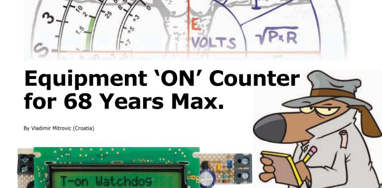
Have you ever wondered how long a piece of electric equipment has been switched on and consuming AC power? The simple circuitry shown here counts the seconds of the ON time periods and keeps the total accumulated time in the EEPROM inside the ATtiny13 microcontroller. Just read the EEPROM with the help of an appropriate ISP programmer or the dedicated readout circuit and you will
