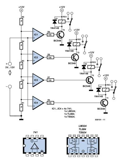
above +12 V) are out of the question. If you do need a switching level in the range 0-1.5 V, consider using an LM324, which contains four opamps in one package. For the high side of the range (10.5 to 12 V), a TL084 or a 'rail-to-rail' opamp like the TS924 is required. However, the TS924 cannot be used with supply voltages above 12 V.
