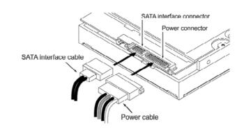
plexing choice! The parallel ATA bus operates with 16 bits simultaneously; the serial bus therefore has to be at least 16 times faster to obtain the same equivalent speed. That is why SATA operates at a clock speed of 1500 MHz and reaches a data transfer speed of 150 MByte/s; versions with 3 GHz and 6 GHz clock speed are planned. The industry made this choice because,
