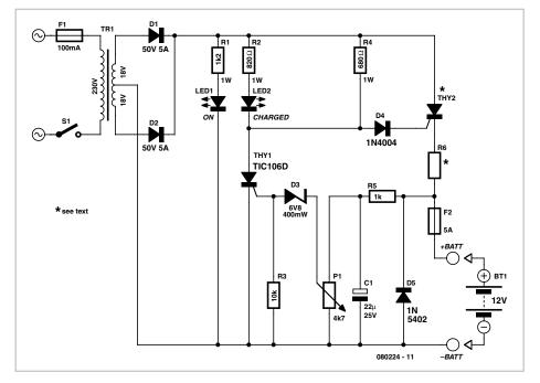
battery is effectively charged, the charging current being limited only by resistor R6, which has to be calculated as shown below. This thyristor is triggered via resistor R4 for each half-cycle of the mains, except when thyristor THY1 is itself triggered. In that event, THY2 turns off the first time its supply voltage drops to zero, and no further current can reach the battery.
