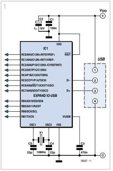
counters, timers, SPI, I<sup>2</sup>C, UNI/O, etc. The USB interface is designed so that all the programming is done on the PC rather than on the chip, which saves a lot of development time.
