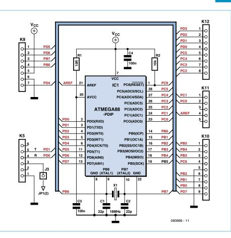
a 6-channel ADC, as against eight for the TQFP version. Apart from this subtle difference, the ATM18-DIP board is similar to its smaller sister in virtually every respect. Virtually, since we must note the following niceties all the same: – connector K12 is moved to the top;
