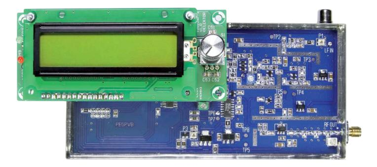
By Sjef Verhoeven, PE5PVB (The Netherlands) Most amateur radio transmitters are not actually designed for transmitting wideband audio signals with high fidelity. However, the wideband 70-cms (430–440 MHz) FM exciter described here is up to the task, with an audio bandwidth of 20 Hz to 100 kHz.
