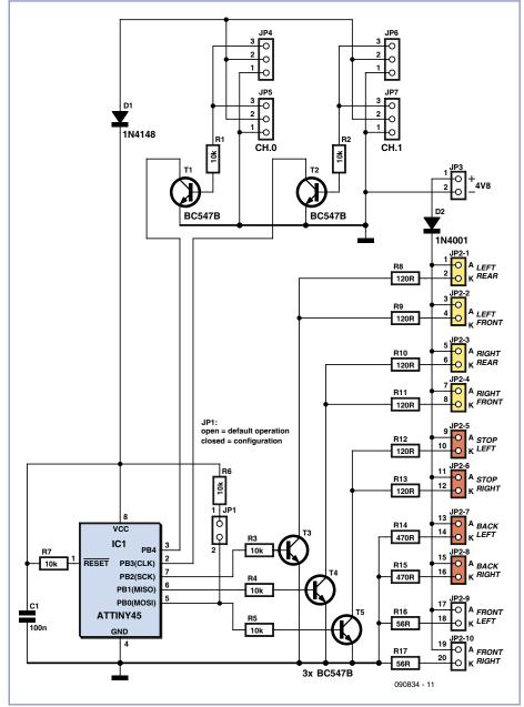
off. Fit jumper JP1 to enable configuration mode, switch on the radio control transmitter, set all proportional controls to their centre positions, and then switch on the receiver. The indicator LEDs should first flash on both sides. Then the car will indicate left for 3 s: during this time quickly turn the steering on the radio control transmitter fully to the left and the throttle to full reverse (maximum braking).
