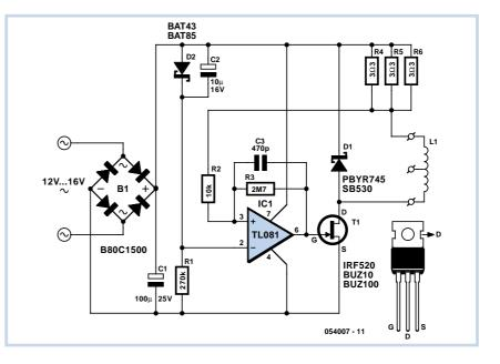
winding increases from zero until it reaches about 0.5 A. At this current the voltage drop across R4-R7 becomes greater than the reference voltage across D2 and the opamp will turn off the FET. The current through the winding continues flowing via D1, gradually reducing in strength. When the current has fallen about 10% (due to hysteresis caused by R3), IC1 will turn on T1 again. The current will increase again to 0.5 A and the FET is turned off again. This goes on continuously.
