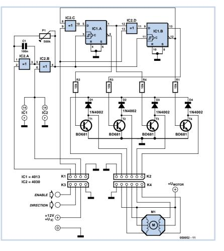
Swapping the outer two coil connections on one of the windings will reverse the direction if this is necessary.
