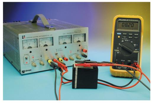
ered charged. It is not a disaster if the battery is connected for longer; overcharging is not possible provided the voltage is less than 4.1 V per cell.
