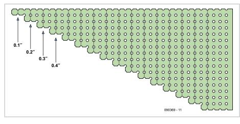
a piece of wire and fold it sharply around the indentations corresponding to the selected pitch. A neat wire link is the result, with exactly the right pitch and ready for soldering tightly into the PCB or prototyping board. With close-fitting wire links the board looks much better and they are also mounted much more quickly.
