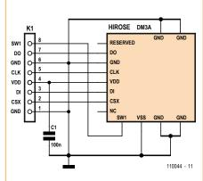
Type DM3 is available in three versions: as push-push type DM3A, as the hinged variant DM3C and as the push-pull connector DM3D. These connectors can be soldered simply with a normal soldering iron.
