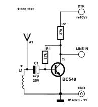
So where is the tuning capacitor? It's not needed, since the receiver has an extremely wide bandwidth and (simulta-
