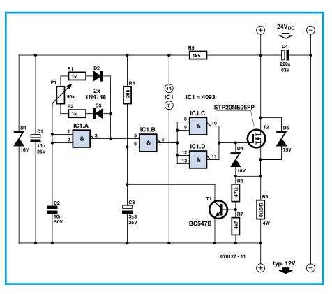
unavoidable in this circuit because of the inductance of the wiring. Any standard N-channel FET able to withstand 100 V can be used for T2.
