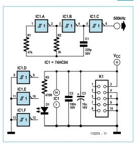
the frequency of around 500 kHz may vary by around  $\pm$ 50 kHz. This doesn't affect the operation of the probe.
