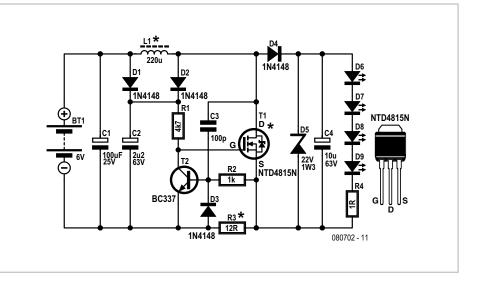
tor R3, this keeps T2 turned on and T1 turned off, so the flyback phase is not clamped until it has given up all its energy. Capacitor C3 provides positive feedback to ensure reliable oscillation and sharpen up the switching edges. Components D1, D2 & C2 form a bootstrap boost circuit for the MOSFET gate, although it is logic level it only guarantees the stated  $R_{D-S(on)}$  at a  $V_g$  level of about 8 V — by happy coincidence the combined  $V_f$  of
