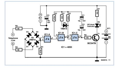
If, for some reason, you wish to change the flash frequency or on/off ratio (duty cycle) then do feel free to experiment with the values and ratio of R1 and R2. The effect will also depend on the brand of the 4093 IC, its exact logic High/Low switching thresholds and hysteresis. The circuit is not approved to BABT standards for connection to the public switched telephone network (PSTN). Please check local/national regulations.
