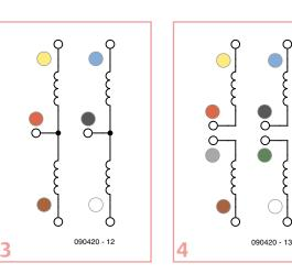
For a motor with **4 wires** we have to find two wires that have a resistance between them. We then write down the value of the resistance and the color of the wires. In this way, you can distinguish between the two stator coils and we know that this is a bipolar motor.
