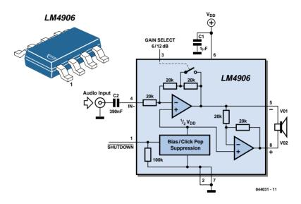
swing for a specified supply voltage. Four times the output power is possible as compared to a single-ended amplifier under the same conditions (particularly when considering the low supply voltage of 5 to 6 volts).
