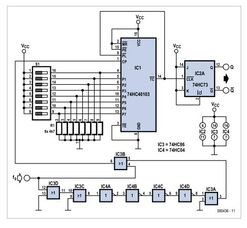
ever the counter reaches zero the terminal count pin ( $\overline{TC}$ ) generates a negative pulse, reloading the counter (via parallel load  $\overline{PL}$ ) with the binary switch setting. The counter continues counting down from this value.
