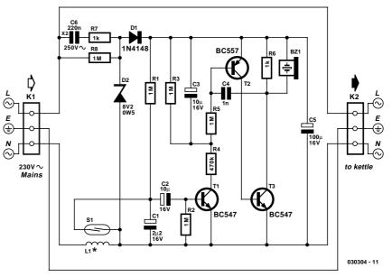
negative going pulses whose basic frequency will depend on the value of C4 and R5. The pulses will be reproduced in the piezo sounder as a tone.
