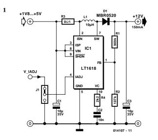
In the form of the LT1618, Linear Technology (<u>www.linear-tech.com</u>) has made available a step-up switching regula-
