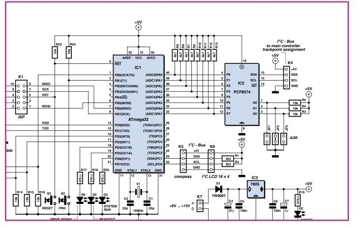
Figure 1. The ATmega32 communicates with the compass and the LCD over an I<sup>2</sup>C bus; the GPS mouse is connected via RS-232. The PCF8574 I<sup>2</sup>C interface chip takes on the task of accepting a control byte and making it available on pins 33 to 40 of the ATmega.
