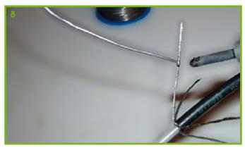
Cover the bundles with solder. Although this step is optional, it does enable the ground plane elements to hold their shape better, and prevents untwisting of the strands.
