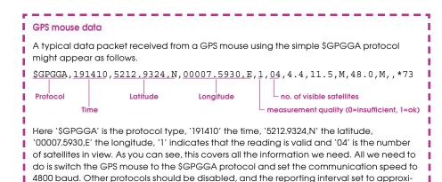
mately 1 s. The settings are made using the software provided with the GPS mouse.
