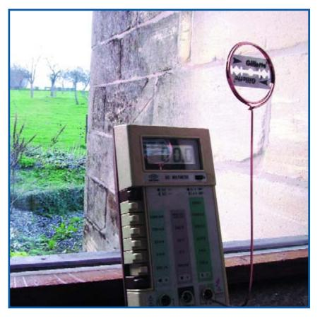
blade somewhere. Attach this razor blade at the top of the antenna. And again, be careful: keep children and pets away. In the picture you can see an assembly were the top of the antenna has one turn. The razor blade is clamped in this and in addition it is a lot harder to injure yourself this way.
