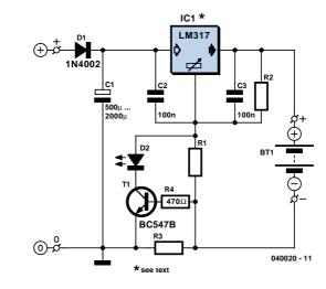
a certain minimum number of cells. For an LM317, the voltage between the reference lead and the output is 1.25 V, which means at least three cells must be charged ( $3 \times 1.45$  V > 2.9 V + 1.25 V). For a 78xx with a voltage drop of around 3 V (plus 2.9 V), the minimum number is four cells.
