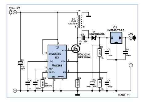
bilised 5 V from the 6-V output (with ripple voltage). The efficiency should be
