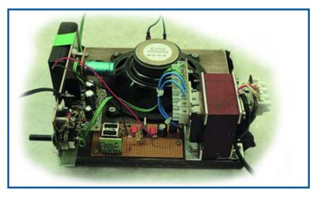
ously whether the amplifier is on or not (the author used a 15-pound speaker set / amplifier for a computer which switches the 12 volts AC). The transformer was replaced with a double secondary winding to avoid any earthing problems between the USB charging device and the amplifier ground.
