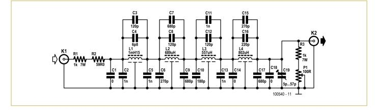
ful Class D power amplifiers. The theoretical values have remained the same as those in the original circuit, and the circuit itself has hardly changed. The biggest improvement is in the way the inductors are made. These are now substantially larger and have an air-gap, which reduces the distortion.
