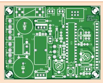
Figure 3. The step-up converter PCB.
