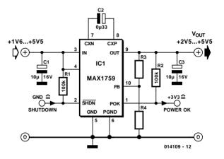
produce an externally settable output voltage between +2.5 V and +5.5 V, as given by the following formula: V<sub>OUT</sub> = 1.235 V (1 + R3/R4)
