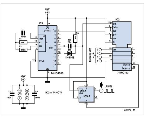
The mark/space ratio is only programma- ble up to 15/16 rather than 16/16; a binary input of 0000 produces a continuous low
