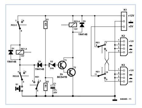
changeover switch would do the job, but that has the disadvantage that it is possible to forget to reset the switch to child mode after use, especially if the switch is hidden. A better solution is to have to press a (hidden) button during boot to put the machine into parent mode. We will now see how this is done.
