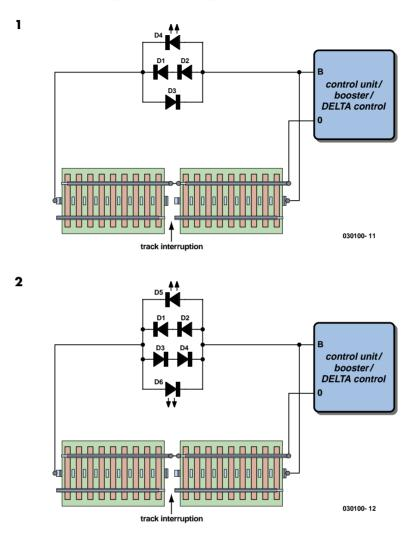
through D3. With a motor current of approximately 250 mA, the voltage drop across a single diode (1N4001 types are used here) is a good 1 V.
