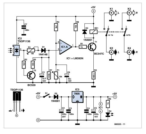
other input on pin 2. This reference voltage, which can be adjusted with P1, determines the switching threshold of the comparator. If IC2 receives an IR signal, T2 conducts, and as a result the voltage on C1 drops rapidly below the threshold level set by P1. This causes T1 to change from its previous 'on' state to the 'off' state. As a result, the relay drops out and the audio link to the stereo system is interrupted for the duration of the noise interval. It's all quite simple, as you can see.
