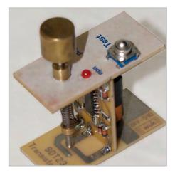
in other words the transistor is defective. An internal short circuit (connection between C and E) is indicated by the two LEDs glowing dimly. A functional NPN transistor conducts only when the voltage on C is higher than on E. LED D1 Is now short-circuited and only D2 flashes. In similar fashion only D1 flashes for a PNP device. The circuit draws only 10 mA or so and using pushbutton S1 for operation means that the battery will have a very long life.
