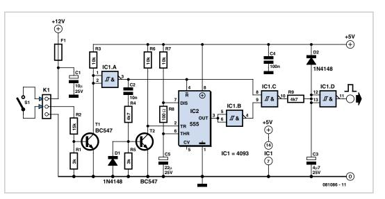
T1 conducts, and the output of inverter IC1. A, and hence also pin 8 of IC1.C, go high. If we now arrange things so that for a preset time the other input to IC1.C remains low, the trigger signal will not be propagated to the output until this period has elapsed. In the case of the author's garage door opener, this will only happen if the button on the transmitter is held down.
