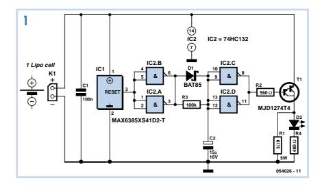
The IC (IC1) normally ensures that the microcontroller receives an active-high reset signal whenever the supply voltage drops below 4.1 V. By contrast, the output goes low when the voltage is 4.1 V or higher.
