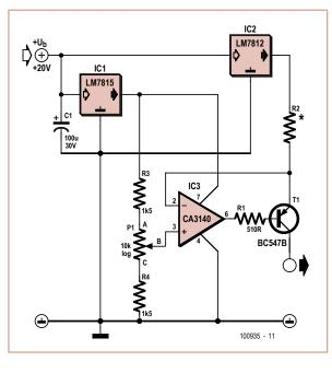
emitter of T1 (the instantaneous voltage) is maintained equal to the voltage at the wiper of P1 (the reference voltage). For all this to work it is of course necessary that a load is connected at the output of the circuit, so that a current can flow to ground.
