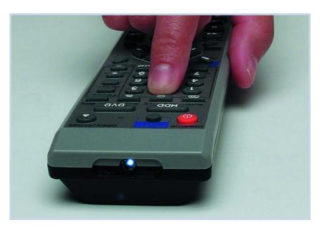
play, aim the remote control unit toward the camera, and press one of the buttons on the remote control, you should see a blinking light coming from the IR LED. If the LED remains dark, you can safely assume that the remote control unit is defective.
