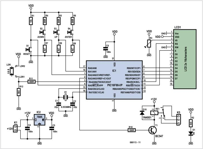
'high' during normal operation (and 'low' for a reset). Hence this input has been connected to the positive supply voltage via pull-up resistor R1.
