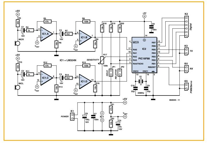
Figure 3. The circuit has two audio channels each with an electret microphone and two-stage amplifier. The two amplifier outputs are connected to the two A/D converter inputs on the microcontroller. take around 500  $\mu$ s to travel the distance between the ears which equates to a half cycle or a 180° phase shift between the two signals. At frequencies of 1 kHz and above it is no longer clear if the signal in one ear leads or lags the other ear.
