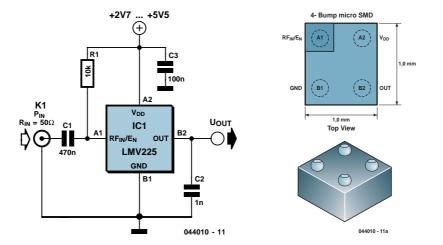
with a slope of 40 mV/dB. The output is 2.0 V at 9 dBm and 0.4 V at -40 dBm. A level of 0 dBm corresponds to a power of 1 mW in 50  $\Omega$ . For a sinusoidal waveform, this is equivalent to an effective voltage of 224 mV. For modulated signals, the relationship between power and voltaae is a several e ages fo impeda around the cha
