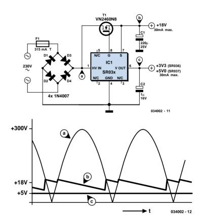
**Warning:** This circuit must only be used in a fully encapsulated enclosure with no direct connections to any external circuit. It is important to be aware that the circuit is connected to the mains and the chip has lethal voltages on its pins! All appropriate safety guidelines must be adhered to.
