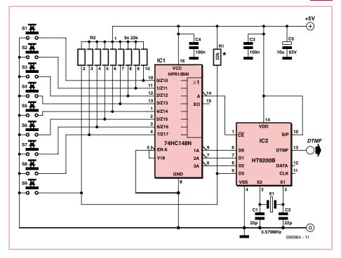
A 74HC148 8-to-3 priority encoder is used to convert the 'keypad' information from S1–S8 into 3-bit tone selection words the HT9200B wants to see at its input. The ninth switch, S9, is connected to input D3 on the encoder chip. Pressing one of the switches S1–S8 generates a complementary 3-bit binary word at outputs A0, A1, A2 of IC1. IC2 then generates the dual tones accordingly to these binary codes.
