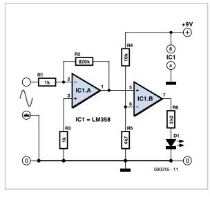
slowly, with the result that the LED will remain dark, but it will generate a signal if the wheel is turned faster and the LED will thus start blinking. Irregularities in the blinking rate can be caused by dirt on the sensor or damage to the pole wheel (gear wheel).
