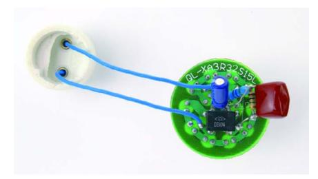
Did it ever occur to you that an array of white LEDs can be used as a small lamp for the living room? If not, read on. LED lamps are available ready-made, look exactly the same as standard halogen lamps and can be fitted in a standard 230-V light fitting.
