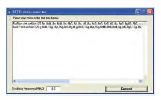
The data section consists of a set of character strings separated by commas, where each string contains a duration, note, octave and optional dotting (which increases the duration of the note by one half). For example here is RTTTL ringtone for the famous *Für Elise* piece: FurElise:d=4,o=6,b=125:8e, 8d#, 8e, 8d#, 8e, 8b5, 8d, 8c, a5, 8p, 8c5, 8e5, 8a5, b5, 8p, 8e5, 8g#5, 8b5, c, p, 8e5, 8e, 8d#, 8e, 8d#, 8e, 8b5, 8d, 8c, a5, 8p, 8c5, 8e5, 8a5, b5, 8p, 8e5, 8c, 8b5, 2a5
