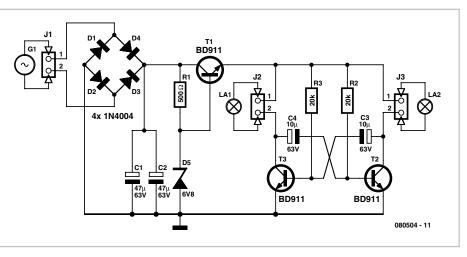
the front light and the rear light. The frequency is determined by the RC time-constant of R3 and C3, and R2 and C4. This time can be calculated with the formula:
