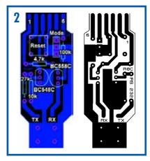
facing toward the R8C. Then, connect the 9-way sub-D plug to the RS232 port on the PC. Turn the setup on, slide the Mode switch toward the top, and push the Reset button. Now, all that's left to do is start programming the chip.
