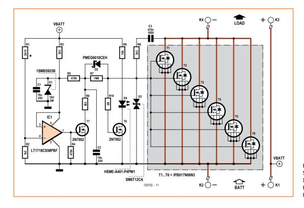
Figure 2. Schematic of the X-Treme Inrush Current Limiter. High current PCB tracks are highlighted and thicker.
