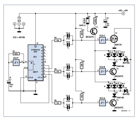
The power consumption of the circuit depends largely on the LEDs used. With the Rapid LED types shown, about 70 mA may be
