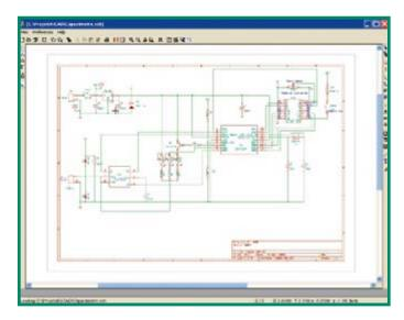
Figure 2. EeSchema: easy schematic capture.
