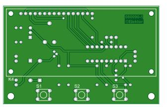
temperature sensor, type DS1820, also serves an important role in the circuit (connected to K5). Fortunately the DS1820 is already factory calibrated, so this saves us from a difficult task. A classic 7805-regulator and a common transistor pretty much complete the circuit. The clock source for the PIC is supplied by a 4 MHz ceramic resonator with built-in capacitors (Conrad Electronics order number 726406/726507).
