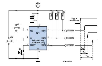
The TD input allows the length of the reset signal to be programmed and jumper JP2 gives the following three possibilities:
