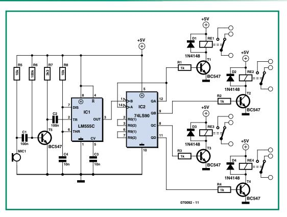
ple, when the first pulse is applied to the 555's TRIG input, the binary coded output on the 7490 will be 0001, for the second pulse the output will be 0010, and so on. For the 15<sup>th</sup> pulse, the output will be 1111. On receiving the next pulse, IC2 automatically cycles back to state 0000.
