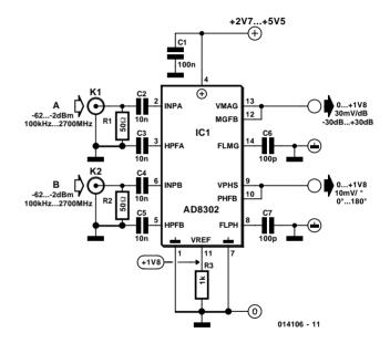
The IC has a bandwidth of 30 MHz, which can be reduced by fitting a capacitor between pins 8 and 14. Pin 11 is a + 1.8 V reference voltage output which can be used when further processing the outputs of the device.
