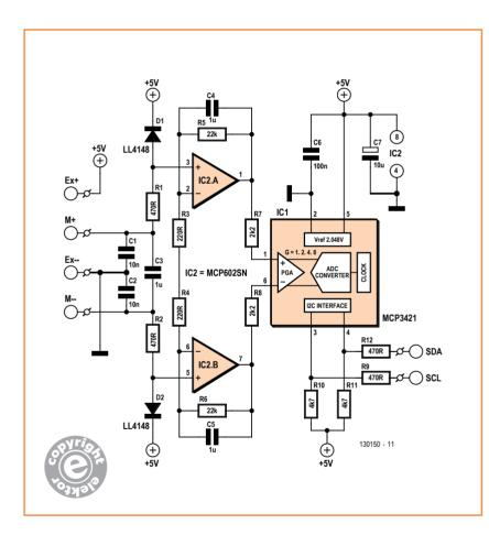
Figure 1. Circuit of the measurement interface.
