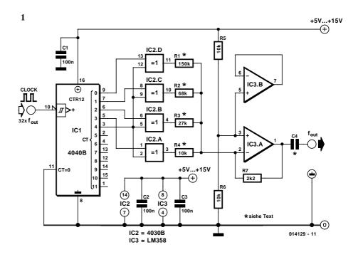
a problem in the circuit being driven, a coupling capacitor C4 must be fitted: the lower the operating frequency and the lower the load impedance, the greater the required value of capacitor.
