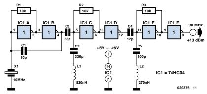
drive a diode-ring balanced mixer directly. The circuit can be used for any output frequency up to about 100 MHz by varying the component values. When, for example, an 8 MHz crystal is used to obtain an output frequency of 72 MHz (9 x 8 = 72), the frequency determining inductors and capacitors have to be adjusted by a factor of 10/8. You should round the values to the nearest value from the E12 series.
