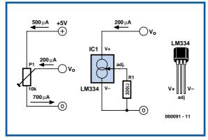
presented here ensures that there is a current of 200  $\mu$ A to ground, independent of the power supply voltage. By substituting a 2.2-k $\Omega$  potentiometer for R1, the current can be adjusted as desired. The value of R1 can be calculated as follows:
