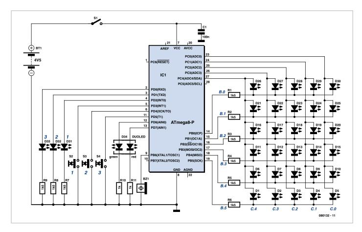
The software for the ATmega8 was generated using BASCOM, and it can be compiled with the demo version. The BASCOM source code and a hex file can be downloaded from the www.elektor.com — the archive file number is 080132-11.zip. A preprogrammed microcontroller is also available (order no. **080132-41**).
