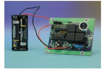
This circuit uses just two standard logic ICs which, with the accompanying receiver, forms a four-channel remote control and has been designed for use with the 'Audio/Video Switch' and the 'Switchbox for Loudspeakers' (shown elsewhere in this issue, as is the IR Rreceiver).
