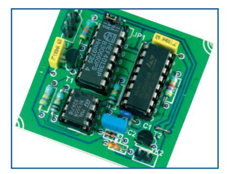
The aforementioned 555 is configured as a one-shot. The pulse-duration depends on the combination of R2/C1. Lowering the voltage on pin 5 also affects the time. This results in reducing the length of the pulse. In this circuit the pulse at the output of IC will last just over 1.5 ms when T1 does not conduct. When T1 does conduct, the duration will be a little shorter than 1.5 ms. We will explain the purpose of
