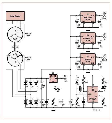
erator), which provides the power for the data logger and associated electronics.
