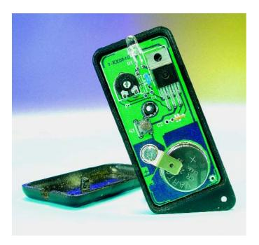
This mini pocket torch combines the advantages of Lithium button cells with a super-bright white LED. The lithium cells are small, have a long shelf life and have very little self-discharge. The LED has very high efficiency, an extremely long life expectancy and a modest current consumption (20 mA). In combination this results in an exceptionally long-life pocket torch.
