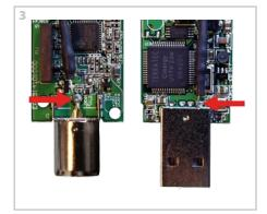
sourced from the computer's USB connector. If we connect this supply via a coil to the antenna input the problem is solved: the coil will present a high impedance to the high frequencies in the TV signal.
