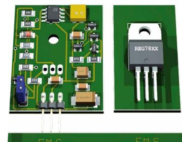
in the form of C1 and C4. The PCB design [1] is double-sided. All of the SMDs are fitted on one side, and the BD136 is fitted on the other side (the copper side). If desired, the power transistor may be fitted with a heat sink and insulating washer. However, the low-drop design makes a heat sink largely unnecessary. The small PCB can be fitted in place of a conventional voltage regulator IC, since IP1 is pin-compatible.
