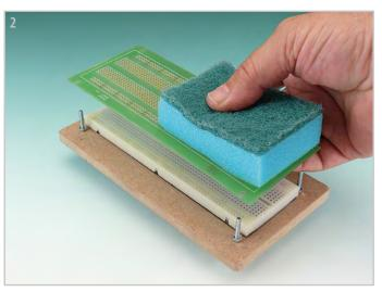
pins). In a circuit built using this arrangement, the contact strips in the breadboard provide the interconnections, so there's no need for soldering.
