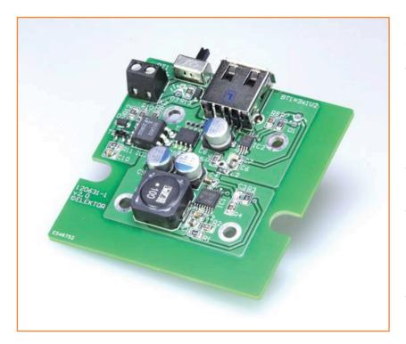
It's great that phone & gizmo manufacturers increasingly fit their devices with USB connectors as the charge port, but chargers are unlikely to be compatible between fruit and non-fruit platforms, and different manufacturers. For example, some devices expect specific voltages on the data lines, or simply a connection (resistor) between the data lines to recognize a charger (Dedicated Charger Port or DCP). The TPS2511 supports three of the most common protocols:
