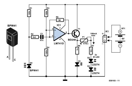
ordinary visible-light LED that flashes when an IR signal is received from the remote. With regard to the setting of P1, do not make the IRED current higher than necessary to reliably reach the final destination of the IR signal. Also, the currents mentioned above are peak levels — due to the small duty factor of the IR pulses, the average current drawn from the battery will be much smaller.
