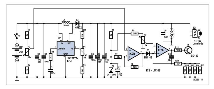
LEDs. One half of the dual op amp IC2 forms an adjustable current source while the other half switches the light off when the supply voltage sinks too low to avoid discharging the cells too much.
