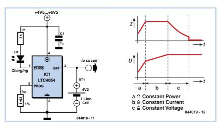
age. The under-voltage lockout circuit is then activated, with less than 2  $\mu$ A being
