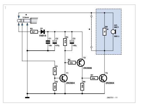
D1 provide a discharge path for the capacitor. C2 ensures that the circuit won't react to spikes caused by interference. As can be seen from the second circuit diagram, use is made of two connectors, a 2.5 mm jack plug for an external headset and a 3.5 mm plug for the PTT function. These connectors are particular to the walkie-talkies we used here. With other types of walkie-talkie you should first check the connection details of the connectors before you connect the circuit up.
