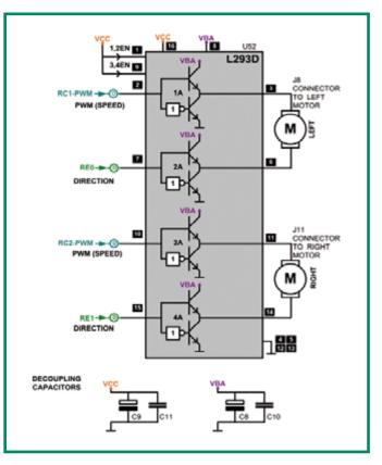
Figure 3. The L293D Double H-bridge motor driver circuit.
