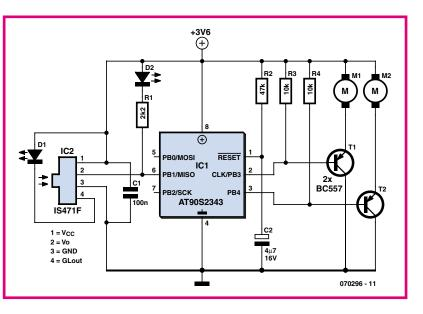
turn left or right, depending on an internal counter. If it still sees the obstacle it continues turning in the same direction until the obstacle disappears from view.
