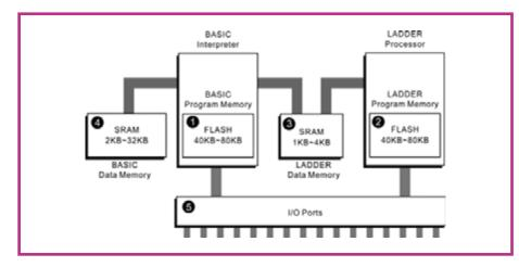
Figure 2. Internal architecture of the Cubloc CB220.
