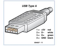
The other wires are used for the actual USB signals. A nice detail is that Microsoft uses exactly the same colours for these wires as those specified in the USB standard, which makes them much easier to recognise.
