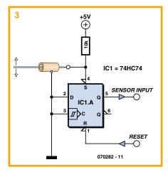
as shown in **Figure 3**. The microcontroller in the robot can then read the state of the flip-flop at its leisure and then reset it.
