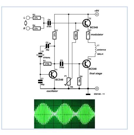
can also be checked using an oscilloscope. Clean amplitude modulation should be clearly visible.
