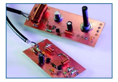
this, it is better to wind the two coils as one, that is, 30 turns with a tap than to wind two separate coils (see photograph). (040383-1)
