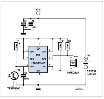
The type CR2032/1HF Lithium cell has a rated capacity of 230 mAh and a nominal voltage of 3 V [2]. On this basis with the typical current in sleep mode the battery would last over 250 years, or effectively for its shelf life, so a CR2032 with tags is worth soldering in to a PCB. Even at the maximum Sleep current, it would last for over 30 years — certainly longer than the fridge! One advantage of a Lithium battery is its long shelf life, and
