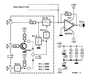
ground. When the switch input goes 'low', IC1a is opened and IC1b is closed and the audio signal is amplified by the opamp.
