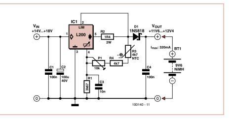
The charger circuit can be connected permanently to the battery pack. Charging starts when a 'plugtop' adaptor is connected to the input of the charger. The unregulated 12 V supply used by the author delivered an open-circuit voltage of 18 V, dropping to 14 V under load. Even though the charge voltage is reduced when charging is complete, the cells should not be left permanently on charge.
