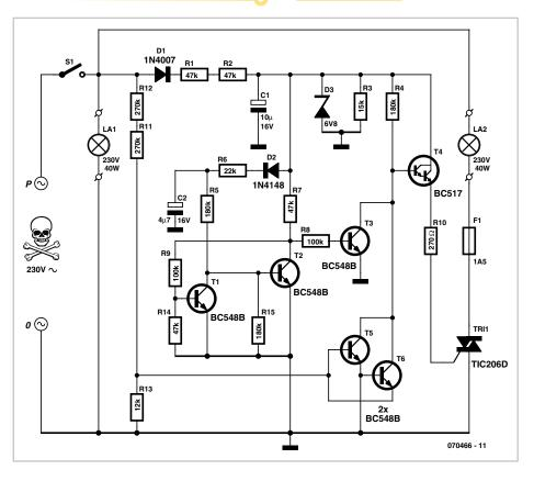
a little later, but when T1 turns on it diverts the base current away from T2, which therefore remains turned off. This situation is stable: the base of T3 is not pulled down and so this transistor conducts.
