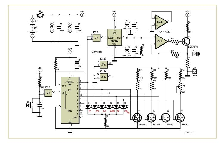
press of the button advances this high to the next output. The outputs switch FETs which in turn connect the voltage divider networks to ground to produce the different gain settings. The outputs also have LEDs, giving a visual indication of the output voltage level setting.
