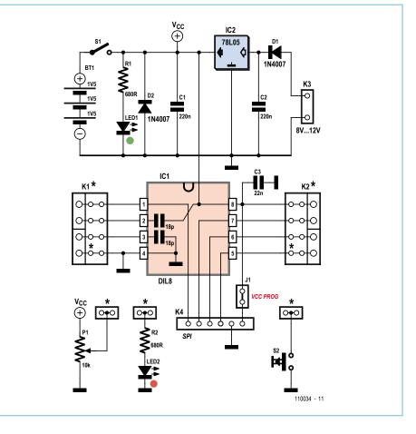
Their rather unorthodox connection (one to ground, the other to +5 V) has made it possible to simplify the PCB layout slightly. The 1N4007 diodes can be either conventional or SMD types, as can the resistors and
