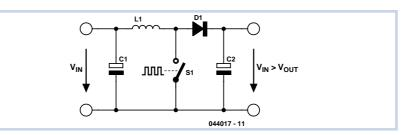
rent limiting. This means that very large currents can flow via coil L and Schottky diode D. Such currents can overload upstream components or destroy circuit board tracks.
