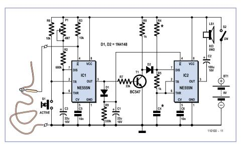
the hoop touches the wire), the monostable returns to the quiescent state. This causes IC2 to generate the low buzz sound. D1 is now reverse biased and C1 discharges through the relatively high-valued resistor R9. After a few seconds the voltage across C1 falls sufficiently that the buzz stops and the circuit is ready for the next player.
