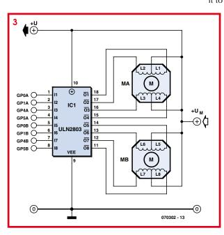
shown in **Figure 3**. This uses a standard ULN2803, usually used to drive relays, but which includes eight medium-power Darlingtons along with their protection diodes. So, this IC is able to properly drive any kind of single-pole stepper motor, as long as the voltage required doesn't exceed 50 V and the current per winding is under 500 mA.
