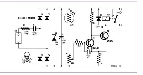
into conduction. This diverts the base current away from T2, with the result that the relay drops out. The switching level can be adjusted with the potentiometer. Capacitor C4 provides a bit of hysteresis to prevent the circuit from jittering near the threshold level.
