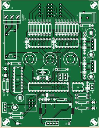
Figure 5. The circuit board layout. All of the user interface elements are located on the underside.
