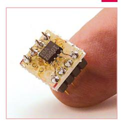
Any recommended supply decoupling capacitors can be mounted directly on the carrier board across the supply pins.
