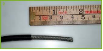
Cut off about 40 mm of the outer insulation. This will expose the braid that forms the cable shield.
