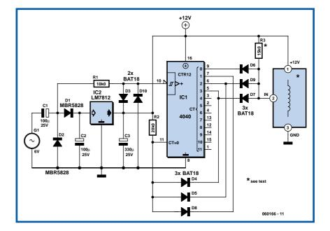
wheel was adjusted to 16/14th of the real size in the setup of the cycle computer. In that case you can leave out D4, D5 and D8. (060166-1)
