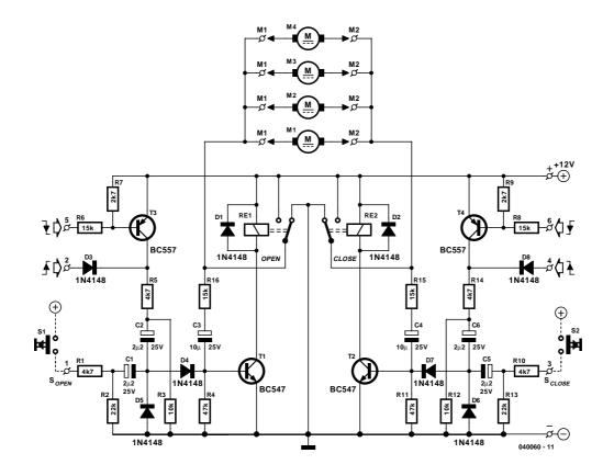
with positive or negative control. In order to make the unit universally applicable, both types of alarm can be used. The circuit around T3 and T4 makes this possible. The diode inputs (D3 and D8) react to a rising edge, R6 and R8 react to a falling edge. An RC time constant is used here as well to ensure that both relays are energised only once.
