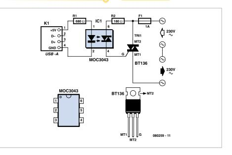
The circuit shown is used by the author for switching loads with a total power of about 150 W and is protected with a 1-A fuse. The circuit can easily handle much larger loads however. In that case and/or when using a very inductive load a so-called snubber network is required across the triac. The value of the fuse will also need to be changed as appropriate.
