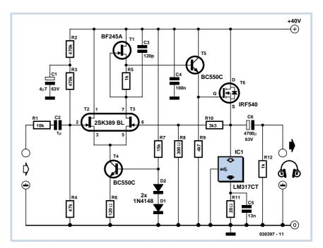
amplifier. The advantage is that excellent audio quality can be achieved even using a simple unregulated mains supply. Given the relatively low power output the power supply is considerably overspecified. Noise and hum thus remain more than 90 dB below the signal (less than 0.003 %), and the supply can also power two amplifiers for stereo operation.
