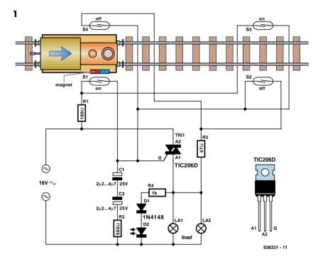
phase shifter, maintains the trigger current. The current through R2, C1 and the gate electrode (G) reaches its maximum value when the voltage across the load passes through zero. This causes the triac to be triggered anew for each half-cycle, even though no pulse is present at the gate. It remains triggered until S2 or S4 is closed, which causes it to return to the blocking state.
