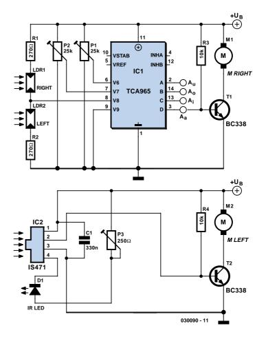
motor to stop, and the vehicle will rotate about the stationary wheel until the obstacle is no longer in its path. The sensitivity of the IS471 can be set using P3. As its range is only around 10–15 cm, the vehicle must not travel too quickly, since otherwise it will not be able to avoid obstacles in time.
