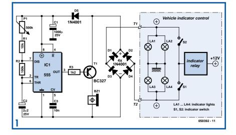
The timer always charges and discharges capacitor C2 to a level between a third and two-thirds of the operating voltage, producing an interval of
