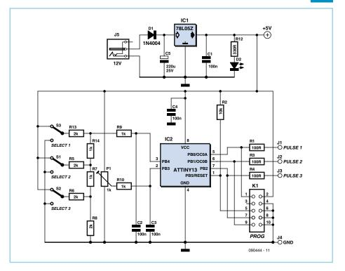
Fuses: CKSEL =  $0,1 \rightarrow 4.8$  MHz CKDIV8 =  $0 \rightarrow$  no divide by 8 SUT =  $1,0 \rightarrow$  slow rising power The source code and a hex file can be down-
