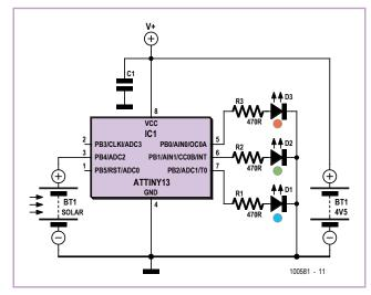
automatically switches on when it gets dark and off when it is light. The light sensor is made from one of the solar cells from a broken solar lamp (it is more common for the battery to fail rather than the solar cells).
