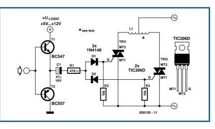
gised. This circuit takes advantage of the fact that triacs can be triggered by negative as well as positive gate currents. If the turnout coils are energised for too long, you should reduce the value of C1. If they are not energised long enough, increase the value of C1.
