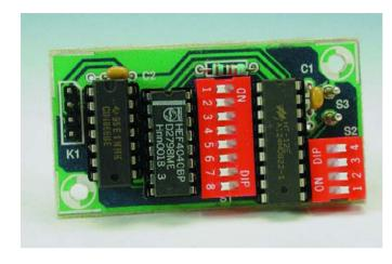
This application can actually be considered to be a slight adaptation of the standard use of the Holtek HT12E encoder (www.holtek.com). We have used this IC several times already, so it does not need any further explanation. The small circuit described here is intended to be used as an extension to the 'Mains Remote Transmitter', but it also clearly illustrates how the IC can be used in a non-standard manner.
