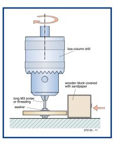
be fitted in the hole. Now secure the screw using a washer and nut, and then clamp it in the chuck of a drill press. Using a small block of wood wrapped in sandpaper, you can quickly sand the disc into a nice circular shape.
