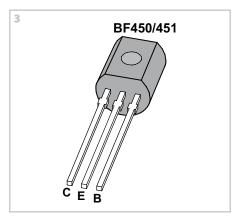
lings is replaced by a modern silicon p-n-p RF transistor like the BF450 or BF451 (**Figure 3**), resistors may have to be changed to get 0.6-0.7 V V<sub>B-E</sub> bias levels in the circuit. Also, almost all silicon transistors will
