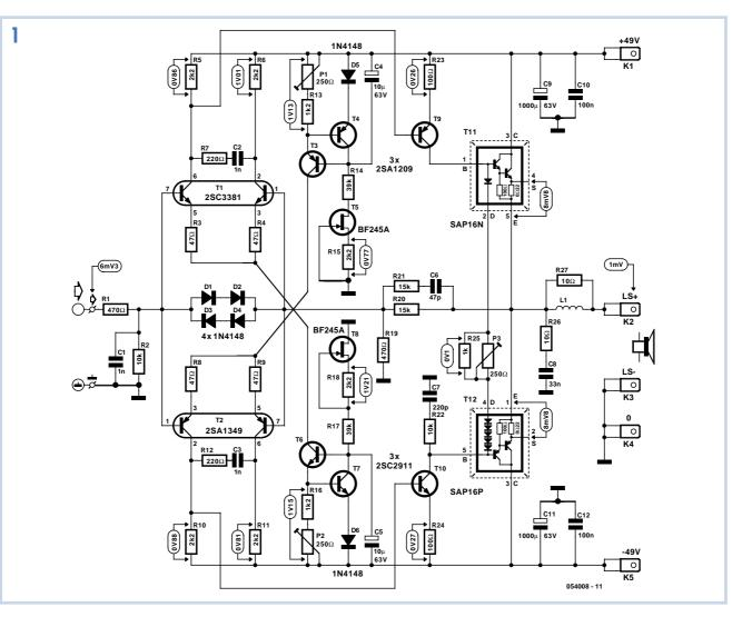
quiescent current, according to the datasheet. This causes an increase in distortion and a reduction in bandwidth. The current through the diodes has to be set to 2.5 mA, when the quiescent current will be 40 mA. This has the advantage that the driver transistors (T9, T10) do not need heat sinks, which helps to keep the circuit small.
