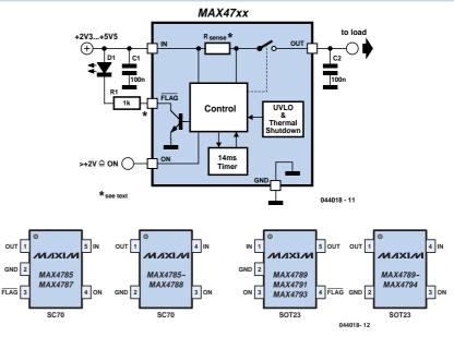
the current. During this 40-ms 'blanking time', the IC checks whether the current is less than the selected limit level. The latching types have the same time delay before
