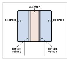
electrons pass from one material to the other. The two contact voltage sources are connected back to back in series which should cancel out the contact potential. So much for theory, in practice the boundary structure is not entirely homogeneous so that tiny potential differences are present. This produces the small potential difference that we can measure at the terminals.
