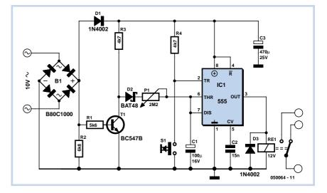
enced to earth potential and the pulsing full wave rectified signal is fed to the base of T1 via resistor R1. A 100-Hz square wave signal is produced on the collector of T1 as the transistor switches. The positive half of this waveform
