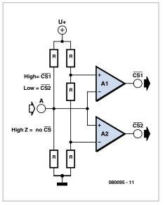
bly types with rail-to-rail outputs). Suitable examples to use are the LM393 or LM311. The resistances in the voltage dividers in this circuit are uniformly 10 kilohms.
