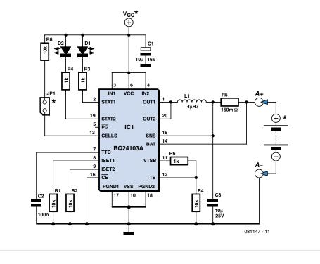
important is to note that jumper JP1 should be fitted **only in the case where two cells are being charged**. When charging a single cell the jumper must **not** be fitted, or there is a risk of **explosion** or **fire** as the charging voltage will be too high. The minimum supply voltage for charging a single cell is 5 V; for charging two cells it is 9 V. According to its datasheet, the IC is specified for supply voltages of up to 16 V.
