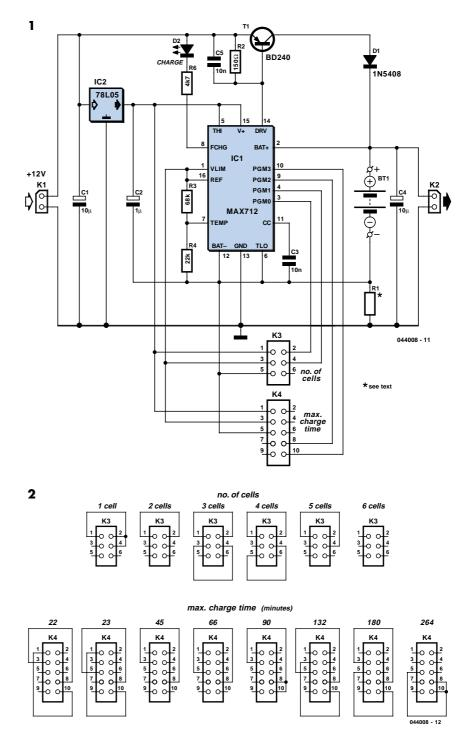
value of R1 the charging current can be set. The value of R1 can be calculated using the formula below:
