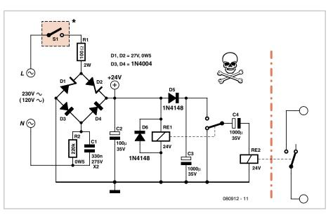
S1 opens when the relay in the wireless switch module is de-energized, which causes RE1 to drop out shortly afterward and connect capacitor C4 to ground. The capacitor discharges through the coil of RE2, causing its 'momentary' contact to be actuated again. The timing diagram shows the switch-on and switch-off sequences of the wireless switch (S1 contact).
