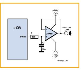
and 10 nF) gives a –3 dB corner frequency of around 4 kHz. When driven by a PWM frequency of approximately 20 kHz the filter will be suitable for outputting audio tones and voice signals with a bandwidth of 4 kHz. This simple filter will attenuate the 20 kHz fundamental PWM frequency by 14 dB which may not sound like much but the human ear has its own high frequency roll-off (the characteristics of which change as we age) so frequencies this high will be barely audible.
