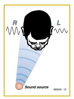
Figure 1. The head acts as a low-pass filter attenuating frequencies above 1 kHz. The ear nearest the sound source will hear the sound louder than the far ear. Despite its impressive functionality, GAS-TON cannot work with a continuous audio signal let alone follow a moving sound source. This ability requires a more complex approach which we will go on to investigate here.
