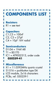
A preprogrammed controller can also be ordered from the site shop as item 050259-41. The CodeVision AVR compiler was used for software development. A demo version is available on the Internet but this version contains a restriction of 500 bytes on the maximum code size. A 'modification' in the code gets round this by specifying the larger 8515 controller and then resetting the stack pointer to the correct value for the 2313, the overall effect is to increase the code space to 2 kBytes.
