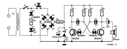
bell transformer. For this purpose, the ac voltage must be rectified by D3-D6, and Zener diode D7 prevents the voltage from rising above approximately 18 V. EMD immunity is provided by the lowpass network R5/C1. The bell can also be silenced using switch S2. In this case, the only thing that happens when someone presses on the bell button is that D1 lights up.
