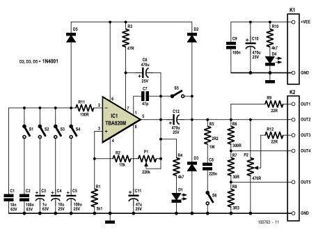
OUT1 is the main output protected with stopper resistor R9. It is used to test unknown circuits where large capacitance or inductances could be present, or circuits presenting a few volts themselves. R9 may be dimensioned to suit the application and can take a value between 22 to 100 ohms at a dissipation of 0.5 to 2 watts.
