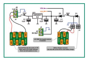
Figure 8. The simple but all-important power supply.
