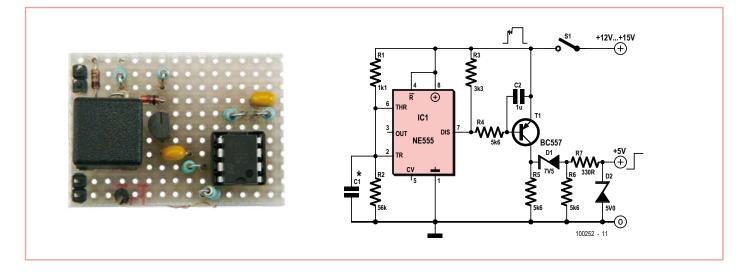
turn to a device such as the 555 timer IC to clean up the signal.
