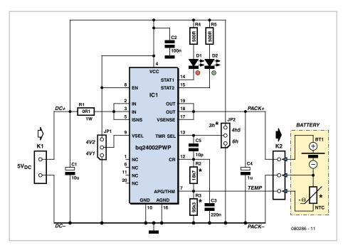
(the supply voltage) the time limit is four and a half hours, and if pin 13 is pulled to ground the time limit is six hours. If the final voltage is reached early, charging will of course cease before expiry of the time limit. The LEDs allow the charge process to be monitored. Red LED D1 lights during charging and flashes to indicate that a fault has been detected. When the cell is more than 90 % charged the red LED is extinguished and the green LED lights.
