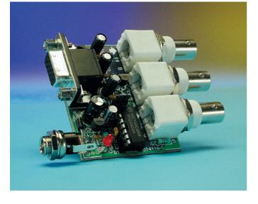
There are monitors which only have three BNC inputs and which use composite synchronisation ('sync on green'). This circuit has been designed with these types of monitor
