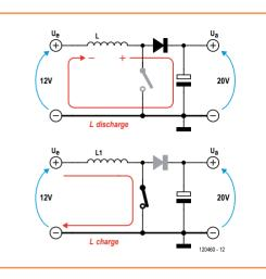
Figure 1. The two phases of the stepup conversion process.
