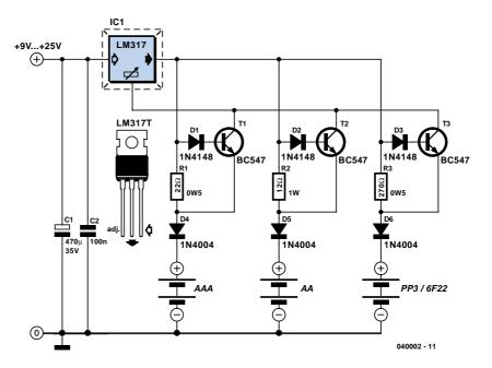
The current should be one tenth of the nominal battery capacity — for example, 170 mA for a 1700-mAh NiCd AA cell. It should be noted that 'PP3' rechargeable batteries usually contain seven NiCd cells so their nominal voltage is 8.4 V and not 9 V as is often thought.
