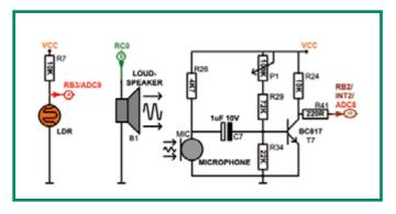
Figure 5. The microphone, loudspeaker and light sensor circuitry.
