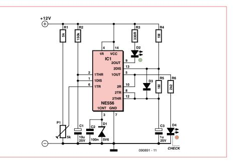
itor a 12-V supply voltage (such as voltage of the electrical system in a car) and signals an undervoltage situation with a blinking green LED, which is more likely to be noticed. The small red LED also lights up in case of undervoltage to provide confirmation. ers. One of them detects the switching threshold, and the other provides the blinking function.
