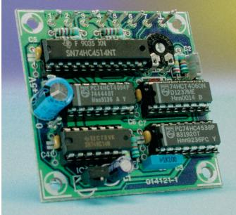
used is a 74HC4538, which is re-triggerable. By connecting the Q-output to the positive trigger input, IC5 is prevented from being triggered whilst it has an active output.
