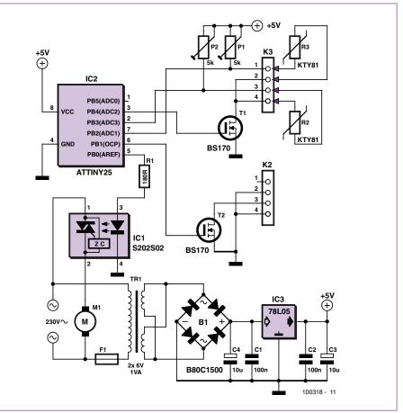
power pin (pin 5) is pulled high and the pump is started via the opto-triac. When the pump is started, another output (pin 6) is pulled low at the same time. You can connect external components to this output, such as an indicator lamp.
