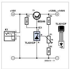
circuits (min. 10 seconds), with a voltage drop of typically no more than 1 V across the collector-emitter path of the transistor.
