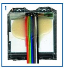
96x64 pixels). You can find numerous sites on the web which sell this product (new or used) as a one-off or in bulk. After such praise, what is there to criticise? Any difficulty in implementation is due to the connections. The connector is composed of gold-plated 'spring' blades (on the LCD) which rest on solder pads
