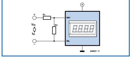
Voltmeter modules are readily available, both as LCD- and LED-versions. A disadvantage of these modules is the standard measuring range of 200 mV DC. So, with such a module you can only measure DC voltages up to 0.2 volts. Fortunately it is not difficult to increase the measuring range to higher voltages. In addition, it is also possible to measure current with these modules.
