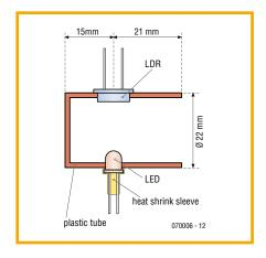
as light from it must pass through the finger and illuminate the LDR. Now, when the heart pumps a pulse of blood through the blood vessels, the finger becomes slightly more opaque and so less light reaches the LDR. This can be converted into an electrical pulse.
