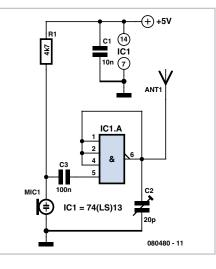
performance and sensitivity of the circuit. C1 serves to decouple the supply voltage so any spikes that may be present are suppressed. Just about any short length of wire makes a suitable antenna.
