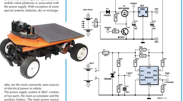
batteries, is for the power supply of the microcontroller only.
