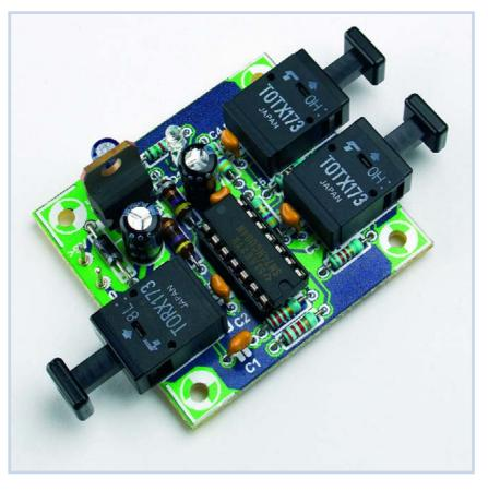
For the power supply a standard 7805 was selected with D2 as reverse polarity protection. L2 decouples the power supply voltage of IC4 some more. This does L1 for IC1 and R3 and R5 for IC2 and IC3 respectively. R4 and R6 are required
