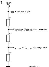
of +60 °C and VSETLOW = 1.641 V for a lower threshold of  $+55 \,^{\circ}\text{C}$  As VREF = 2.5 V. the values of R1, R2 and R3 can now be readily calculated from the current and the voltage drops across the resistors. The values calculated in this manner are shown in the schematic diagram, without taking into account whether such values are actually available. As the temperature thresholds used here are relatively close together, the
