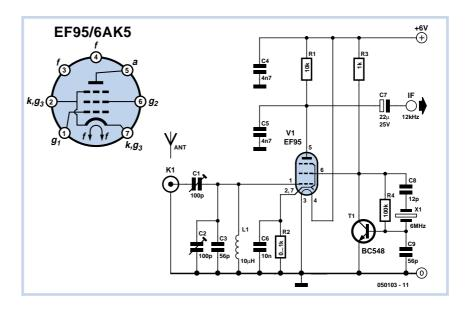
input impedance can be increased by increasing the value of the cathode resistor. However, good results can also be achieved with the cathode connected directly to ground.
