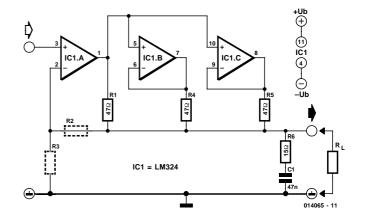
In the adjacent application note, IC1a is the boss and is supported by IC1b and IC1c or as many stages as you require. IC1a delivers, via R1, current to the load  $R_L$ . The 'helper-opamps' are connected to the voltage drop across R1. This way they will all deliver an identical current, because the resistors R4 and R5 have all the same values. Make sure that the whole thing does not oscillate — the addition of an RC-network R5-C1 across the load can work wonders.
