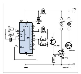
14-stage binary counter and some minimal output selection logic. Cycle time is determined by the way the internal oscillator is configured (resistor and capacitor on pins 9/10) and can be varied within quite broad limits. High-efficiency LEDs are your first choice for the indicators connected to the Beacon and Strobe outputs (remember to fit series resistors appropriate to the operating voltage Ub and the current specified for the LED used).
