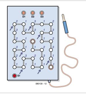
wishes to move) if the probe is touching one of the sockets. All 30 sockets are classified into three types, represented in the schematic diagram by one socket for each type. All sockets belonging to a particular type are simply connected together electrically, which is not shown on the schematic diagram for the sake of clarity.
