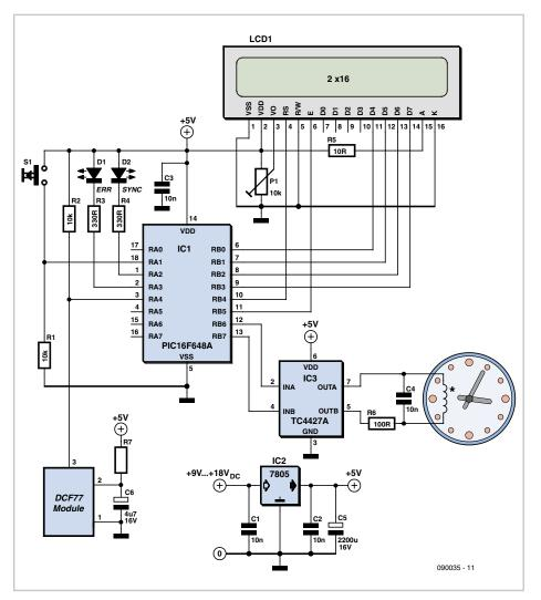
the hardware. The circuit is built around a PIC16F648A clocked by its internal 4-MHz oscillator. A standard two-row LCD (HD44780 compatible) is connected to the microcontroller to display operating instructions or the date and time.
