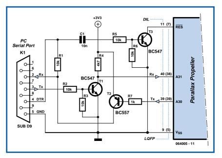
processors, the Propeller has a simple serial programming interface. The developer's toolkit from Parallax has a modern USB port for that purpose, but a reasonably simple alternative (illustrated here) is also possible for anyone who prefers to work with the familiar RS232 port. Don't forget that the Propeller works with a 3.3-V supply voltage.
