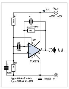
middle setting will suit us fine. Pin 8 is therefore connected to the voltage divider R1/R2. The current consumption of the entire circuit is impressively modest and at 5 V this is just 56 µA! The oscillator also functions astoundingly well at 3.3 V. At the same time the current drops to a more battery-friendly 41 µA. A prototype built in the Elektor Labs produced the slightly higher values indicated in the circuit diagram.
