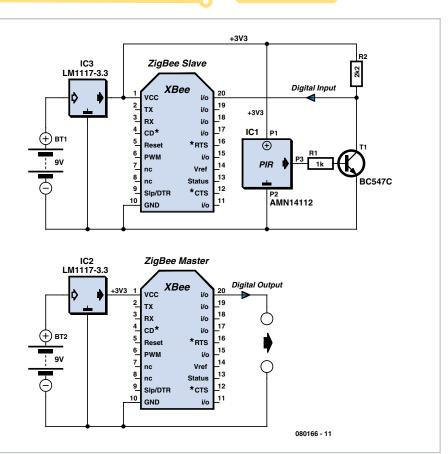
off and the 3.3-V supply voltage is applied to the ZigBee module via a 2.2-k $\Omega$  pull-up resistor. Power is provided by the 9-V battery. This compact circuit can be built into
