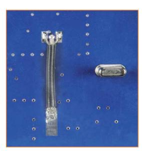
is as follows. First clamp the bare board in the sheet-metal box and fit all necessary chassis components. An SMA chassis-mount connector is recommended for the antenna connection. If you use a bulkhead connector, it can easily be soldered to the sheet metal. This also eliminates the need for screws. The connectors for the supply voltage and the audio input can be fitted in any desired location. A Cinch (RCA) chassismount connector is a good choice for the audio connection.
