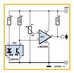
as a failsafe precaution against the robot dropping off a table edge.
