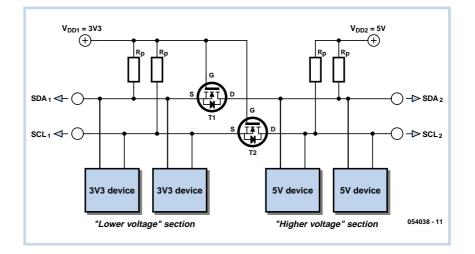
of the lower voltage section, and the drains (d) to the same of the higher voltage section. The MOSFETs should have their source connected to the substrate when in doubt check the datasheet. Other supply voltages than 3.3 V and 5 V may be applied, for example, 2 V and 10 V is perfectly feasible. In normal operation VDD2 must be higher than or equal to VDD1.
