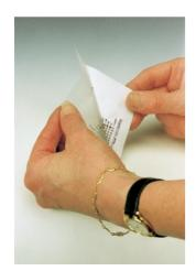
1. The decal is designed at true size (1:1 or 100%) with a graphics program or a word processor, and then printed in black and white on a sheet of white paper (do not use the colour ink cartridge). Allow the ink to dry. Cut the foil as required, then pull the adhesive sheet from the paper carrier sheet. Keep the carrier paper handy, it will be used in the next phase.
