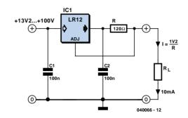
The output voltage is defined by a potential divider chain connected between the output and the ADJ (adjust) input pin. The regulator simply changes its output voltage until the divided voltage at the ADJ input is equal to 1.2 V. The output voltage can be more precisely expressed as a function of R1 and R2 in the formula:
