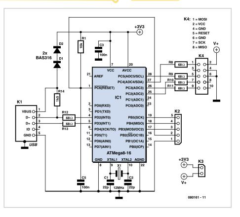
AVR Studio, the standard Atmel development environment, as if it were a 'real' AVR-ISP programmer. The circuit is easily built on a small piece of prototyping board or even on a breadboard, since the controller is available in a DIP-28 package. If you are going to program the controller yourself (via connector K2) then make sure that you set the configuration fuses so that the internal oscillator uses the external crystal as the
