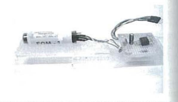
Figure 7-20 Magnetometer sensor and regulator assembly
