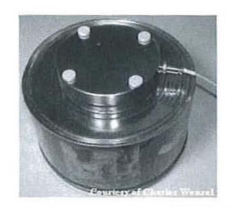
Figure 10-12 Ion chamber housed in a metal can
