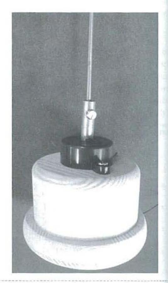
Figure 6-6 Mounted piezo sensor housing
