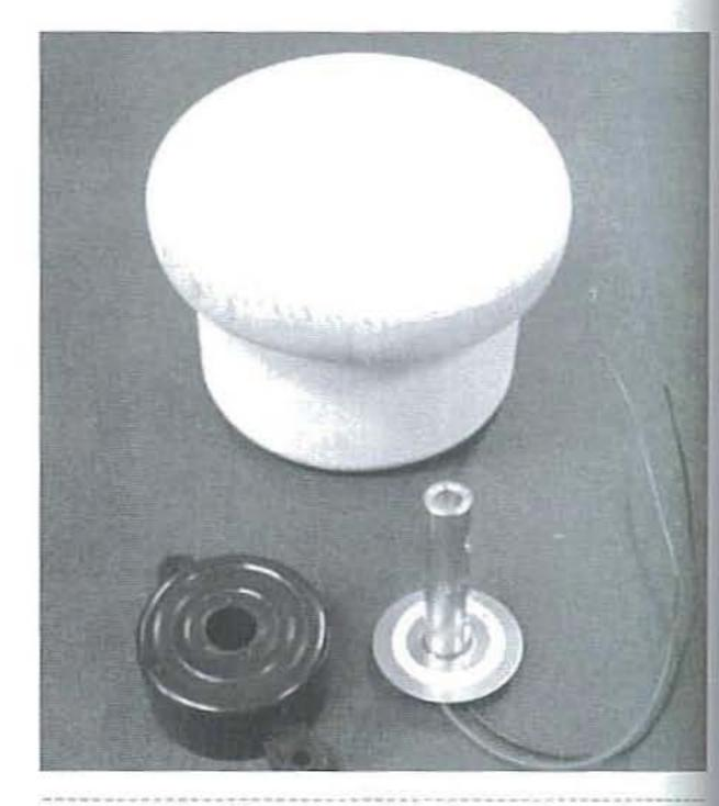
Figure 6-5 Piezo sensor and mounting components
