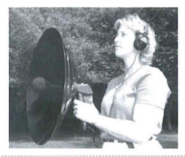
Figure 1-2 Parabolic microphone
