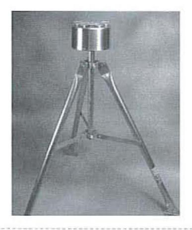
Figure 8-17 Cloud charge monitor mounted on a short tripod
