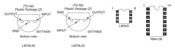
Figure 19-3 Semiconductor pin-outs
