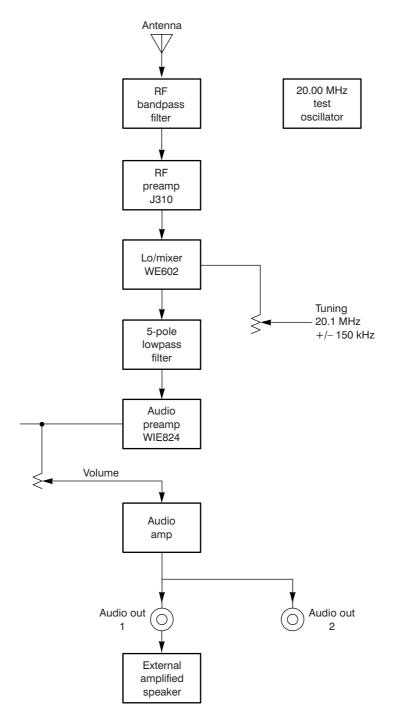
Figure 22-3 Jupiter radio block diagram
