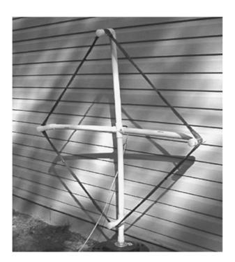
Figure 19-5 Loop antenna
