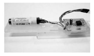
Figure 18-2 FGM-3 Magnetometer sensor
