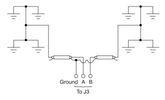
Figure 21-6 ULF receiver antenna circuit
