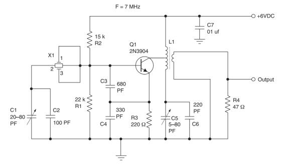
Figure 2-8 Ceramic resonator VFO circuit
