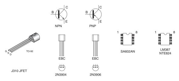
Figure 22-5 Semiconductor pin-outs
