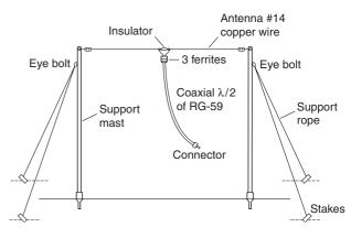
Figure 22-6 Basic dipole antenna diagram. Courtesy Wes Greenman, Charles Higgins
