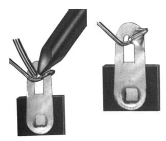
Figure 3-7 Wire to lug soldering joint
