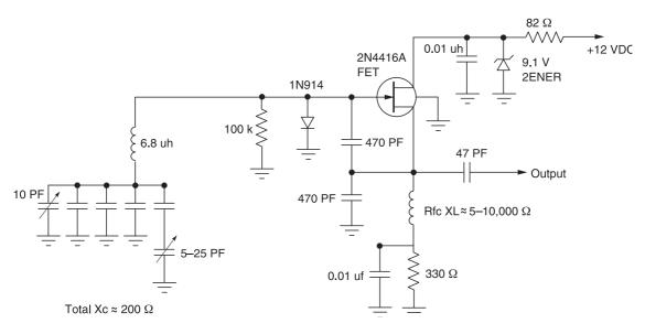
Figure 2-5 Series tuned Colpitts oscillator circuit
