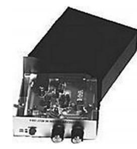
Figure 9-1 80/40 meter code receiver
