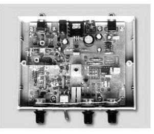
Figure 23-2 Weather satellite receiver
