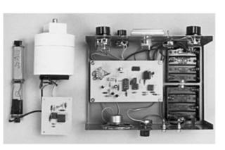
Figure 20-2 Aurora monitor console and sensor
