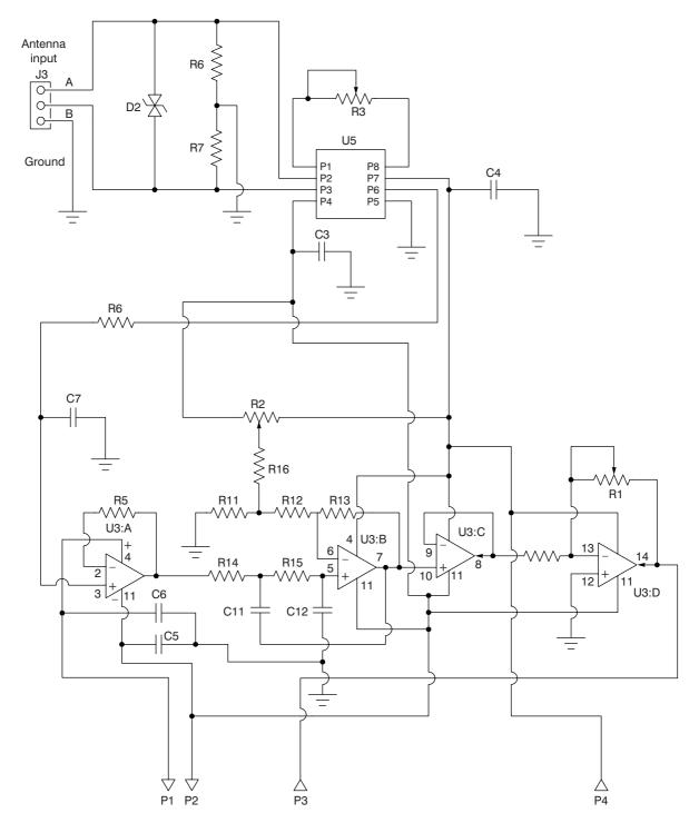
Figure 21-2 ULF receiver schematic – Part I
