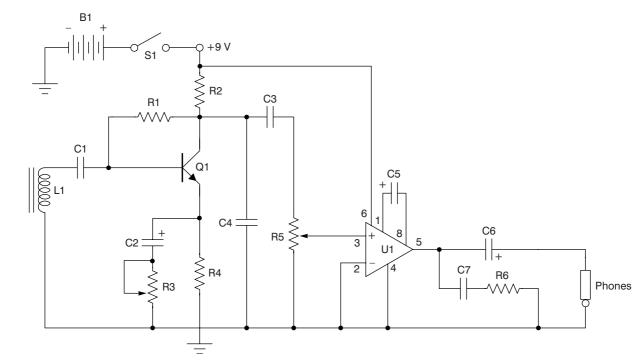
Figure 15-5 Induction loop receiver schematic
