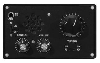
Figure 12-1 6N2 meter amateur radio receiver
