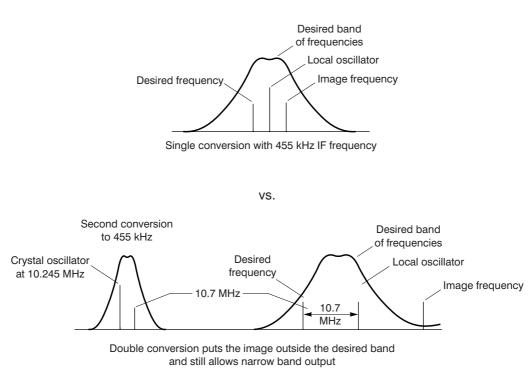
Figure 12-3 Single vs. double conversion receiver
