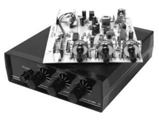
Figure 13-1 Active aircraft band receiver
