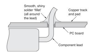
Figure 3-10 Excellent solder joint
