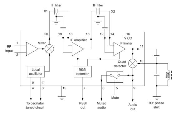
Figure 23-3 Weather satellite receiver block diagram
