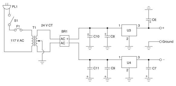
Figure 19-4 Dual voltage power supply
