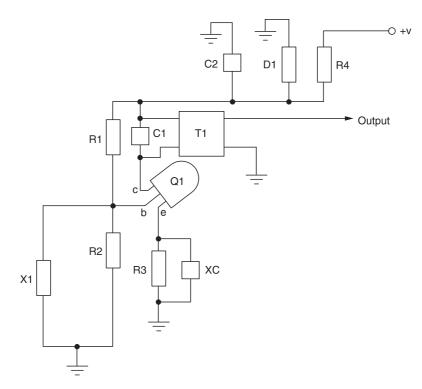
Figure 2-7 Crystal oscillator pictorial diagram
