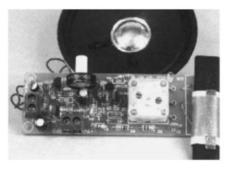
Figure 5-3 AM TRF receiver
