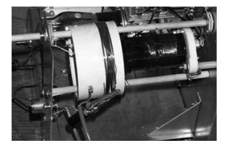
Figure 7-4 Doerle coil assembly
