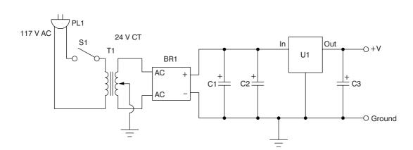
Figure 18-9 Magnetometer power supply
