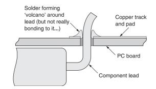
Figure 3-11 Inferior solder joint: Example 1
