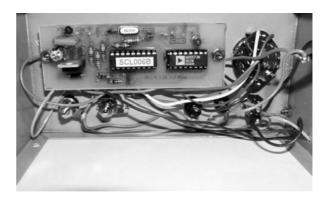
Figure 18-8 Magnetometer – inside view
