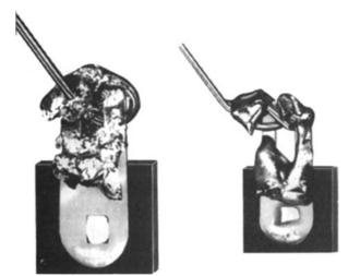
Figure 3-8 Inferior wire to lug solder joint
