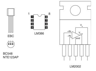
Figure 15-6 Semiconductor pin-outs
