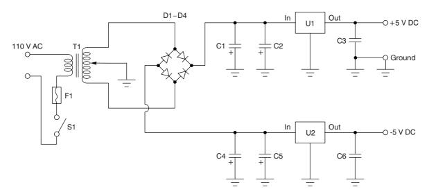
Figure 21-4 ULF receiver power supply
