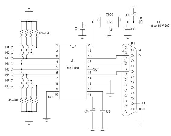
Figure 24-3 8 channel A/D converter – ADC 2. Courtesy of Radio-Sky Publishing
