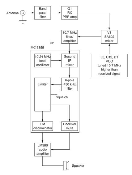
Figure 11-2 VHF monitor receiver block diagram
