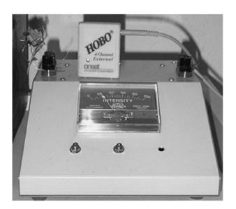
Figure 19-1 Sudden ionospheric disturbance receiver
