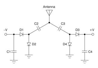
Figure 17-2 Ambient power module 1
