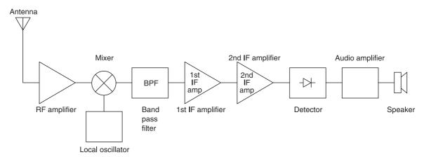
Figure 1-6 AM radio block diagram
