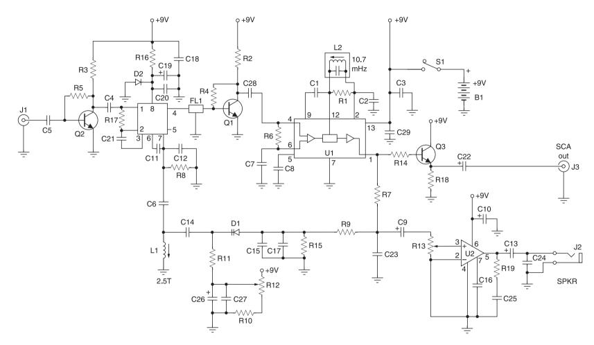
Figure 6-4 FM broadcast receiver. Courtesy of Ramsey Electronics
