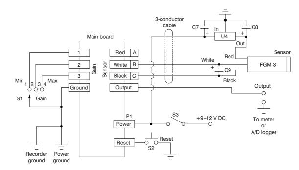
Figure 18-5 Magnetometer connection diagram
