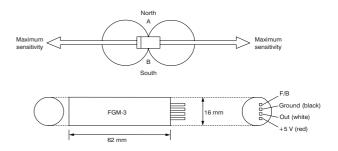
Figure 18-3 FGM-3 Magnetometer sensor
