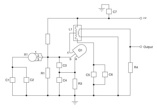
Figure 2-9 Ceramic resonator VFO pictorial circuit diagram
