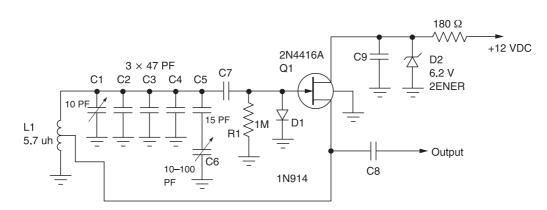
Figure 2-4 Hartley oscillator circuit
