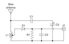
Figure 4-6 Simple FM crystal radio
