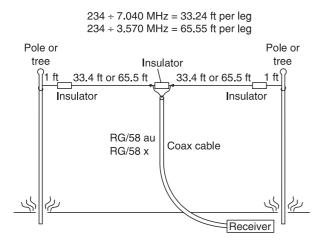
Figure 9-4 80/40 meter dipole antenna
