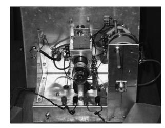
Figure 7-2 Doerle receiver – inside view
