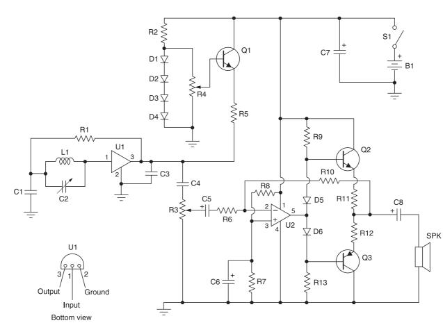
Figure 5-5 TRF AM receiver broadcast band receiver
