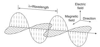
Figure 1-2 Magnetic vs. electric wave
