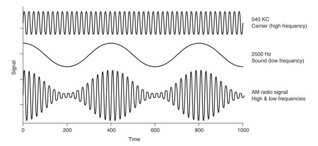
Figure 5-2 AM carrier and modulation signals
