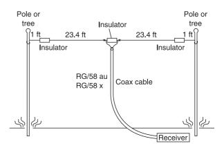
Figure 10-6 *MHz dipole antenna*
