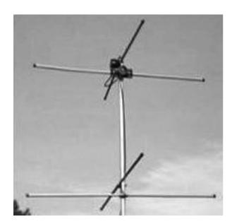
Figure 23-6 VHF turnstile antenna
