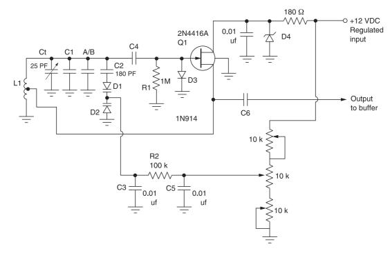
Figure 2-10 Voltage controlled oscillator (VCO) circuit
