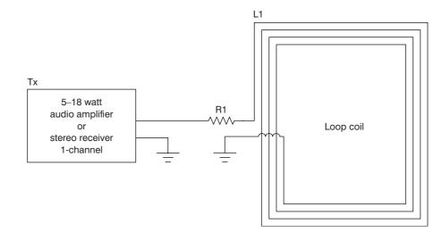
Figure 15-2 Induction loop transmitter I
