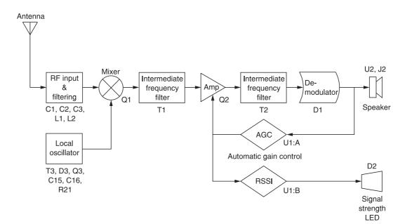
Figure 8-2 Shortwave receiver block diagram
