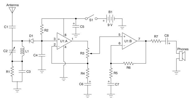
Figure 13-4 Passive aircraft receiver schematic
