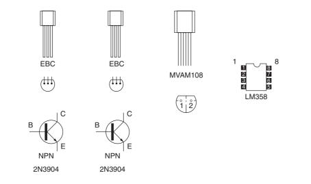
Figure 8-4 Semiconductor pin-outs
