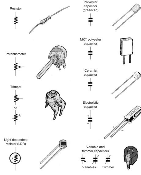
Figure 2-1 Electronic components 1
