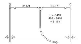
Figure 8-5 Shortwave dipole antenna
