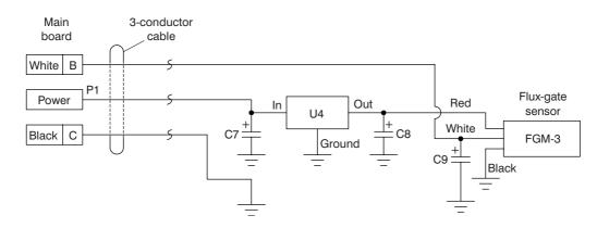
Figure 18-6 Flux-gate sensor board
