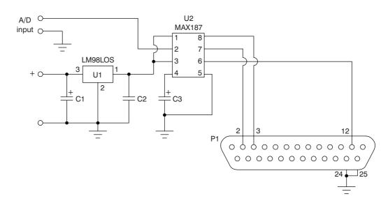
Figure 24-1 Single channel A/D converter – ADC 1. Courtesy of Radio-Sky Publishing
