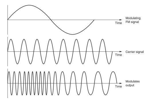
Figure 1-4 FM modulation waveform
