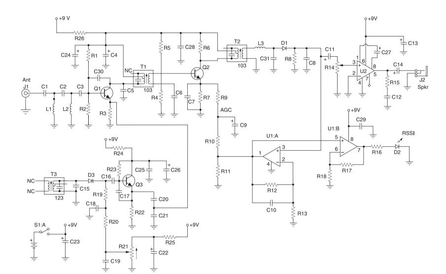
Figure 8-3 Shortwave receiver schematic. Courtesy of Ramsey Electronics
