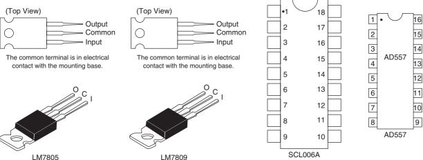
Figure 18-7 Semiconductor pin-outs
