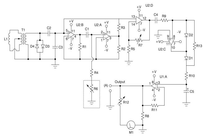
Figure 19-2 Sudden ionospheric disturbance receiver
