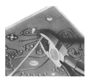
Figure 3-13 Trimming excess component leads
