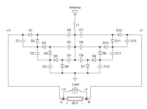
Figure 17-4 Ambient power module II
