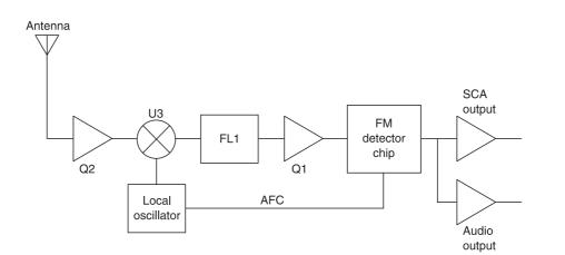
Figure 6-3 FM broadcast receiver block diagram
