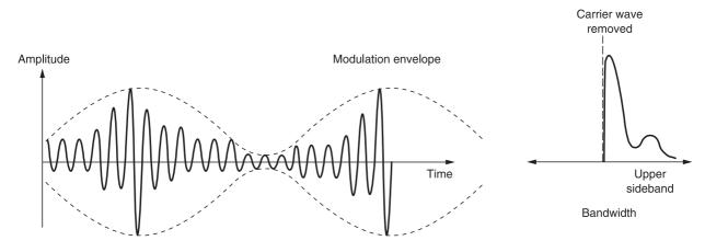
Figure 1-5 Single sideband modulation waveform
