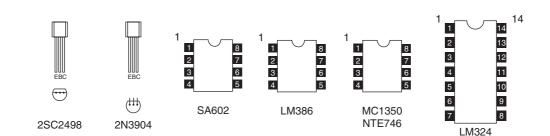
Figure 13-3 Semiconductor pin-outs
