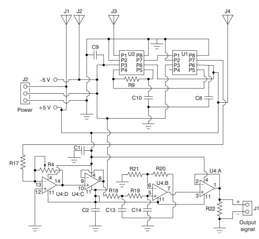
Figure 21-3 ULF receiver schematic – Part II
