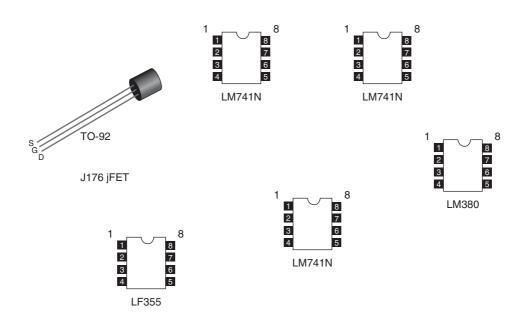
Figure 16-3 Semiconductor pin-outs
