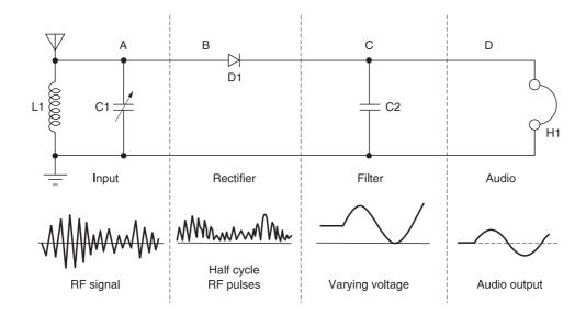
Figure 4-2 Basic crystal radio
