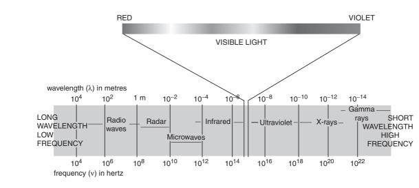
Figure 1-1 Electromagnetic spectrum
