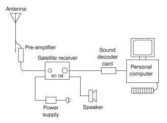
Figure 23-8 Weather satellite receiving system diagram
