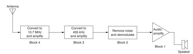
Figure 12-2 % meter amateur radio receiver block diagram
