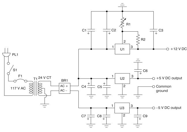
Figure 16-5 Multi-voltage power supply
