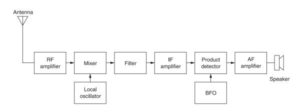
Figure 1-8 SSB shortwave receiver block diagram
