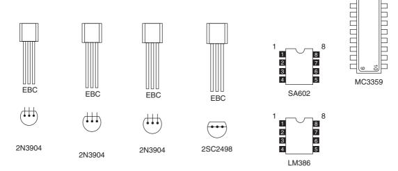
Figure 11-4 Semiconductor pin-outs
