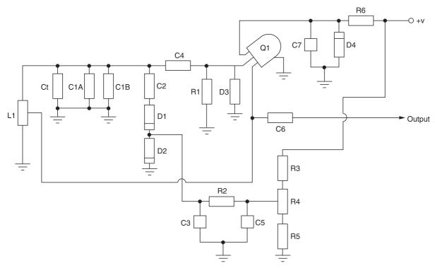
Figure 2-11 Voltage controlled oscillator (VCO) pictorial diagram
