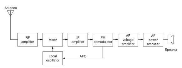
Figure 1-7 FM radio block diagram
