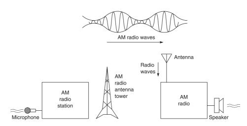
Figure 5-1 AM broadcast system block diagram
