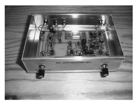
Figure 22-2 Radio Jupiter receiver project
