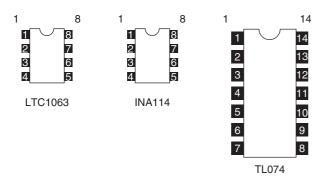
Figure 21-5 Semiconductor pin-outs
