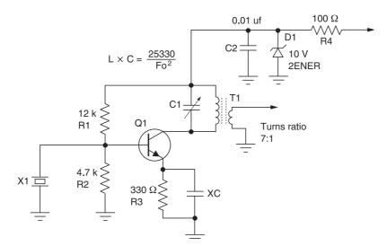
Figure 2-6 Crystal oscillator circuit
