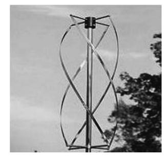
Figure 23-7 Quadrifillar antenna
