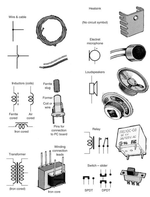
Figure 2-3 Electronic components 3
